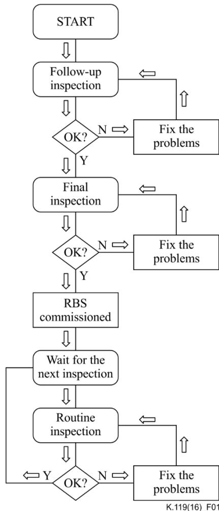
**Figure 1 – Flowchart of the conformance assessment process**
