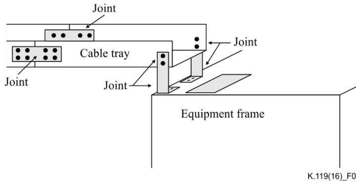
**Figure 4 – Details of the electrical continuity in trays and equipment frame**
