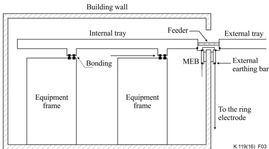
**Figure 3 – Lateral view of the RBS showing the bonding between the internal tray and equipment frame**
