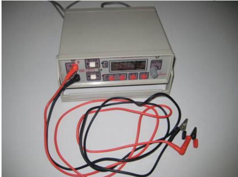
Figure I.1 – A typical example of apparatus for the test of the DC parameters of MOV SPDs
