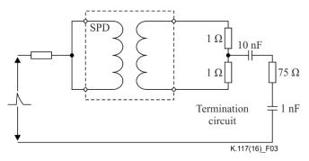
Figure 3 – Isolating transformer common-mode voltage blocking (partial circuit for only one twisted pair)
