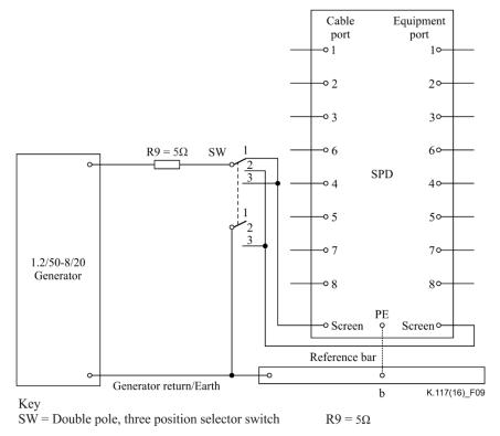
Figure 9 – Screen bonding test
