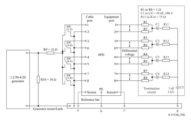
Figure 5 – Single twisted-pair differential-mode surge test circuit
