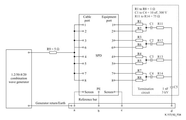
Figure 4 – Impulse limiting voltage under common-mode surge conditions
