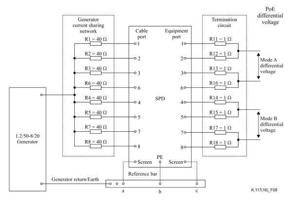
Figure 8 – Power feed pair common-mode to differential mode surge conversion test circuit
