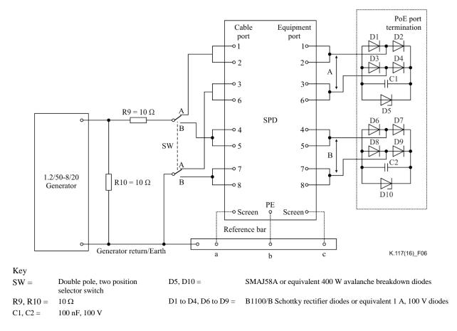
Figure 6 – Power feed differential mode surge test circuit
