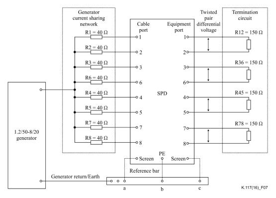
Figure 7 – Twisted-pair common-mode to differential mode voltage surge conversion test circuit
