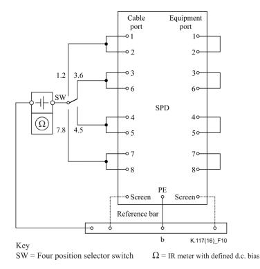
Figure 10 – Test circuit to measure the insulation resistance of an SPD with a PE terminal or screen terminals, or both
