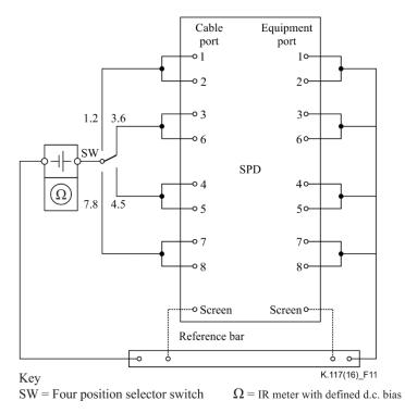
Figure 11 – Test circuit to measure the insulation resistance of an isolating transformer SPD without a PE terminal
