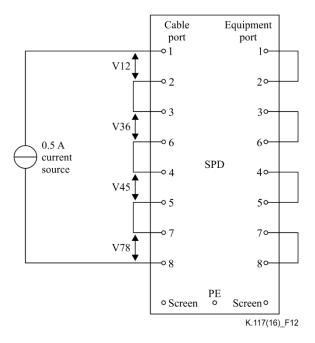
Figure 12 – Test circuit to measure the PoE SPD d.c. input/output voltage drop
