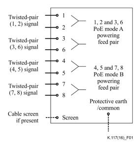
Figure 1 – Ethernet RJ45 contact connections
