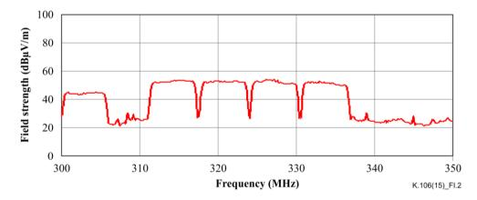
Figure I.2 – Radio spectrum of disturbance from coaxial cabling
