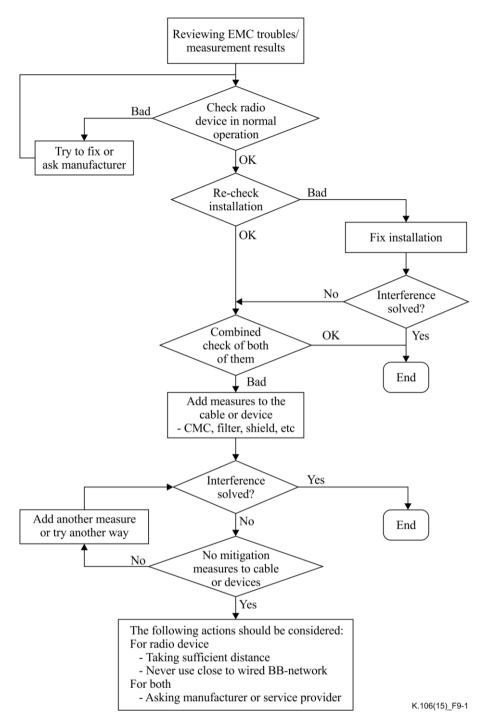
Figure 9-1 – Procedure to mitigate an interference problem
