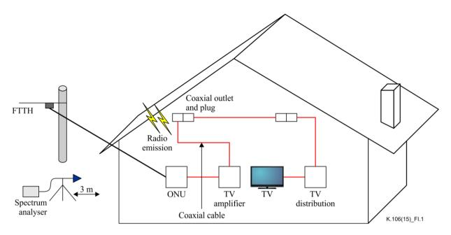
Figure I.1 – Configuration of telecommunication systems in which a radio disturbance occurred (disturbance caused by TV signal from ONU of FTTH)
