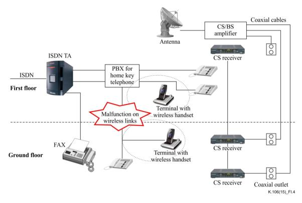
Figure I.4 – Configuration of a telecommunication system in which a radio disturbance occurred (disturbance caused by IF signal of CS/BS antenna)
