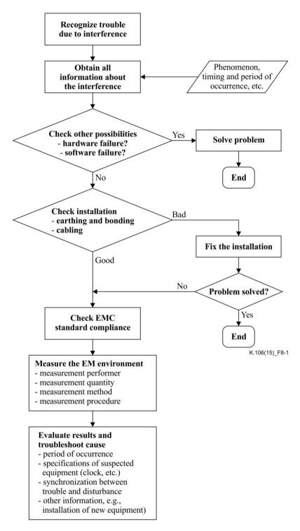
Figure 8-1 – Interference reduction and troubleshooting flowchart
