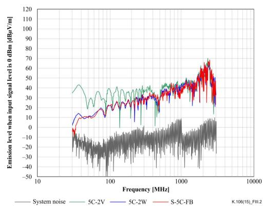
Figure III.2 – Frequency dependency of emission for different structures of coaxial cable (vertical polarization)
