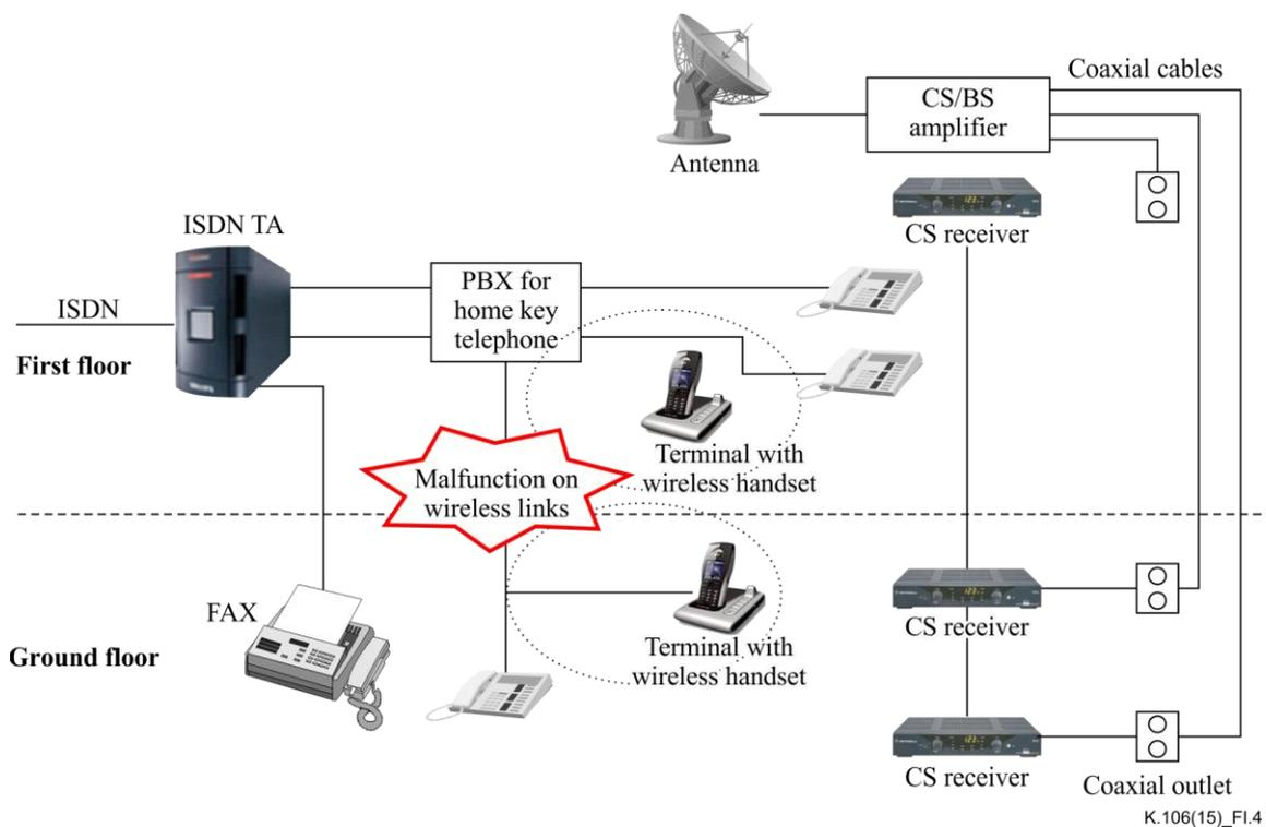
**Figure I.4 – Configuration of a telecommunication system in which a radio disturbance occurred (disturbance caused by IF signal of CS/BS antenna)**
