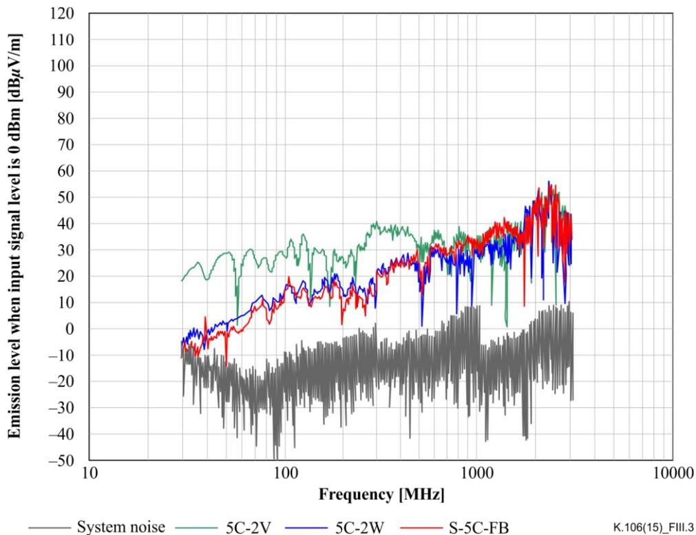
**Figure III.3 – Frequency dependency of emission for different structures of coaxial cable (horizontal polarization)**
