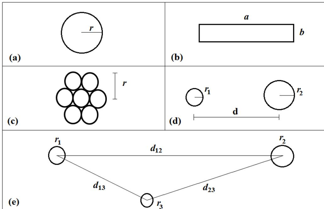
**Figure A.1 – Geometric mean radius of typical conductors**
