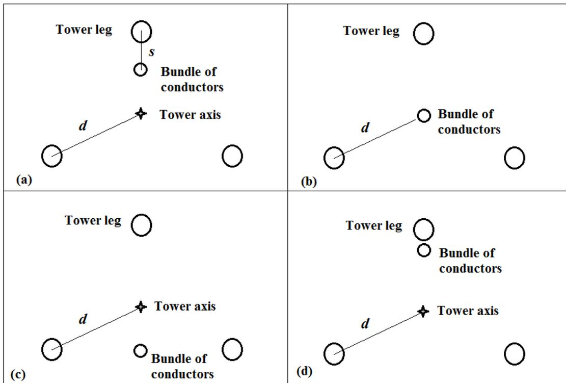
**Figure 4 – Distances for three-legged tower**
