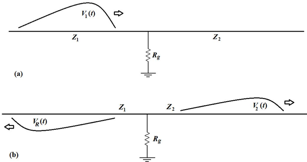
**Figure 7 – Incident voltage  $V_1(t)$  arriving at a line discontinuity (a) and the resulting reflected  $V_R(t)$  and refracted  $V_2(t)$  voltages (b)**
