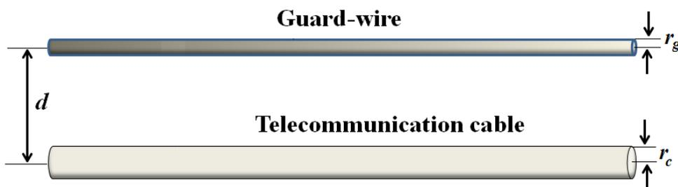
Figure 2 – Guard-wire above a telecommunication cable
