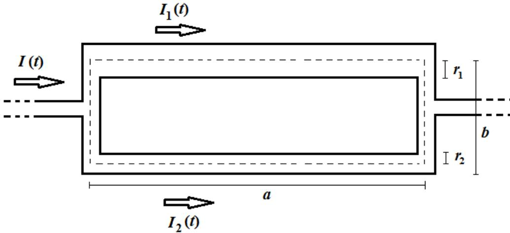
**Figure 1 – Representation of a transient current being split into two parallel conductors**
