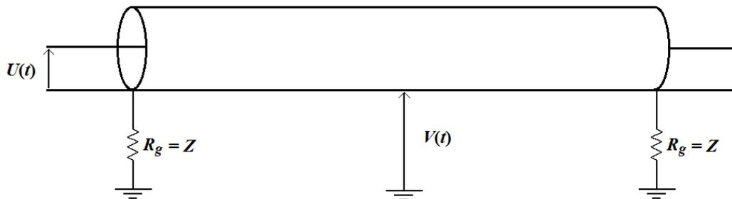
**Figure 8 – Equivalent circuit for shielded telecommunication cable**
