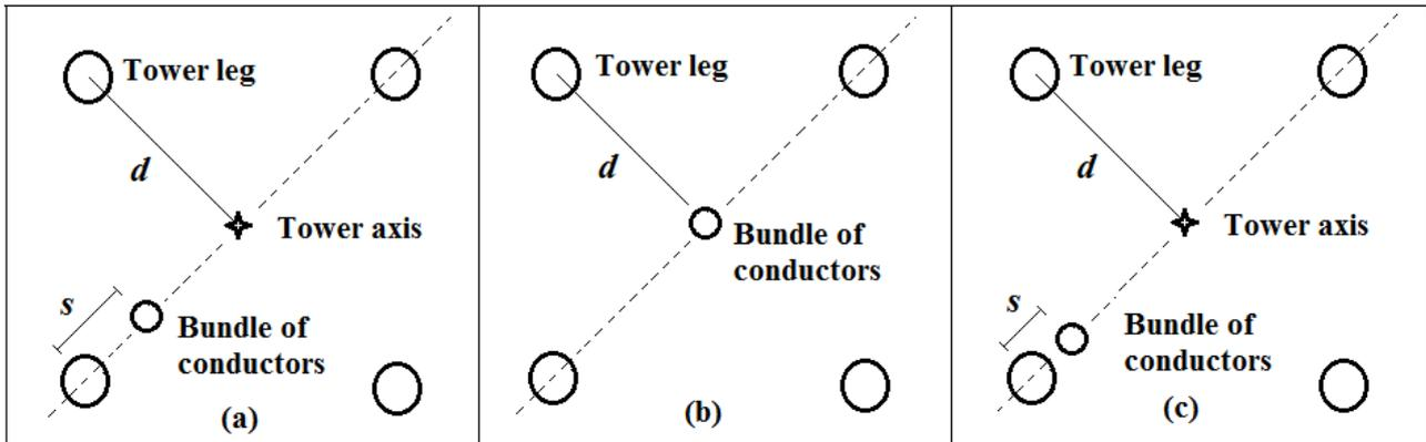
Figure 5 – Distances for four-legged tower
