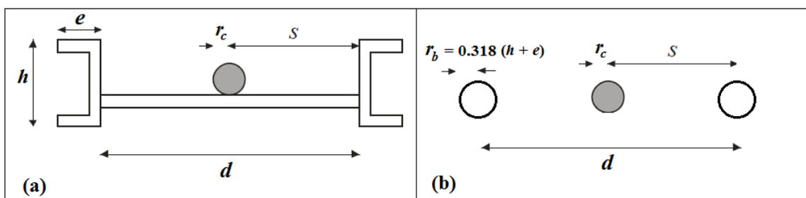
**Figure 6 – Representation of a ladder tray by cylindrical conductors**
