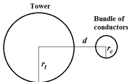
Figure 3 – Distances for tubular tower
