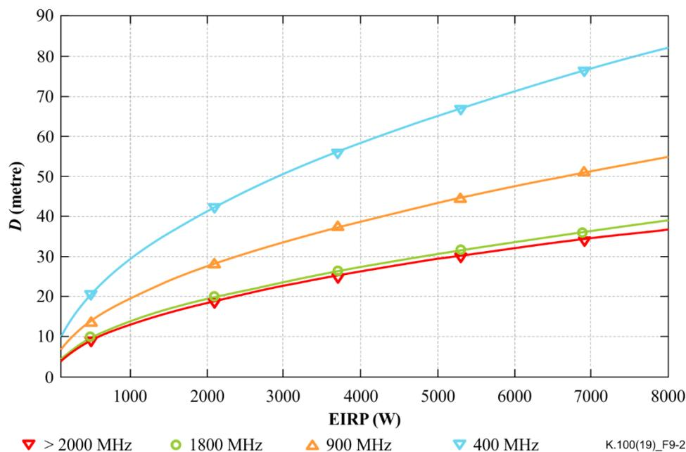
**Figure 9-2 – Side length of the assessment domain boundary as a function of the equivalent isotropically radiated power for some frequencies, estimated using equation 9-1<sup>13</sup>**
