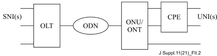
**Figure II.2 – Generic GPON system (from ITU-T G.983)**
