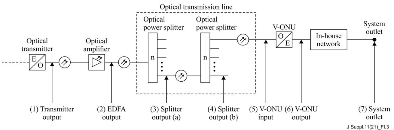
**Figure I.3 – Measurement points of video distribution system**
