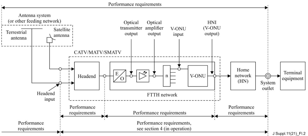
**Figure I.2 – Points of performance specification of the FTTH system**
