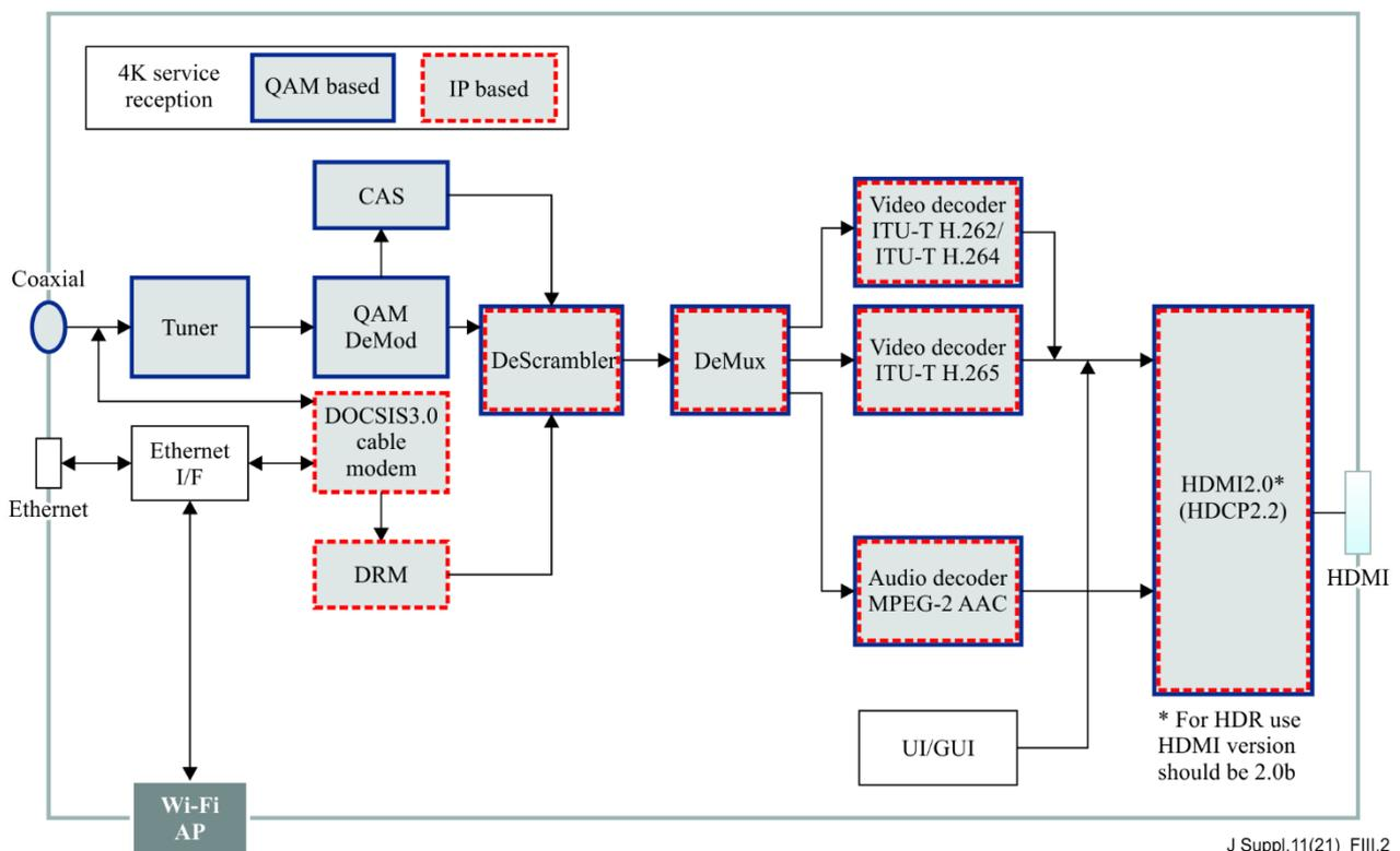
Figure III.2 – Example of 4K cable STB block diagram (from [b-ITU-T J.297])
