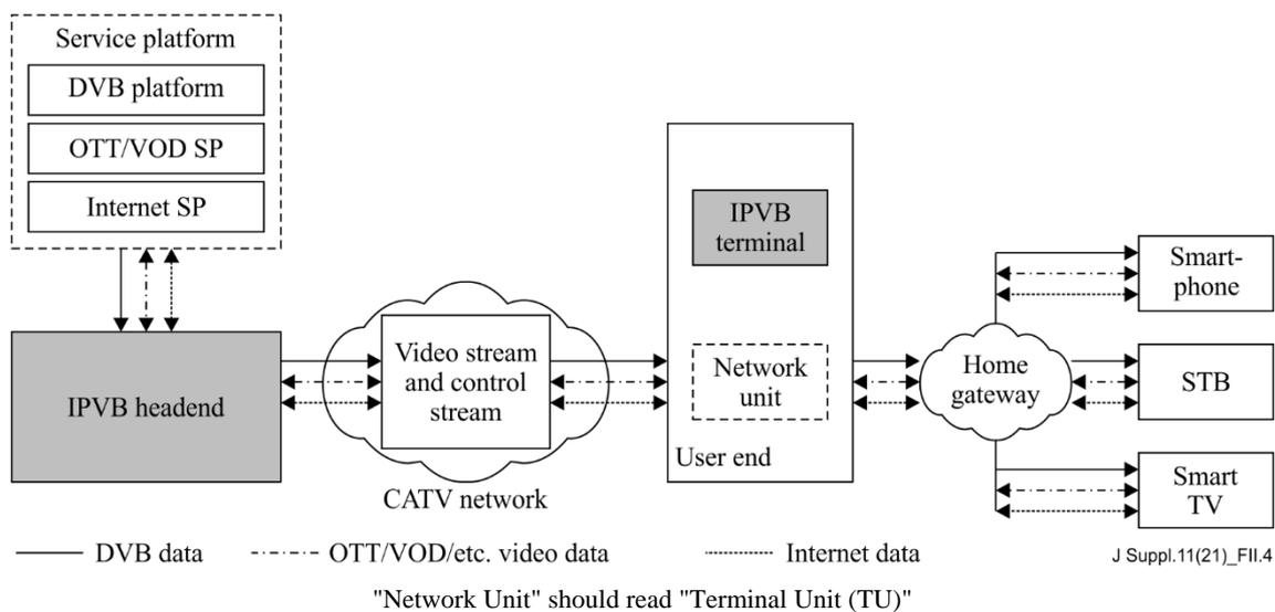
**Figure II.4 – IPVB architecture (from ITU-T J.1210)**
