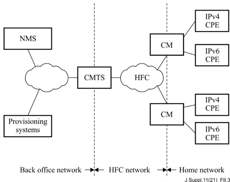
**Figure II.3 – DOCSIS network (from [b-ITU-T J.222.1])**
