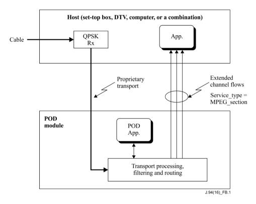
Figure B.1 – A framework for the extended channel service information stream
