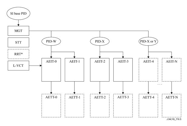
Figure III.5 – Hierarchy of Table Sections – Profile 6
