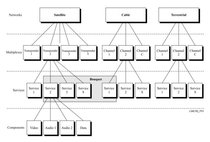
Figure 1 – Digital broadcasting, service delivery model
