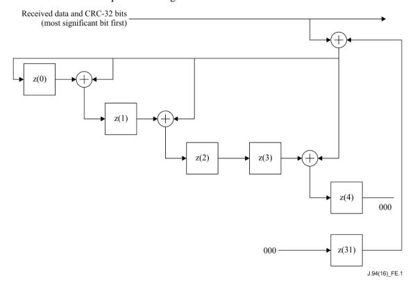
Figure E.1 – 32 bit CRC decoder model
