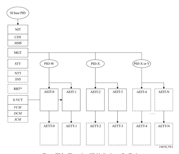
Figure III.3 – Hierarchy of Table Sections – Profile 4
