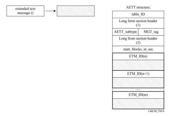
Figure III.9 – Structure of AETT
