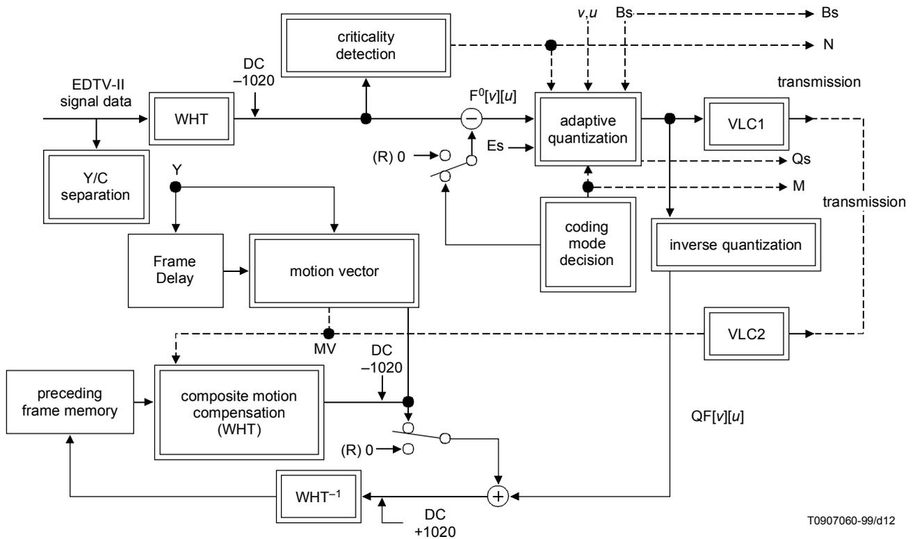
Figure A.2-1/J.88 – Whole structure of coding process
