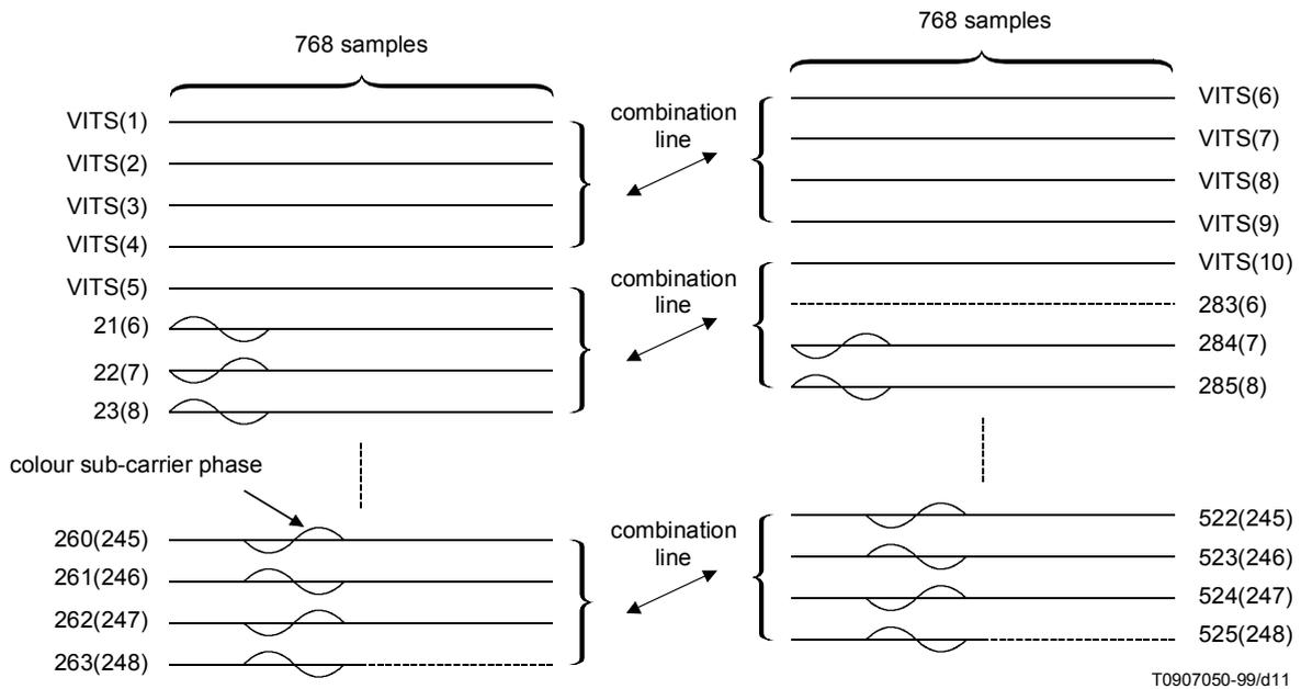
Figure A.1-9/J.88 – Frame-based WHT coding based on field merge
