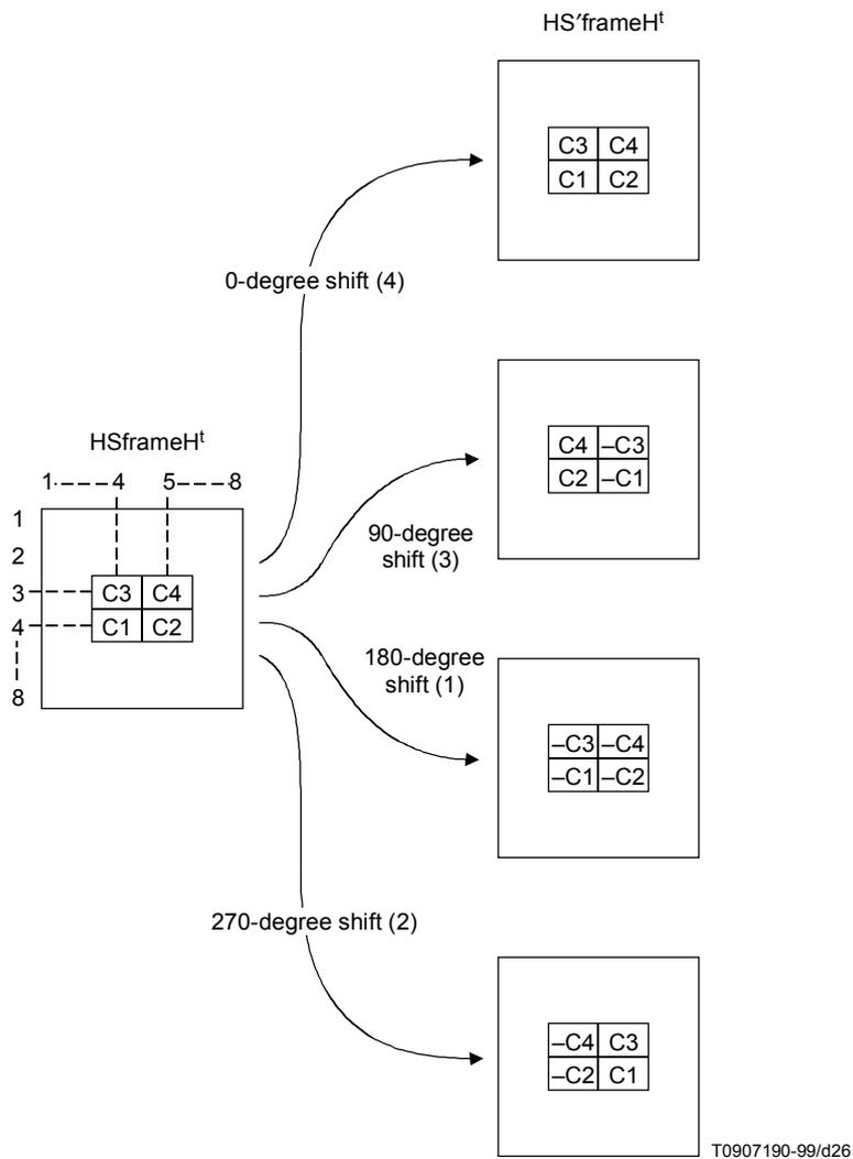
Figure A.2-13/J.88 – Colour sub-carrier on two-dimensional Hadamard transform
