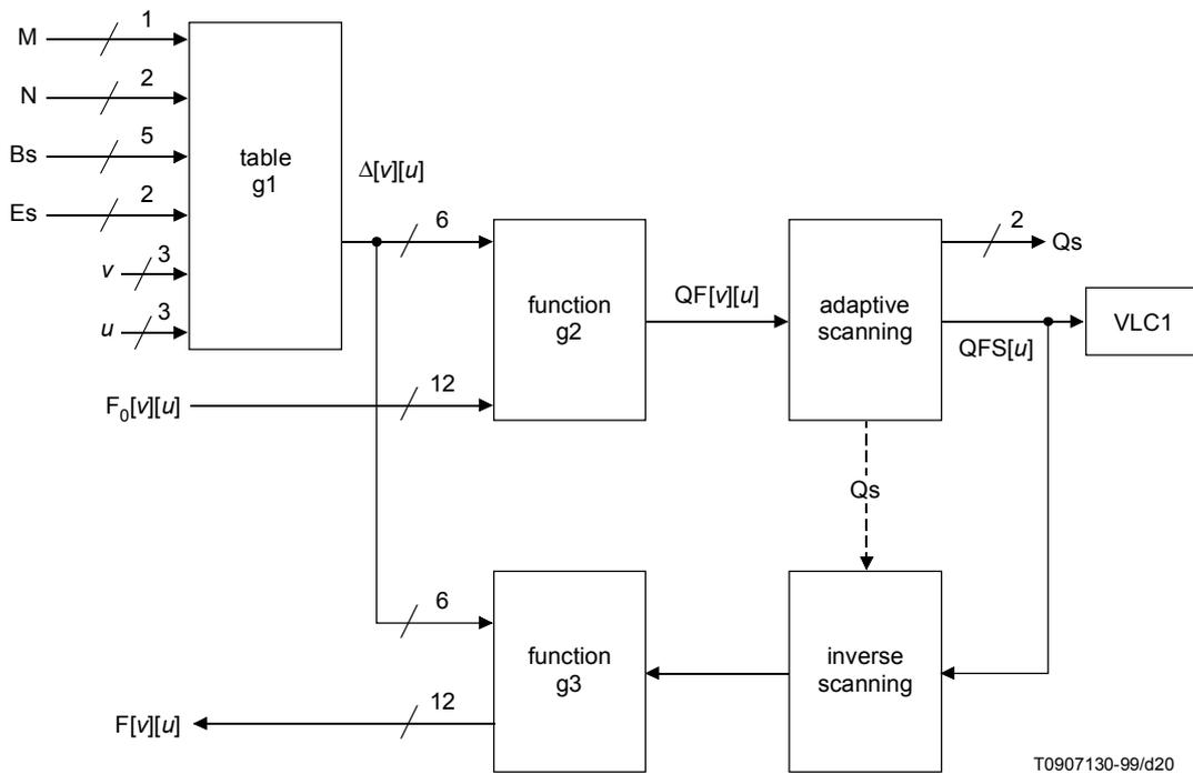
**Figure A.2-7/J.88 – Adaptive quantization/adaptive scanning**
