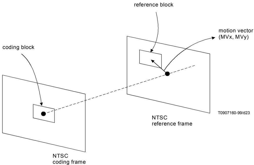
**Figure A.2-10/J.88 – Motion compensation interframe coding of NTSC**
