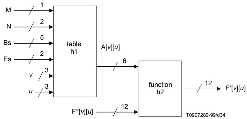
Figure A.3-3/J.88 – Structure of inverse mixed mode
