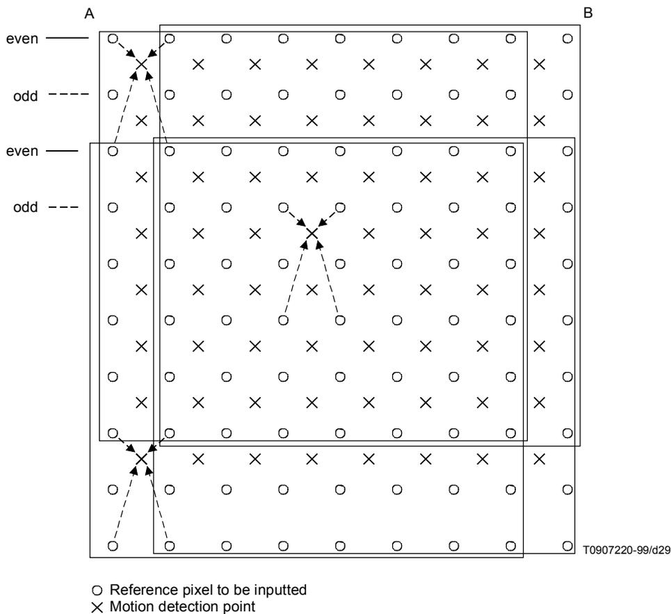
**Figure A.2-16/J.88 – Reference pixel to be inputted and motion detection point**
