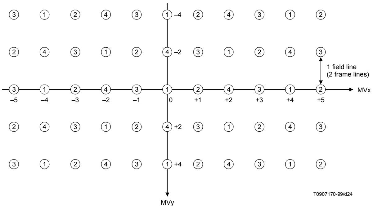
**Figure A.2-11/J.88 – Phase shift of colour sub-carrier depending on the motion vector ( $MV_x$ ,  $MV_y$ )**
