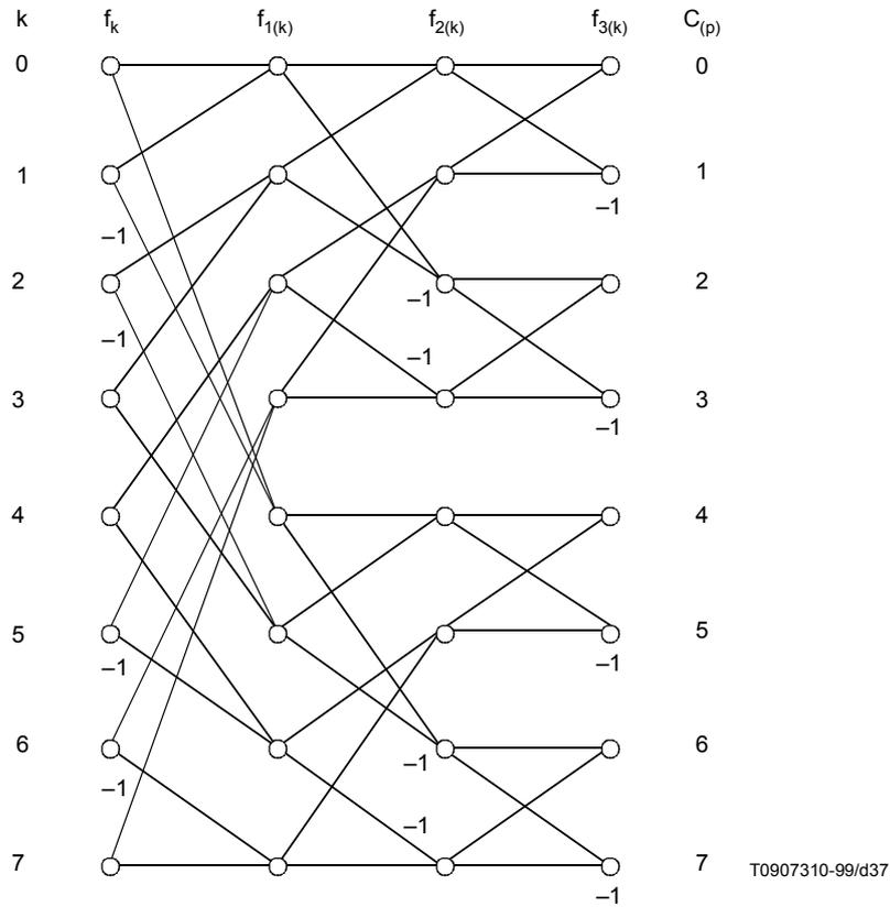
Figure IV.2/J.88 – Flow diagram  $\alpha$  of  $H(8)$
