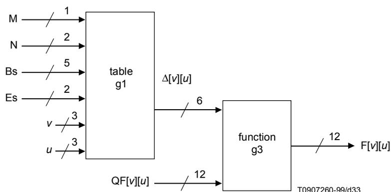
Figure A.3-2/J.88 – Structure of inverse quantization
