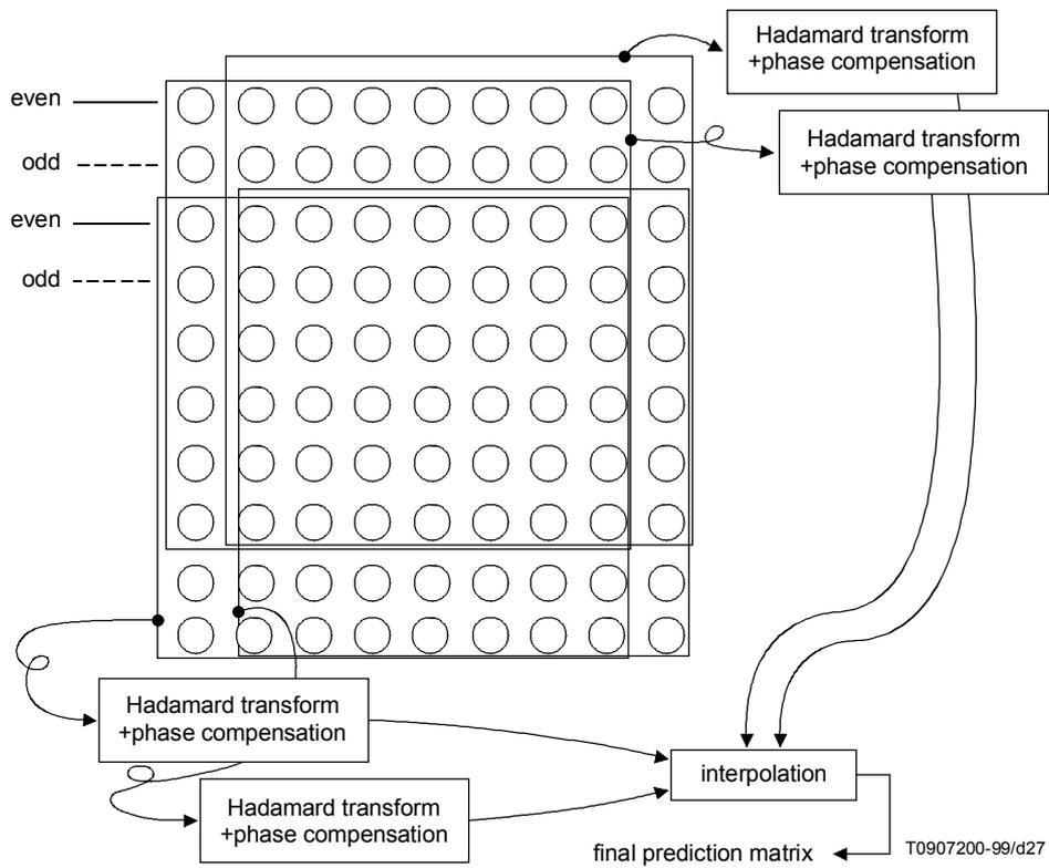
Figure A.2-14/J.88 – Concept of interpolation process on Hadamard transformation structure
