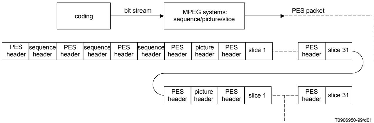
**Figure A.1-1/J.88 – Outline of coding bit stream structure**
