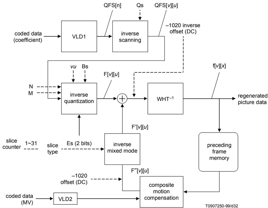
Figure A.3-1/J.88 – Whole structure of decoding process
