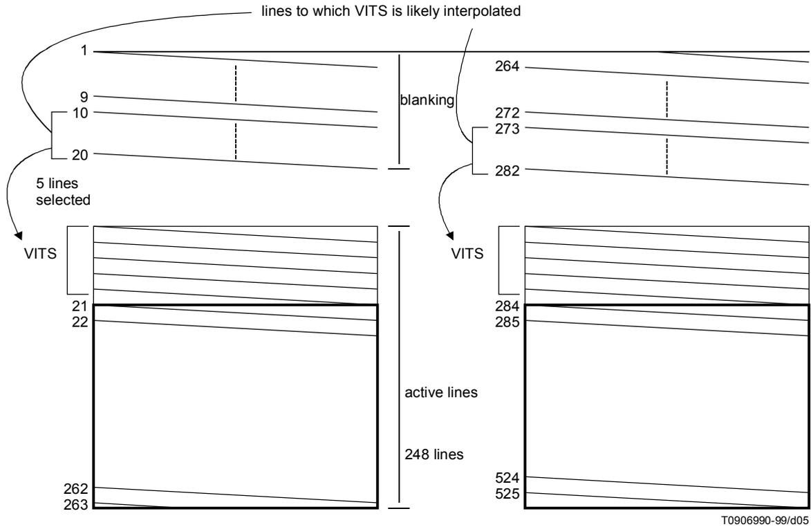
Figure A.1-3/J.88 – Removal of vertical blanking period signal
