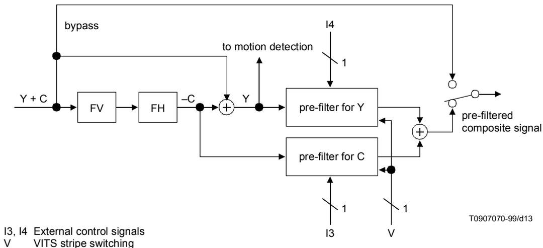
Figure A.2-2/J.88 – Structure of Y/C separation type pre-filter
