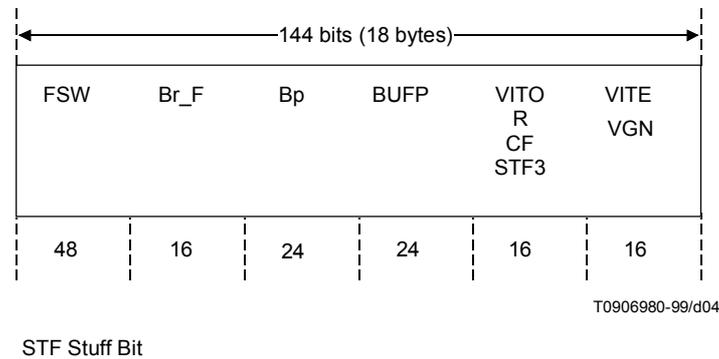
**Figure A.1-2/J.88 – Structure of picture header**
