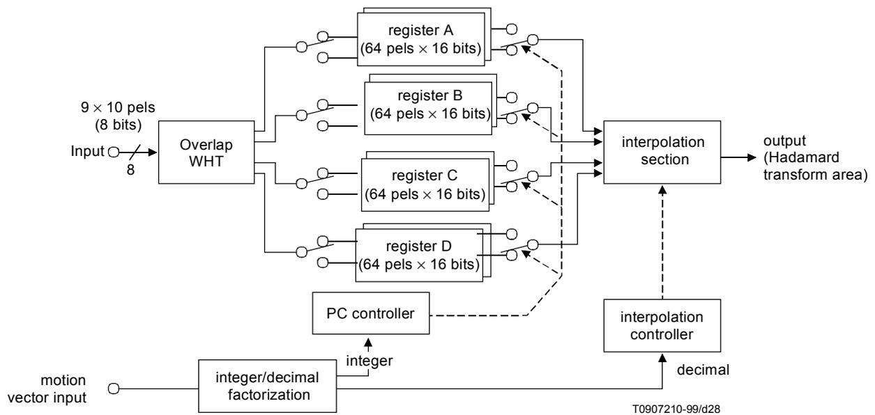
Figure A.2-15/J.88 – Structure of composite motion compensation
