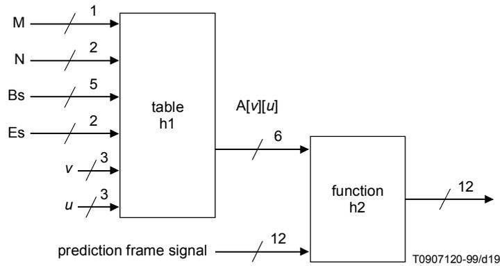
**Figure A.2-6/J.88 – Structure of prediction value conversion**
