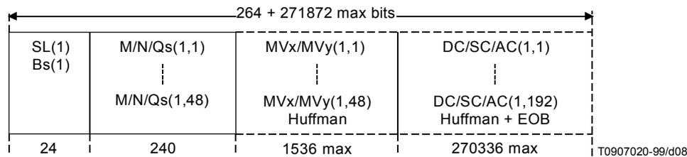
**Figure A.1-6/J.88 – Internal structure of a slice**
