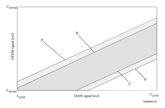
Figure A.3/J.87 – Range of signal level for adjacent QAM/OFDM signals at subscriber's tapoff
