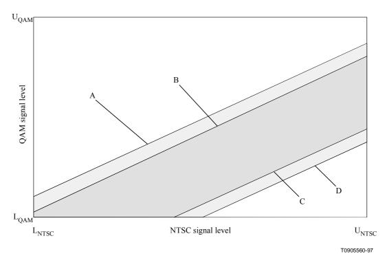
Figure A.1/J.87 – Range of signal level for adjacent NTSC/QAM signals at subscriber's tapoff
