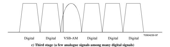
Figure 1/J.87 – Reference model for evolution of hybrid analogue/digital links
