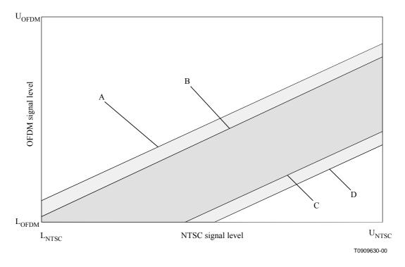
Figure A.2/J.87 – Range of signal level for adjacent NTSC/OFDM signals at subscriber's tapoff
