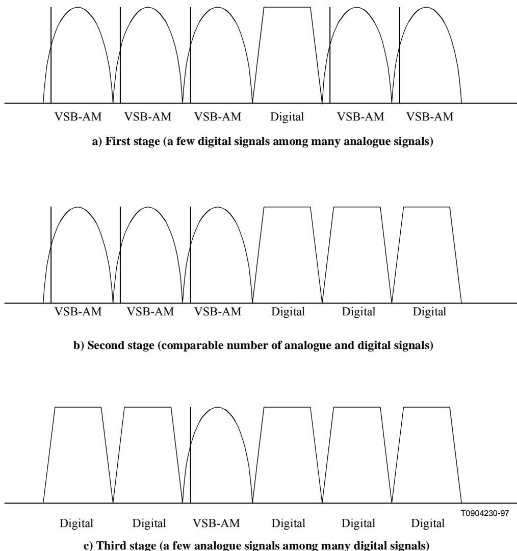
**Figure 1/J.87 – Reference model for evolution of hybrid analogue/digital links**
