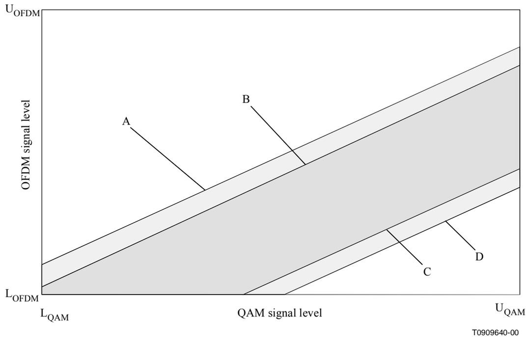
**Figure A.3/J.87 – Range of signal level for adjacent QAM/OFDM signals at subscriber's tapoff**
