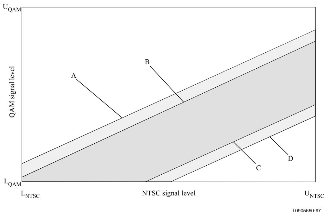
**Figure A.1/J.87 – Range of signal level for adjacent NTSC/QAM signals at subscriber's tapoff**
