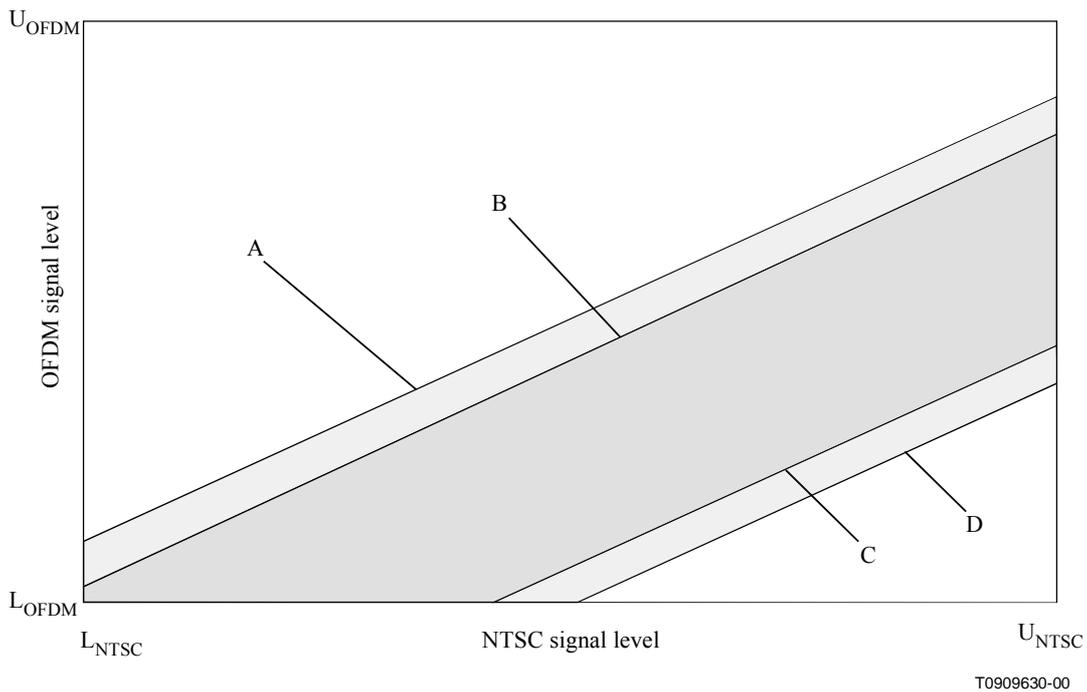
**Figure A.2/J.87 – Range of signal level for adjacent NTSC/OFDM signals at subscriber's tapoff**
