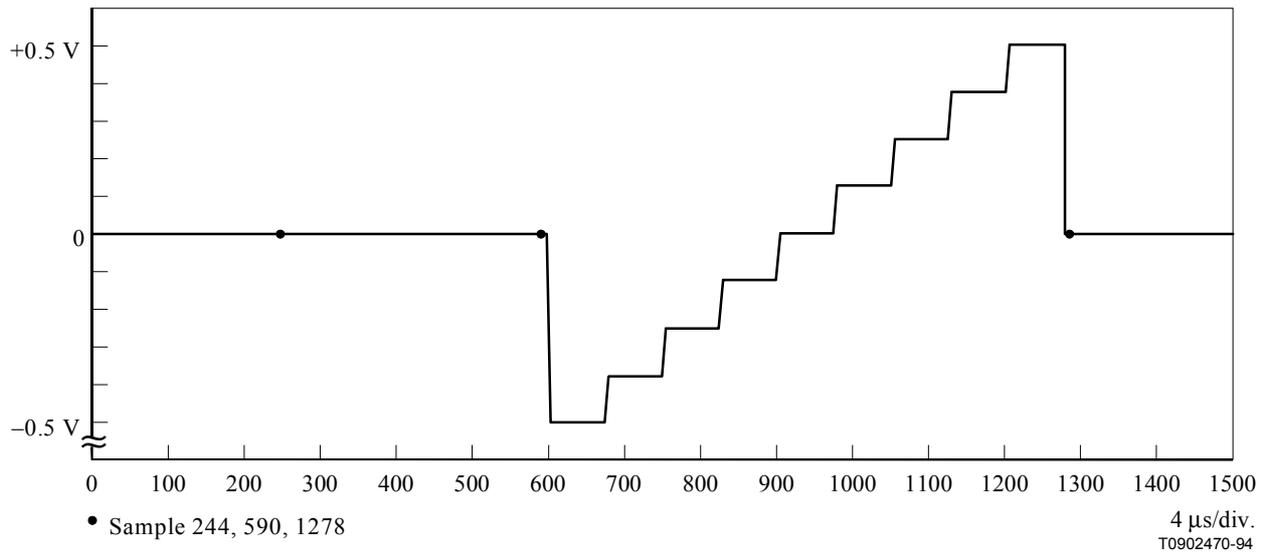
**Figure A.5/J.67 – Test signal No. 5**
