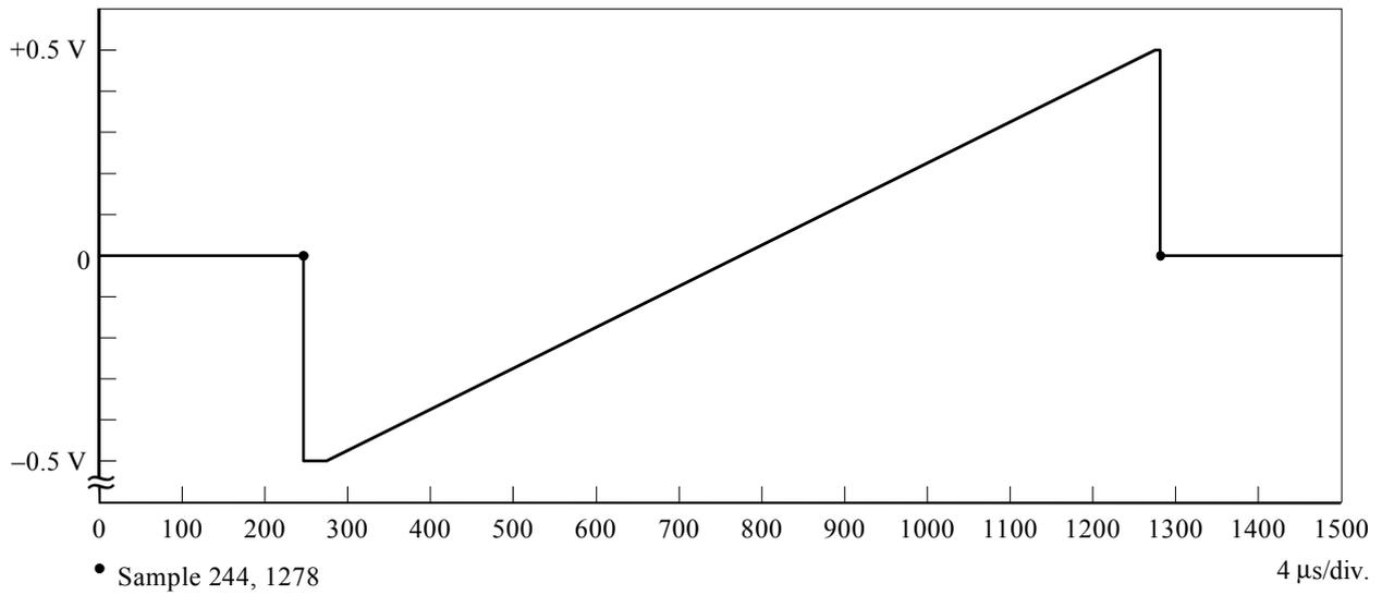
a) Test signal No. 2a – Even frame
