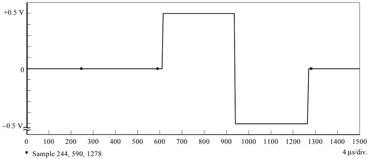
**b) Test signal No. 1b – Odd frame**
