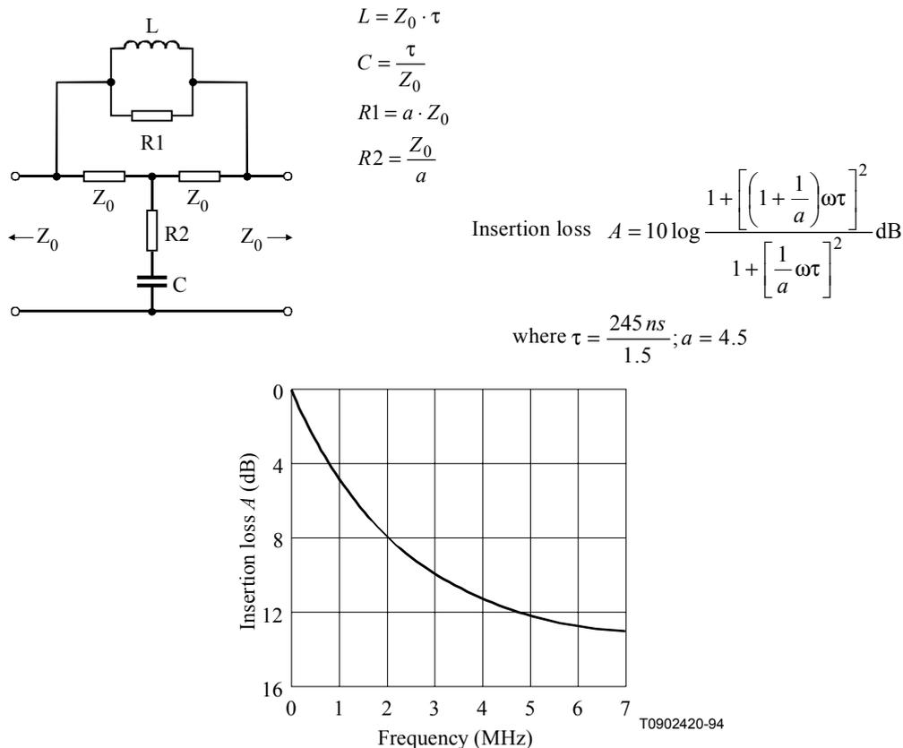
**Figure 1/J.67 – Unified random noise weighting filter for MAC circuits using a compression ratio of 3:2**
