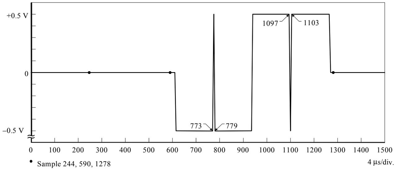
**b) Test signal No. 1a – Even frame**
