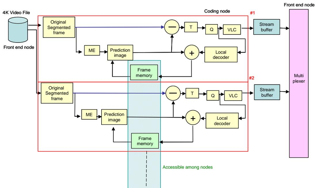
Figure II.I – Block diagram of the example encoder system
