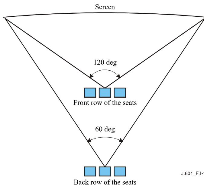
**Figure I.1/J.601 – Horizontal viewing angle of the IMAX system**
