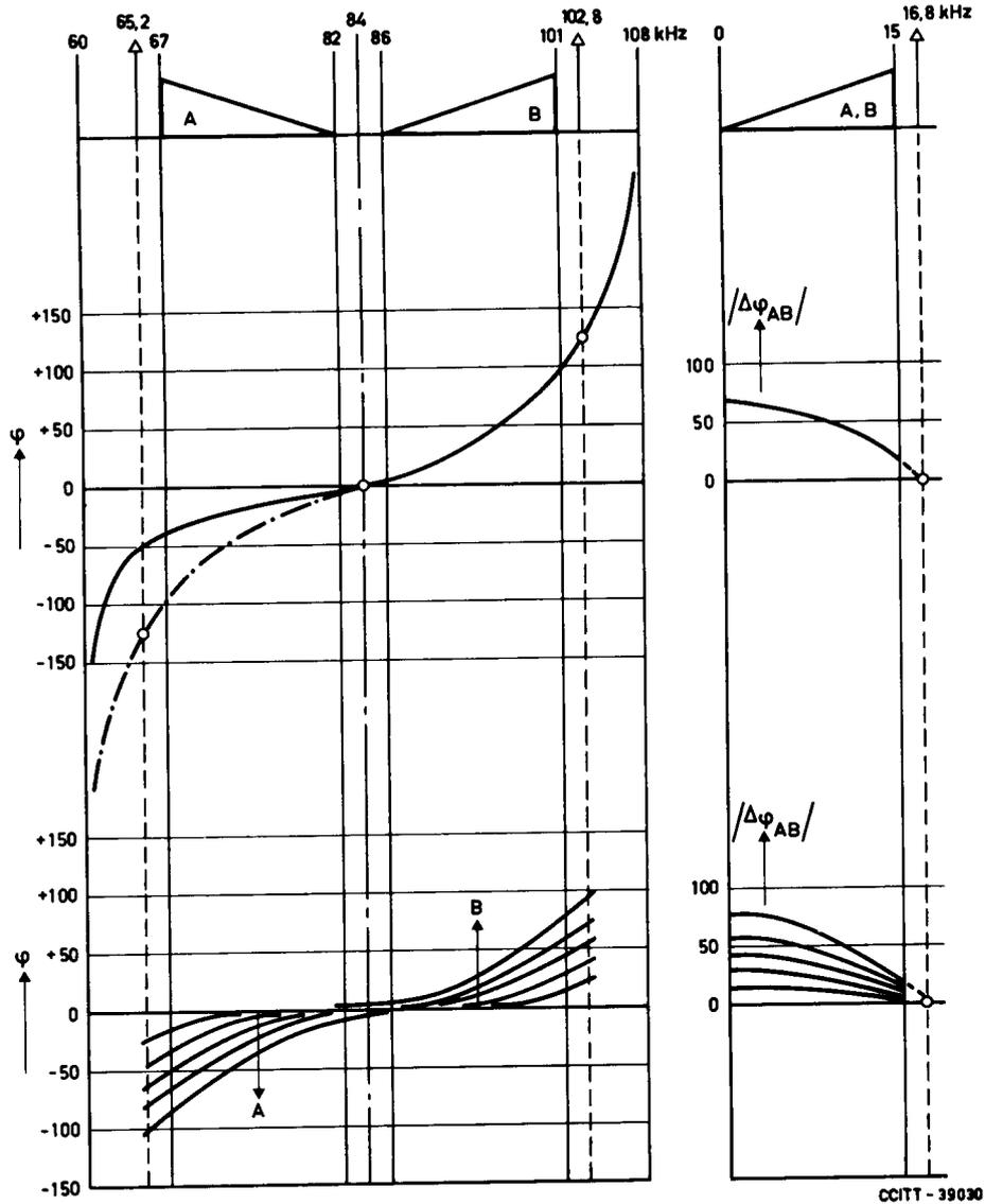
Top: Example of phase symmetry distortion. Ideal skew-symmetric phase characteristic shown.
