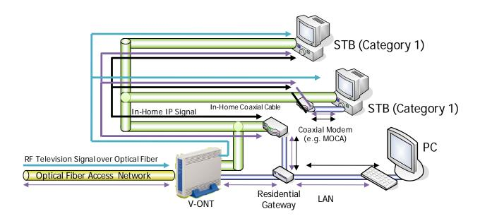
Figure II.2 – Home networking with IP-based access network and RF-based content signal
