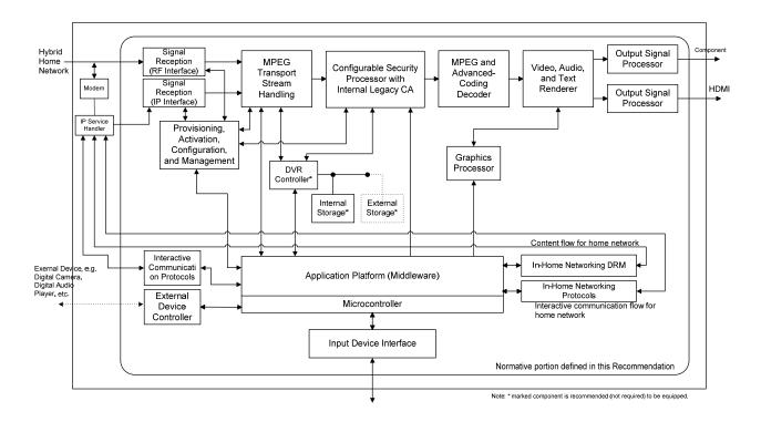
Figure I.2 – Functional block diagram of hybrid STB with a single network interface using a home network coaxial modem
