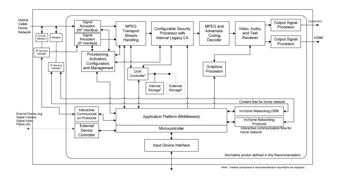
Figure I.4 – Functional block diagram of hybrid STB with an embedded DOCSIS cable modem and an embedded home network coaxial modem for IP home networking
