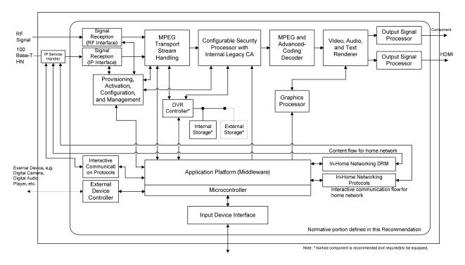
Figure I.1 – Functional block diagram of hybrid STB with a dual network interface
