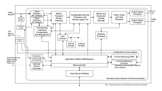
Figure I.3 – Functional block diagram of hybrid STB with an embedded DOCSIS cable modem
