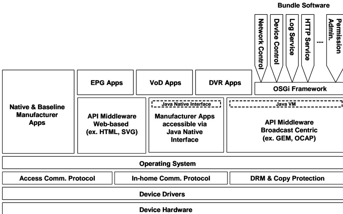
**Figure V.1 – A relationship between STB protocol stacks and bundle software**
