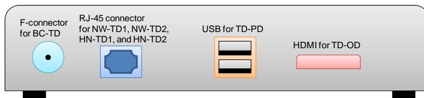
**Figure 5 – Example of physical interface implementation (rear view of STB)**
