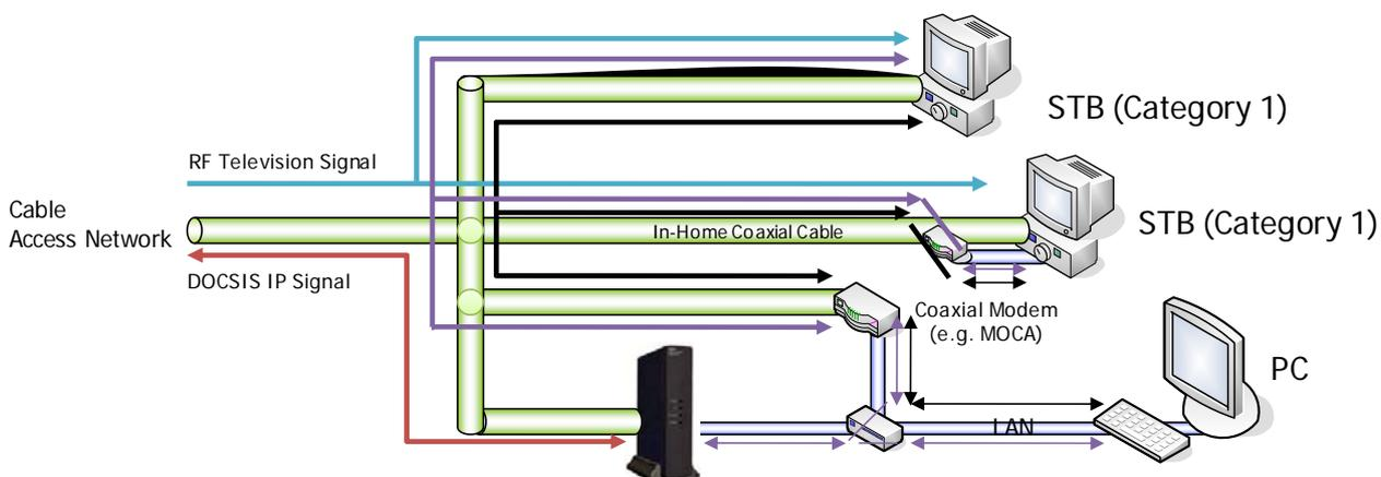
**Figure II.3 – Home networking with Cable-based access network and external DOCSIS modem**
