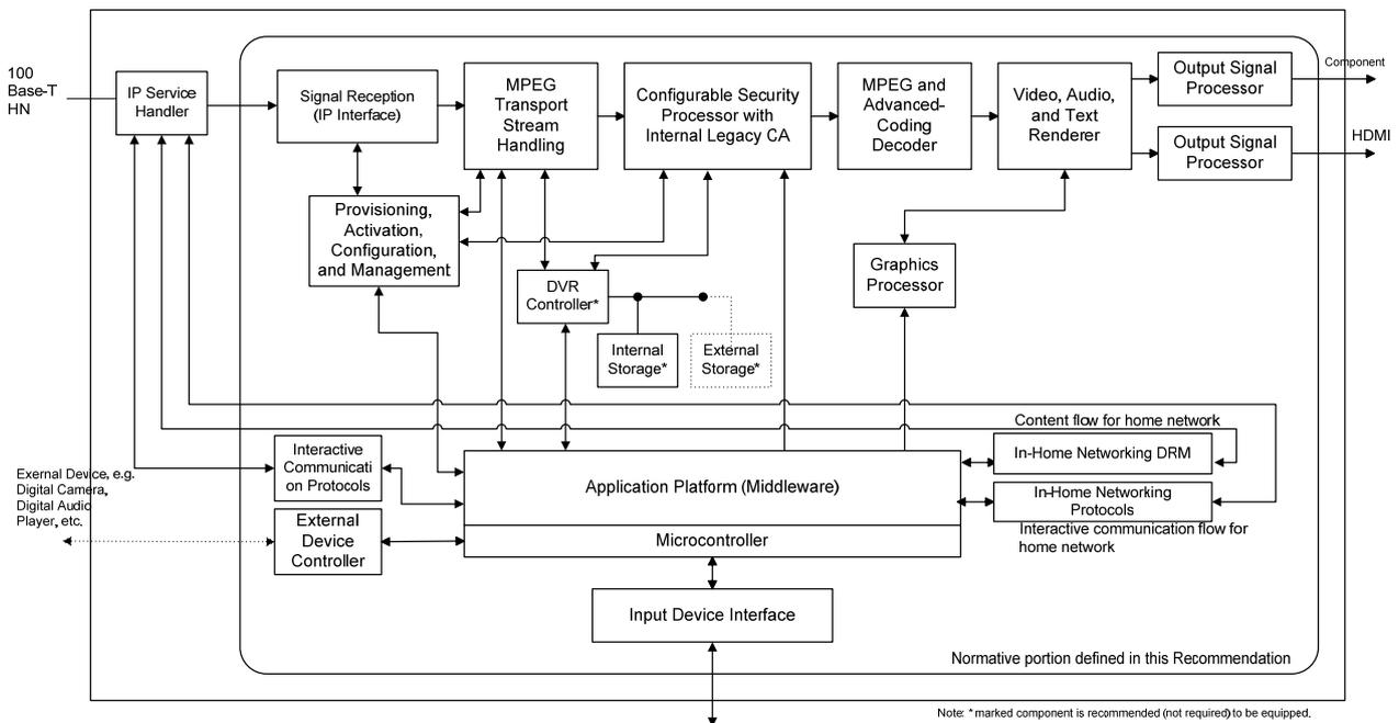
**Figure I.5 – Functional block diagram of IP-only STB**
