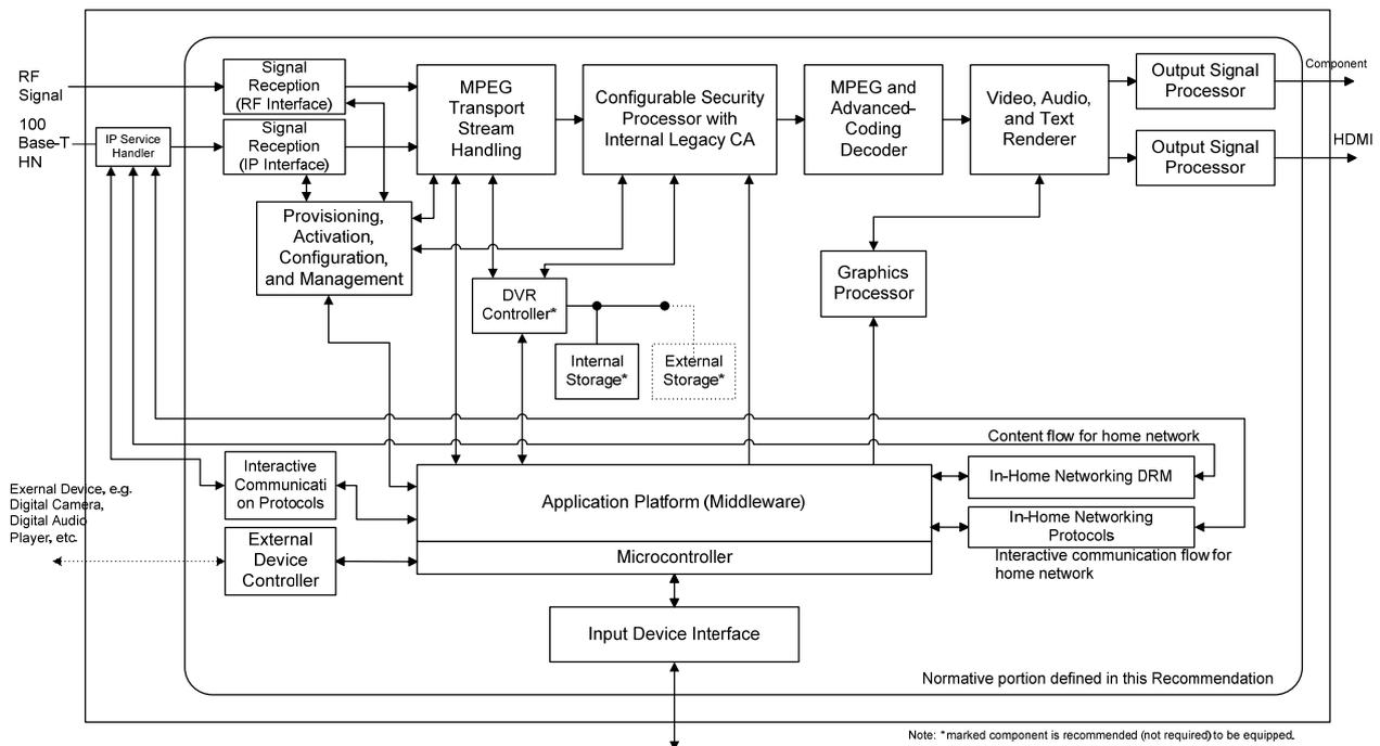
Figure I.1 – Functional block diagram of hybrid STB with a dual network interface
