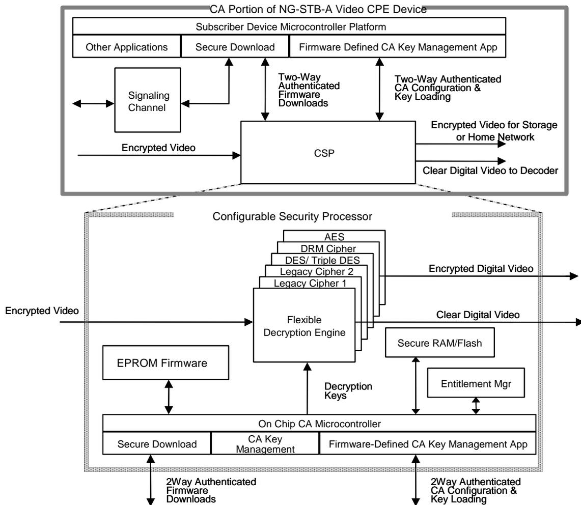
**Figure 6 – CSP Reference Model**
