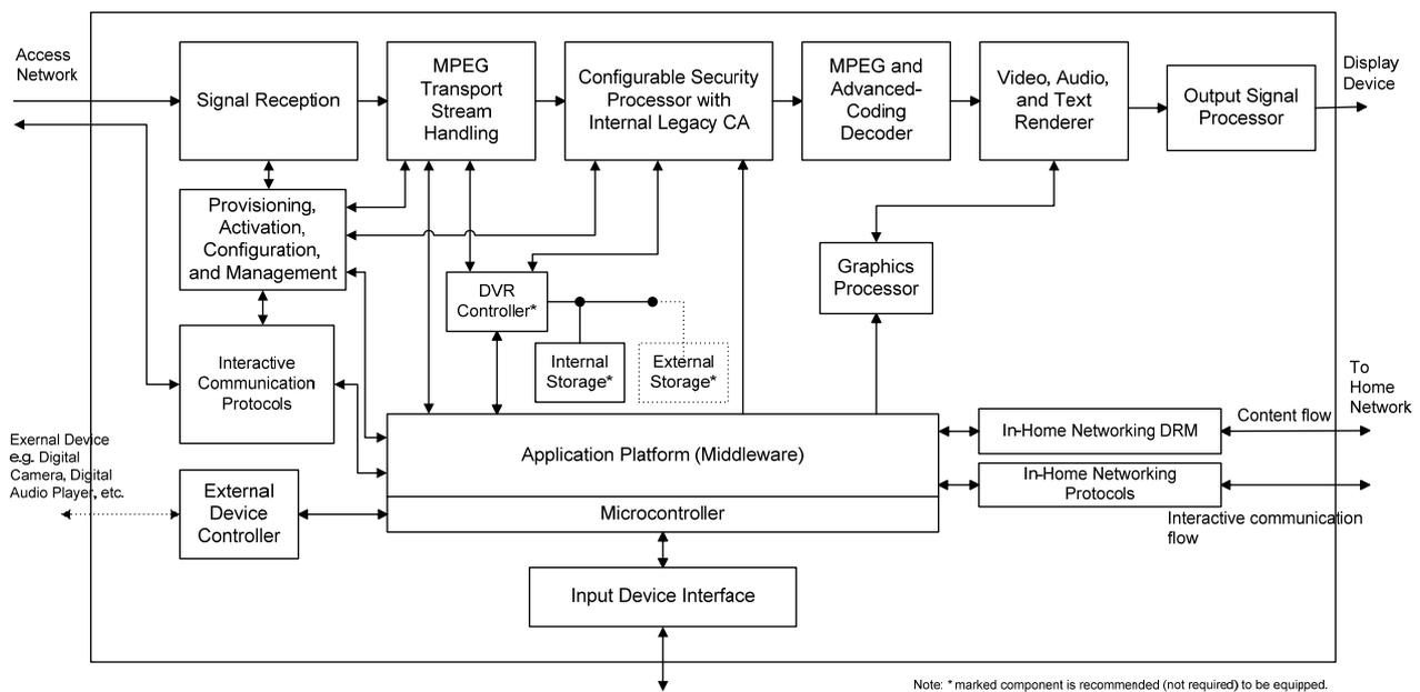
**Figure 2 – Functional Block Diagram based on [ITU-T J.290]**
