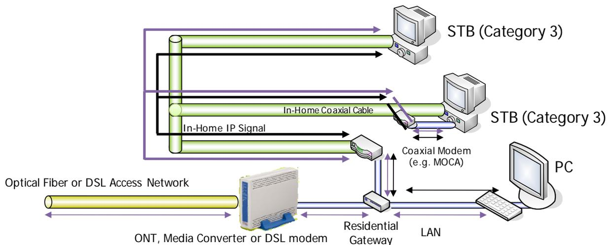
**Figure II.1 – Home networking with IP-based access network**
