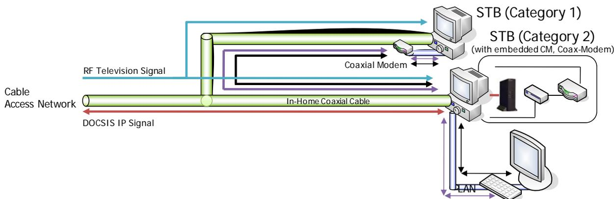
**Figure II.4 – Home networking with Cable-based access network and embedded DOCSIS modem**
