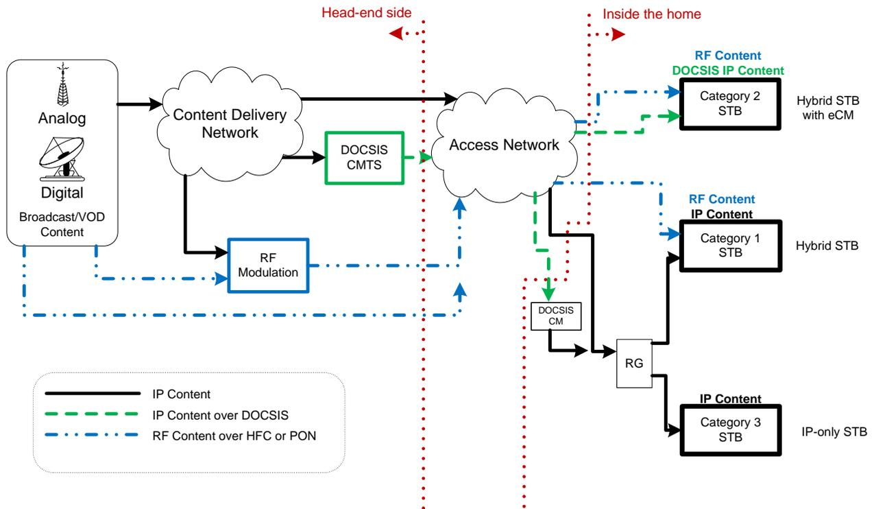
**Figure 1 – Client devices in an assumed content distribution network: content flow aspect**
