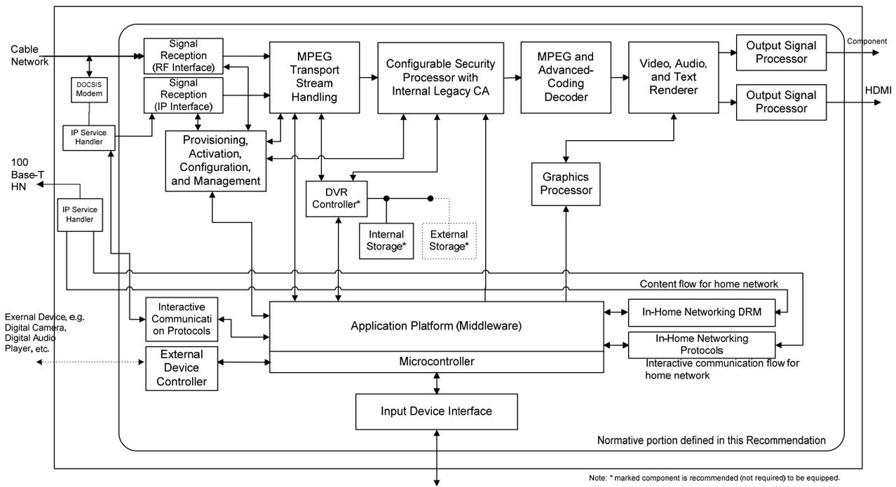
**Figure I.3 – Functional block diagram of hybrid STB with an embedded DOCSIS cable modem**
