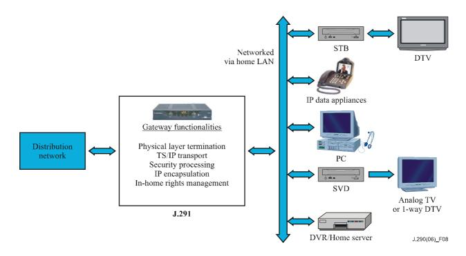
Figure 8 – Examples of CPE deployment for subscriber with IP-based home data network (In-home DRM system is applied)
