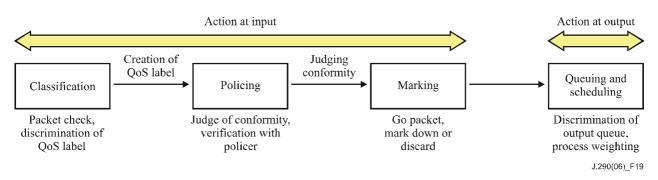
Figure 19 – An Example of QoS process flow
