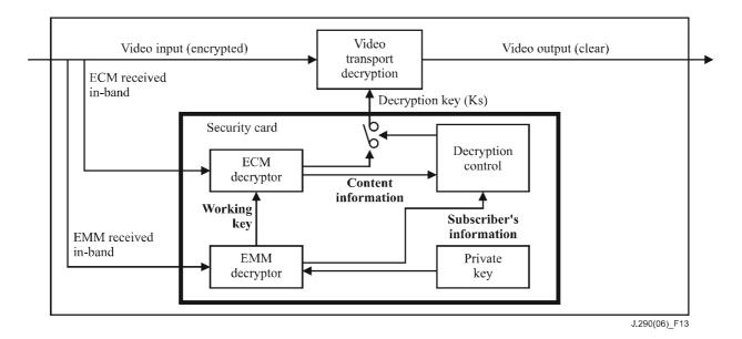
Figure 13 – Signal flow in use of security card
