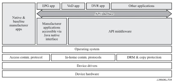
Figure 4 – Video CPE software architecture
