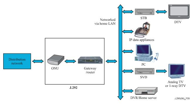
Figure 9 – Examples of CPE deployment for subscriber with IP-based home data network
