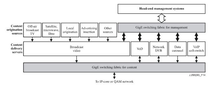
Figure 14 describes the overall head-end network delivery architecture.
