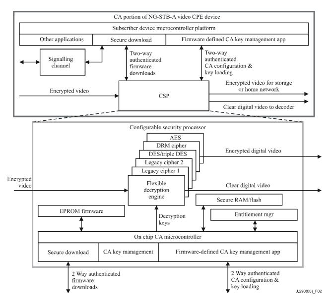
Figure 2 – Example of security block diagram
