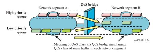
Figure 17 – Aspect of QoS class mapping
