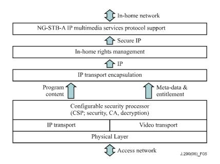
**Figure 5 – Gateway communications architecture**
