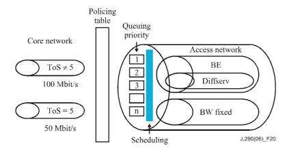
Figure 20 – An aspect of queuing priority between core network and access network
