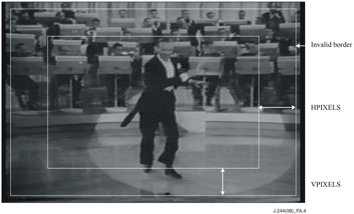
**Figure A.4 – HPIXELS and VPIXELS visually demonstrated**
