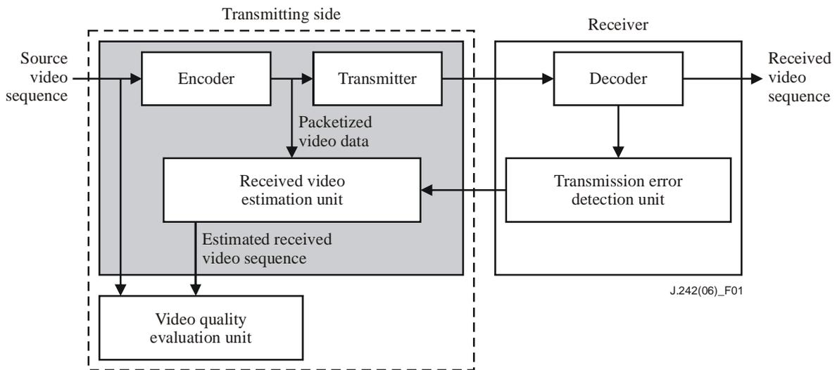
**Figure 1 – A method for a transmitting side to monitor video quality at a receiver using transmission error information**
