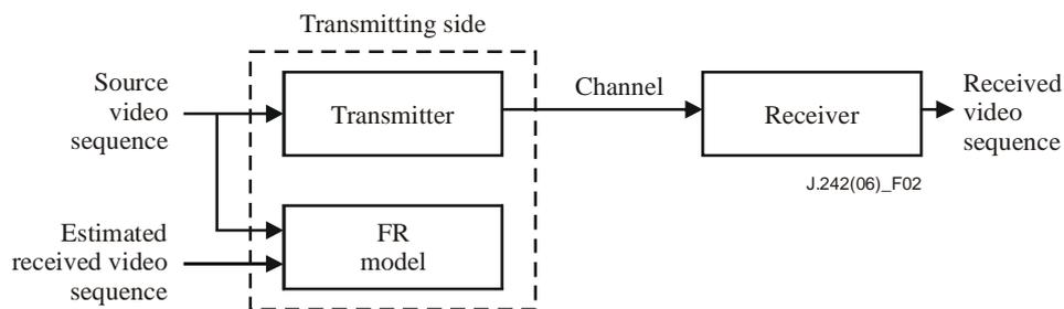
**Figure 2 – A block diagram for the transmitting side computing the video quality of the received video sequence using the estimated received video sequence (FR model)**
