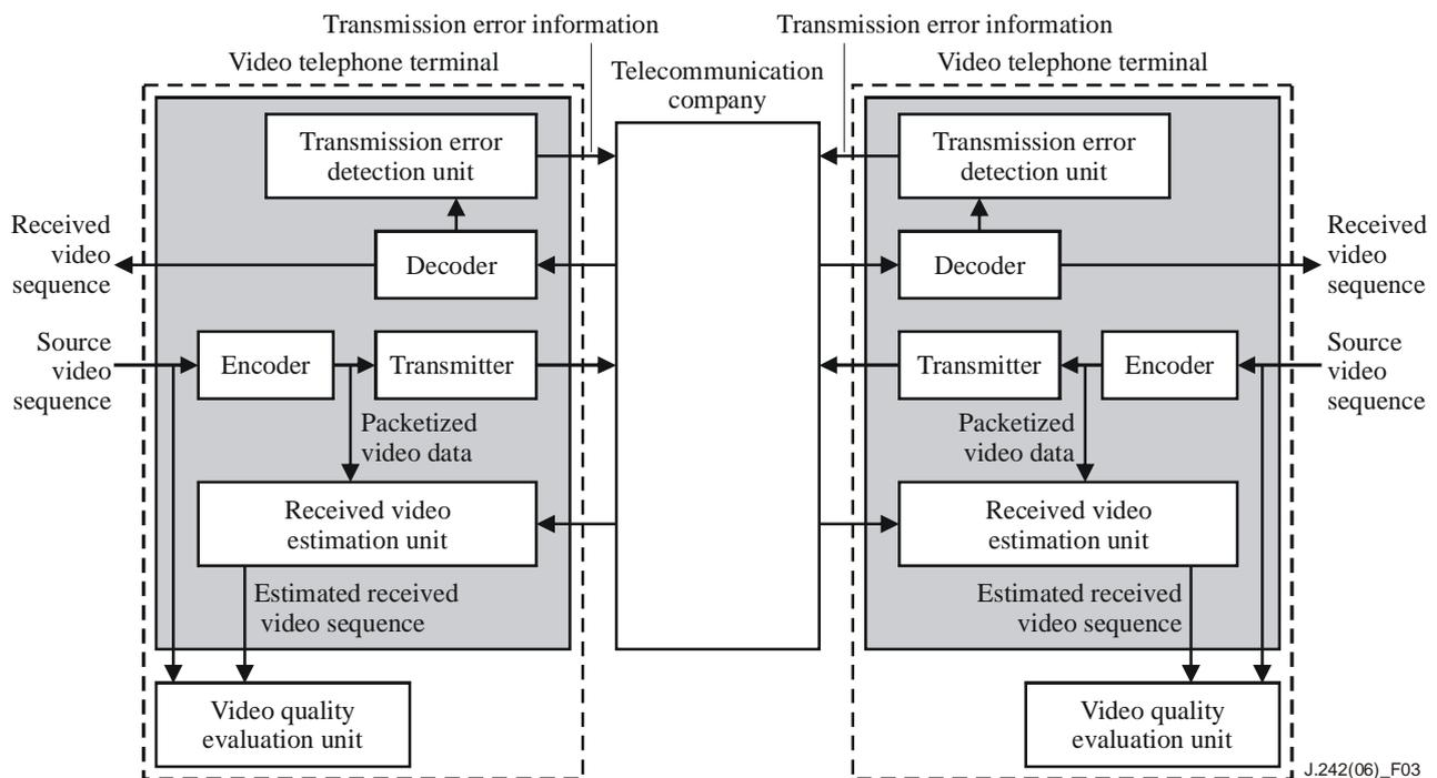
**Figure 3 – A method for a transmitting side to monitor video quality at a receiver using transmission error information (video telephony)**
