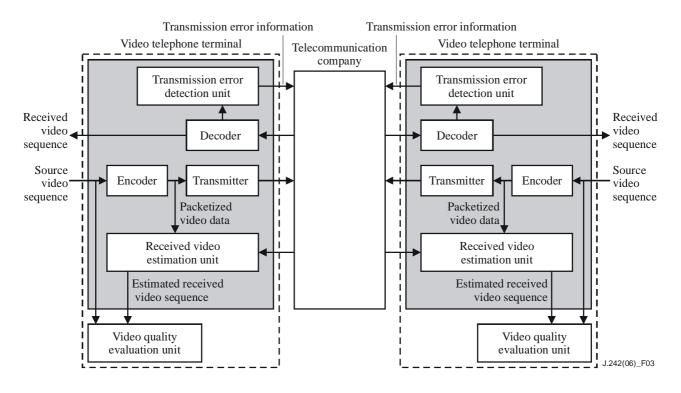
Figure 3 – A method for a transmitting side to monitor video quality at a receiver using transmission error information (video telephony)
