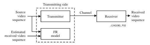
Figure 2 – A block diagram for the transmitting side computing the video quality of the received video sequence using the estimated received video sequence (FR model)
