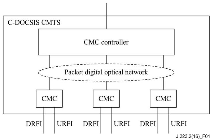
**Figure 1 – C-DOCSIS CMTS network diagram**
