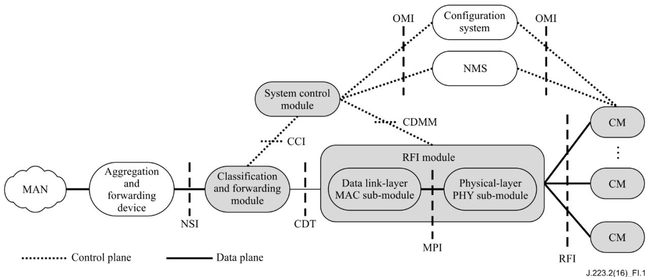
**Figure I.1 – Functional module of the C-DOCSIS system**
