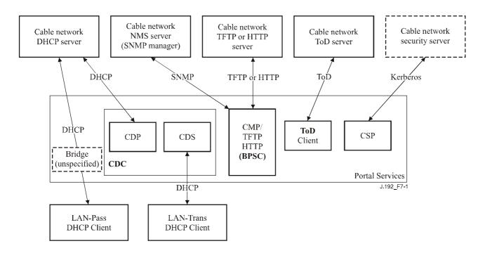
Figure 7-1/J.192 – Provisioning architecture
