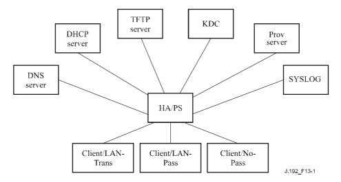
Figure 13-1/J.192 – IPCable2Home provisioning functional elements
