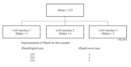
Figure 6-6/J.192 – ifStack implementation example
