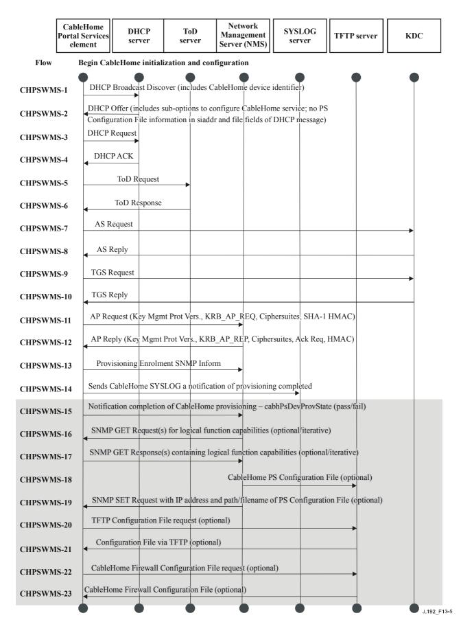
Figure 13-5/J.192 – Provisioning process for PS management – SNMP Provisioning Mode
