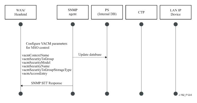
Figure 12-6/J.192 – PS configuration (VACM parameters) sequence
