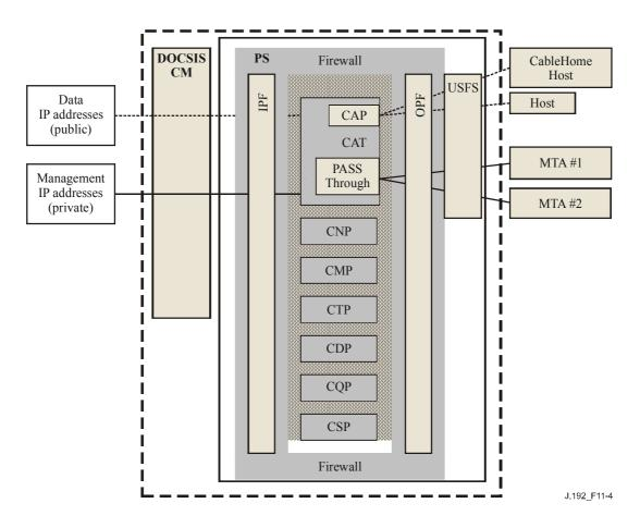
Figure 11-4/J.192 – Firewall functionality inside the PS
