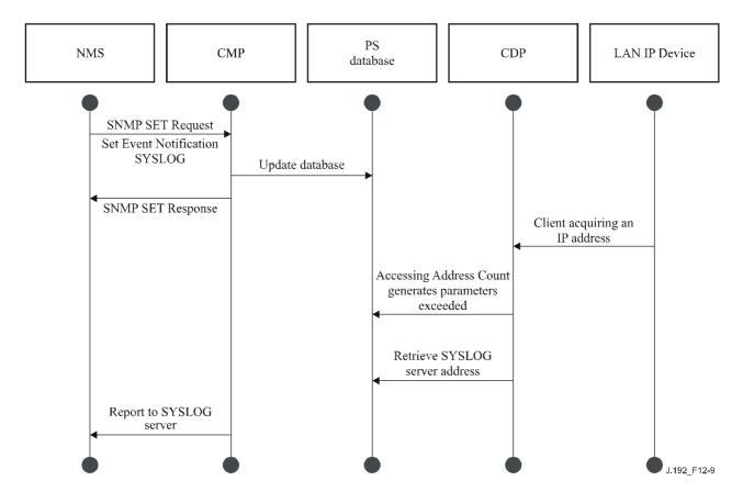
Figure 12-9/J.192 – Address acquisition (Request exceeds provisioned count) sequence
