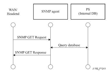
Figure 12-3/J.192 – PS Database access from the PS WAN-Man interface sequence diagram
