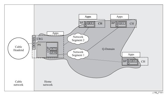
Figure 10-1/J.192 – Example of CqoS functional elements
