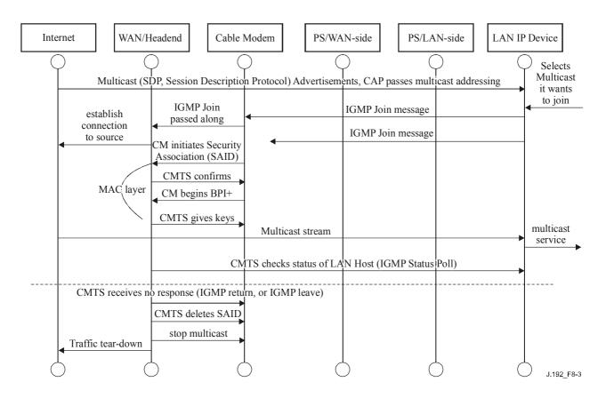
Figure 8-3/J.192 – Multicast via IGMP sequence
