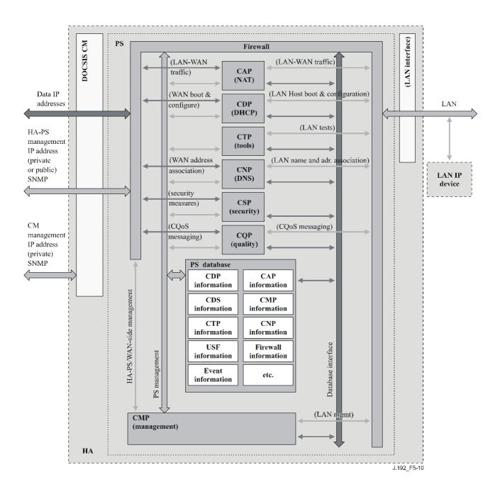
Figure 5-10/J.192 – PS database detailed example implementation
