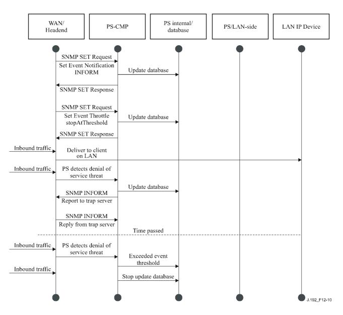
Figure 12-10/J.192 – CMP event throttling and limiting operation
