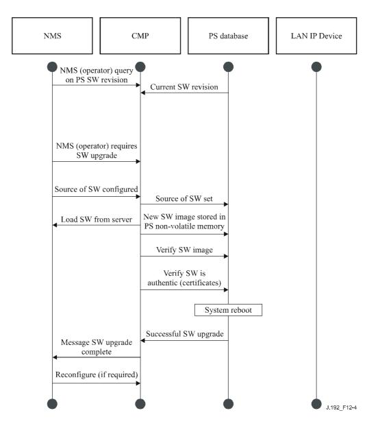
Figure 12-4/J.192 – PS software download sequence diagram
