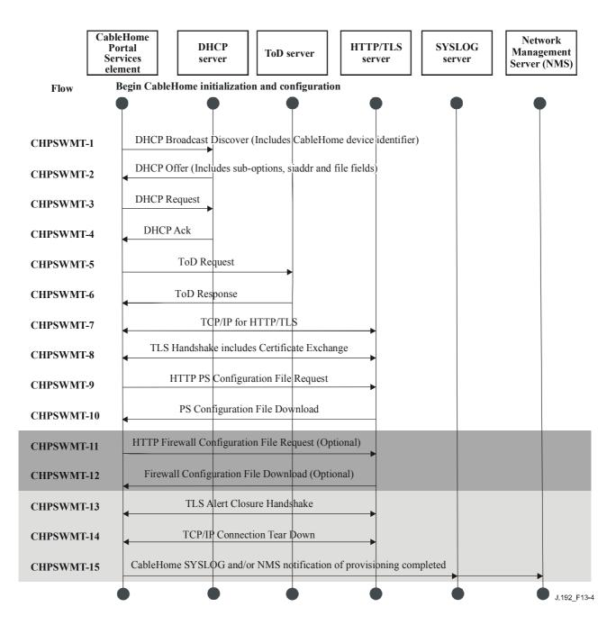
Figure 13-4/J.192 – Provisioning process DHCP Provisioning Mode using HTTP/TLS
