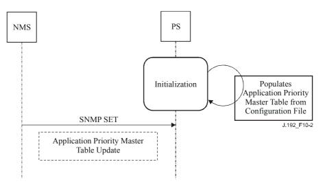
Figure 10-2/J.192 – WAN information exchange and processing at the PS
