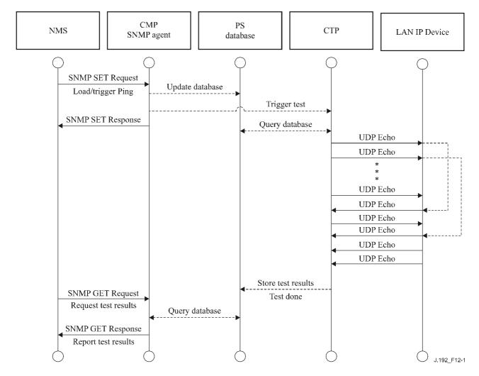
Figure 12-1/J.192 – Connection Speed Tool Process sequence diagram
