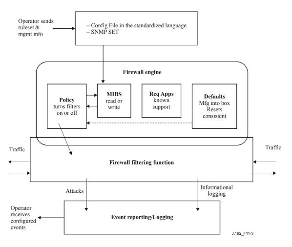
Figure 11-3/J.192 – Firewall logical reference
