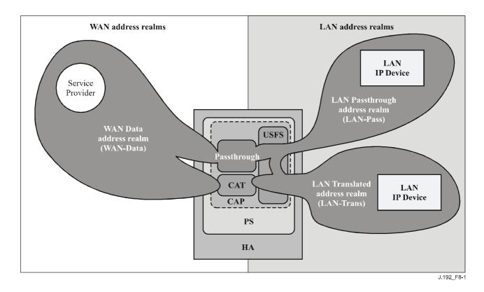
Figure 8-1/J.192 – IPCable2Home Address Portal (CAP) functions
