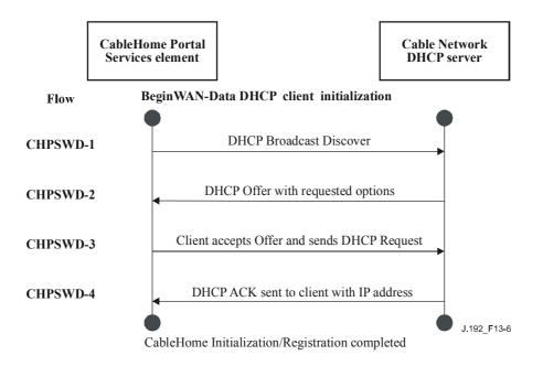
Figure 13-6/J.192 – PS WAN-Data provisioning process
