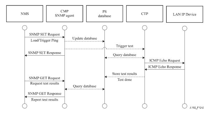
Figure 12-2/J.192 – Ping Tool process sequence diagram
