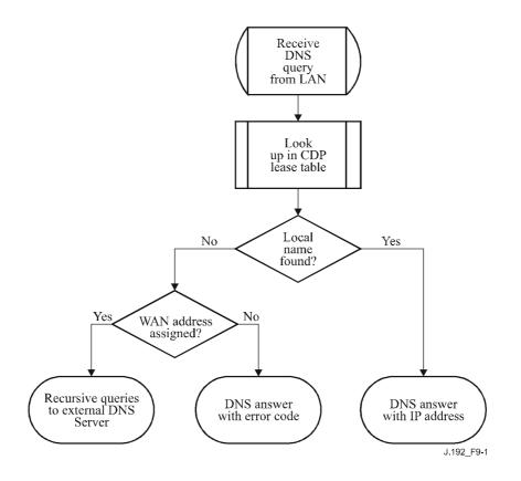
Figure 9-1/J.192 – CNP packet processing
