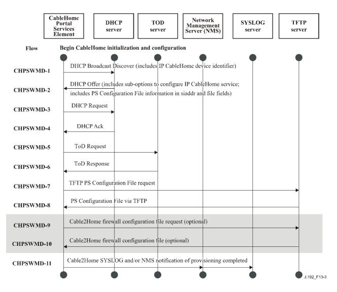
Figure 13-3/J.192 – Provisioning process for PS management – DHCP Provisioning Mode
