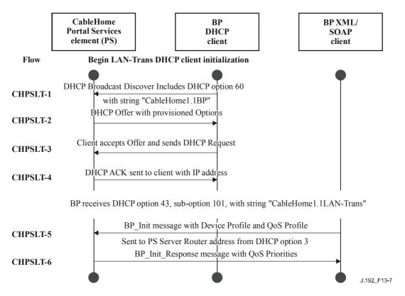
Figure 13-7/J.192 – Provisioning process for a BP in the LAN-Trans realm
