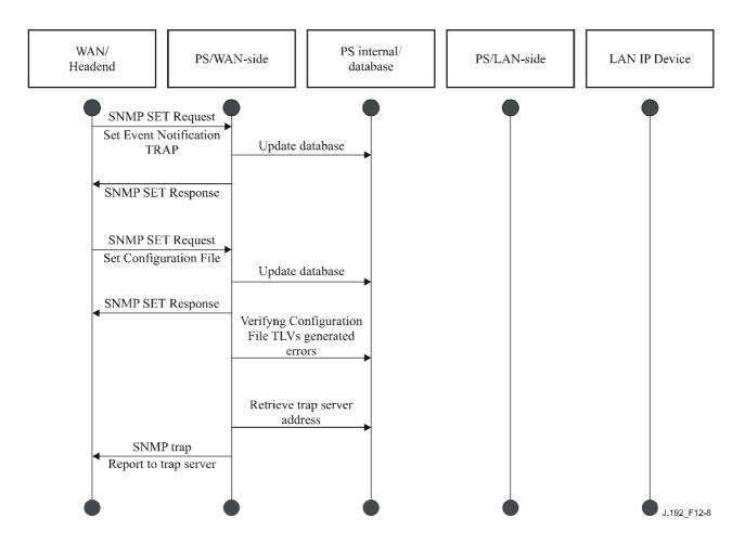
Figure 12-8/J.192 – PS Configuration File download (with invalid TLVs) sequence
