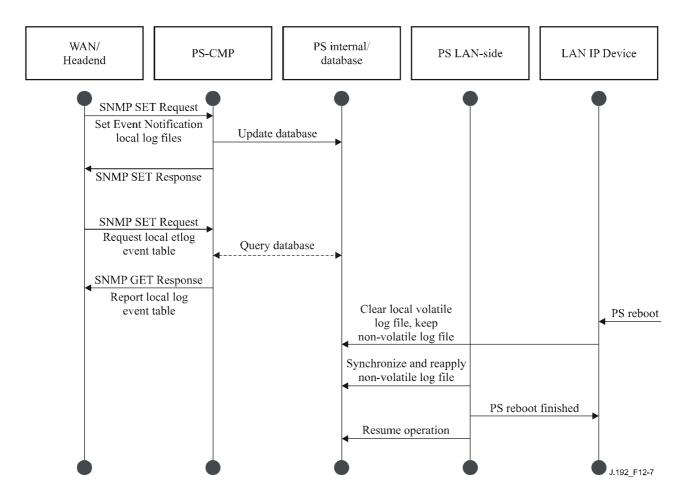
Figure 12-7/J.192 – PS configuration (Event control) sequence
