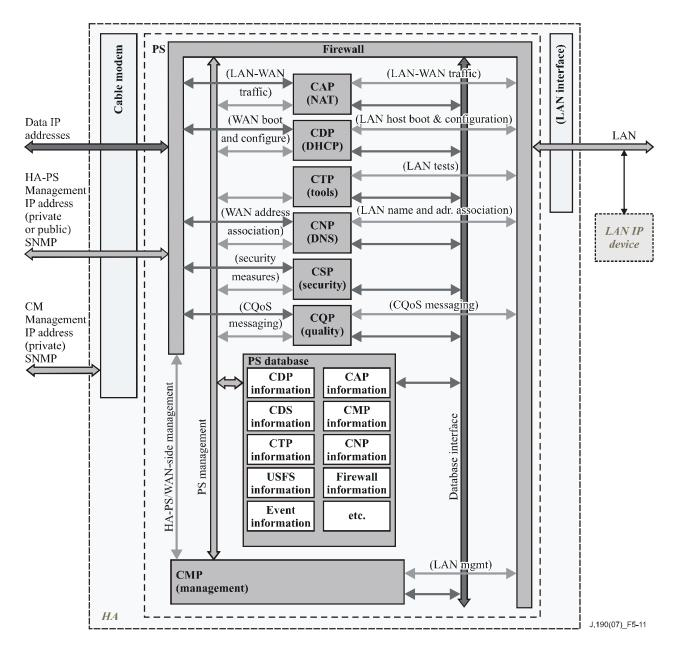
Figure 5-11 – PS database detailed example implementation for cable access network
