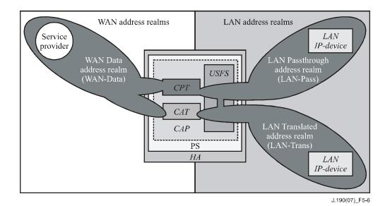
Figure 5-6 – IPNet2Home address portal (CAP) functions
