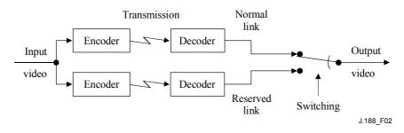
Figure 2/J.188 – Method for improvement in transmission efficiency
