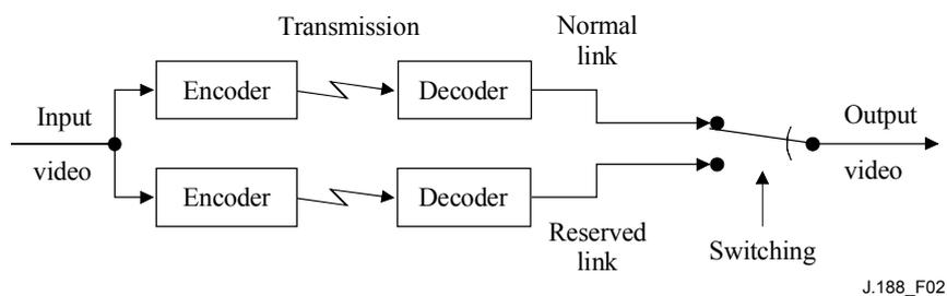
Figure 2/J.188 – Method for improvement in transmission efficiency
