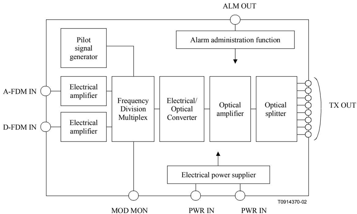
**Figure 4/J.186 – Block diagram of TX**
