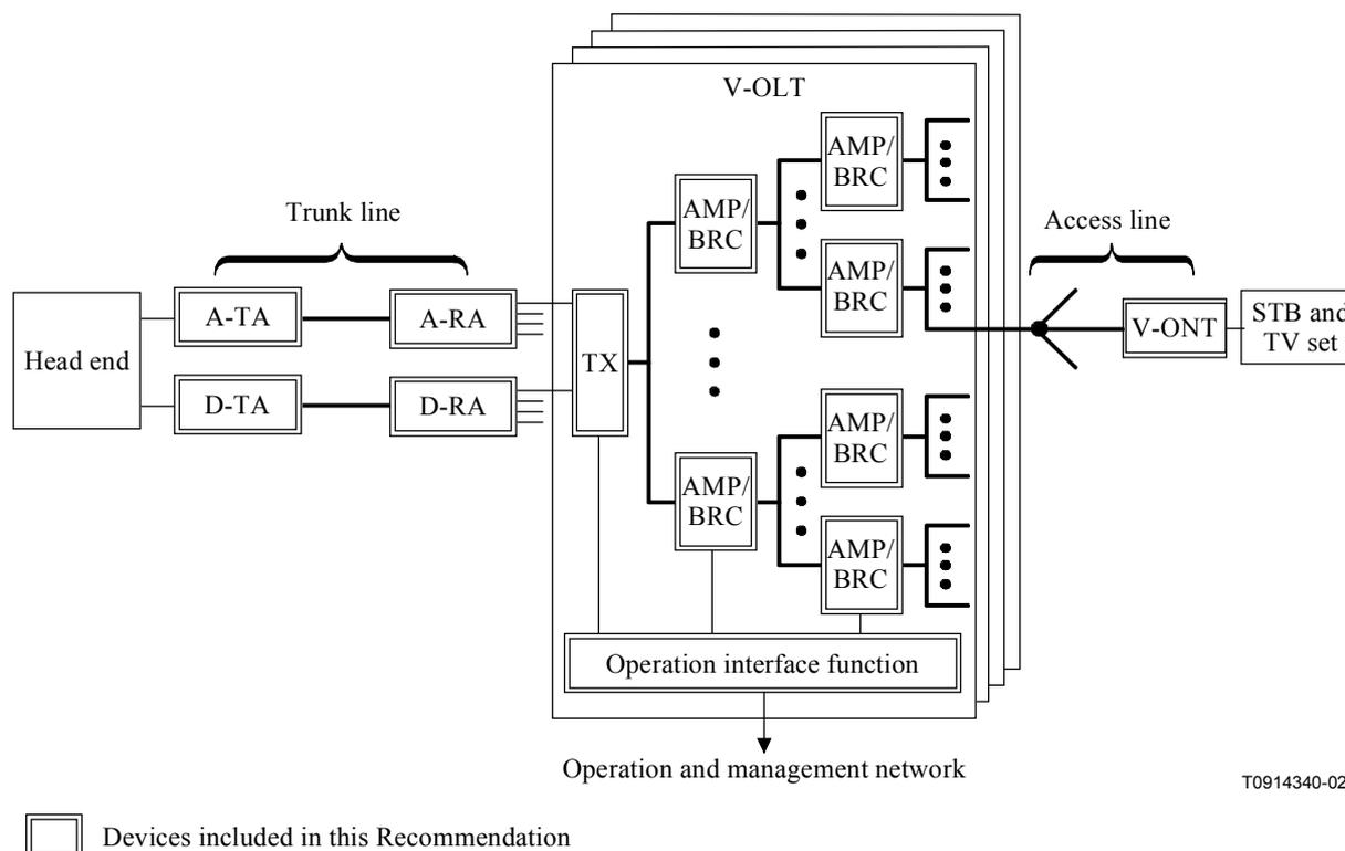
**Figure 1/J.186 – Configuration of the SCM multi-channel video signal transmission system**
