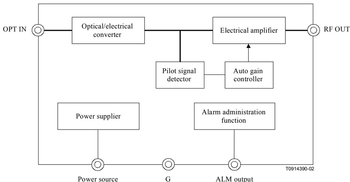
**Figure 6/J.186 – Block diagram of V-ONT**
