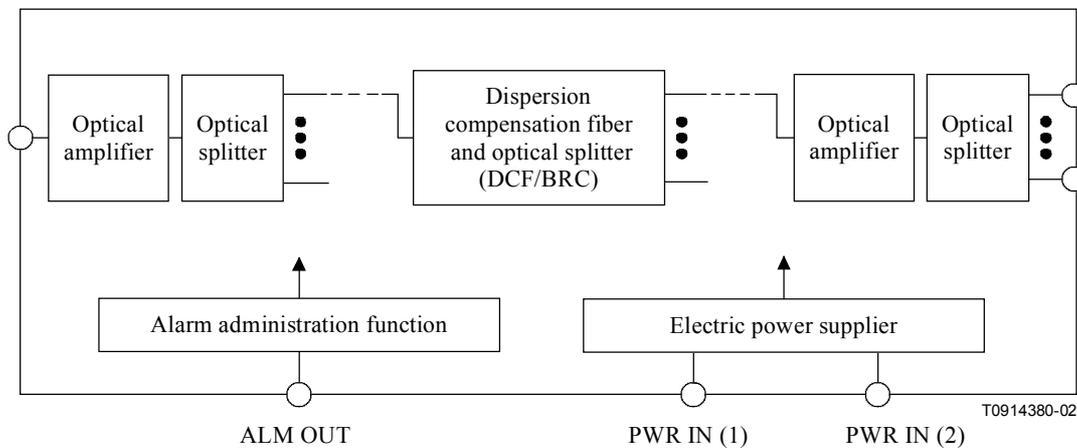
**Figure 5/J.186 – Block diagram of AMP/BRC**
