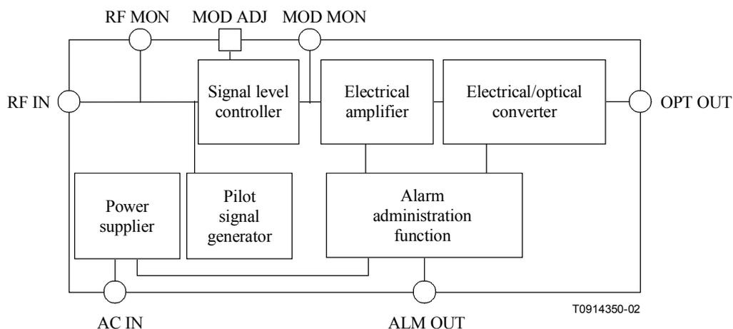
**Figure 2/J.186 – Block diagram of TA**
