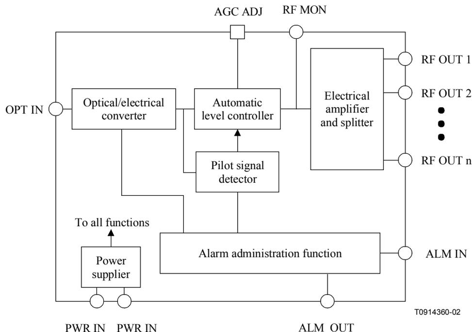
**Figure 3/J.186 – Block diagram of RA**
