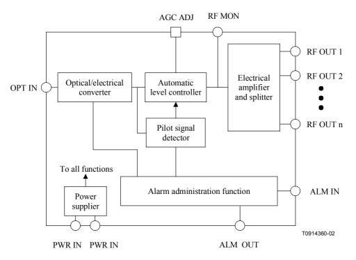
Figure 3/J.186 – Block diagram of RA
