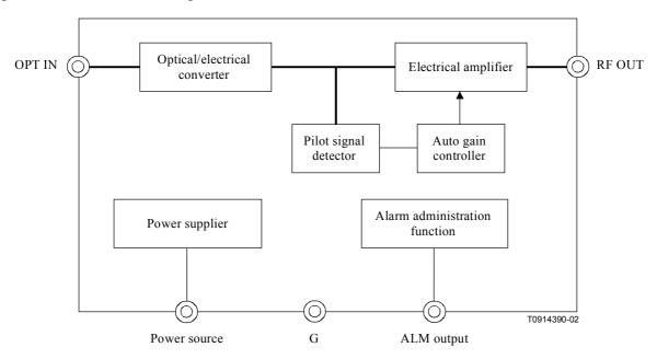
Figure 6/J.186 – Block diagram of V-ONT
