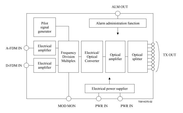
Figure 4/J.186 – Block diagram of TX
