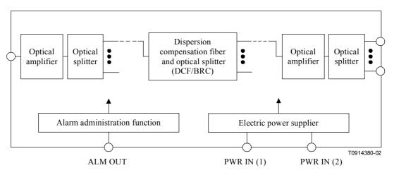
Figure 5/J.186 – Block diagram of AMP/BRC
