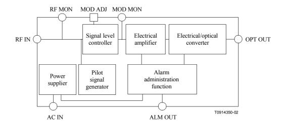
Figure 2/J.186 – Block diagram of TA
