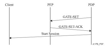
Figure 7/J.179 – Sample signalling of gate-set
