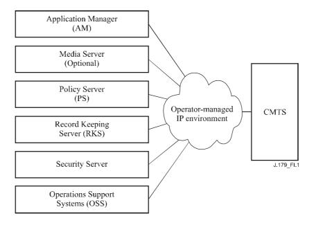
Figure I.1/J.179 – Operator multimedia network elements
