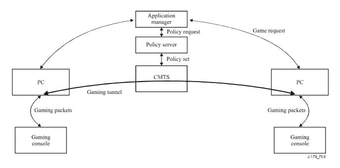
Figure I.6/J.179 – Gaming consoles networked via a QoS-enhanced IP tunnel
