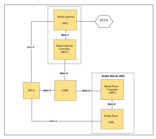
Figure 23. Audio Server Components and Interfaces
