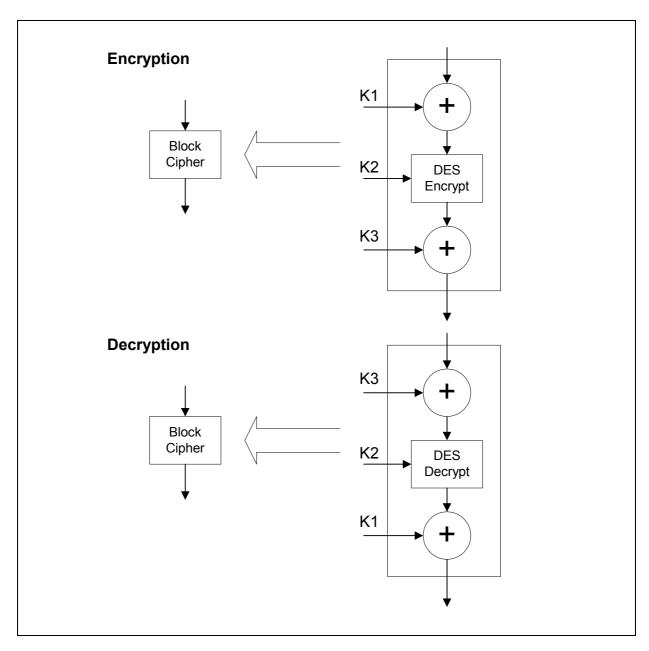
Figure 28. DESX-XEX as Block Cipher
