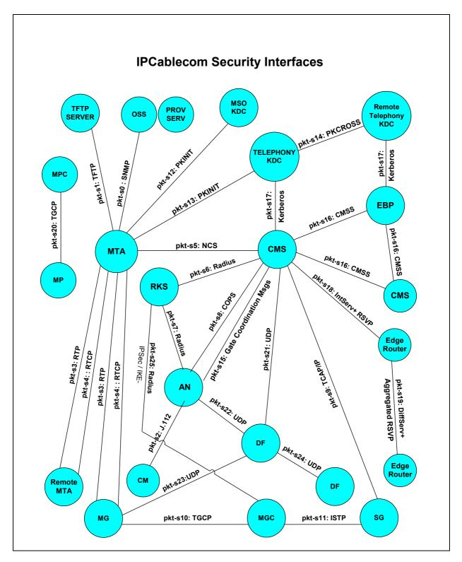
Figure 2. IPCablecom Secured Interfaces
