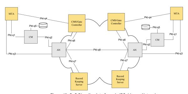
Figure 12: QoS Signaling Interfaces in IPCablecom Network
