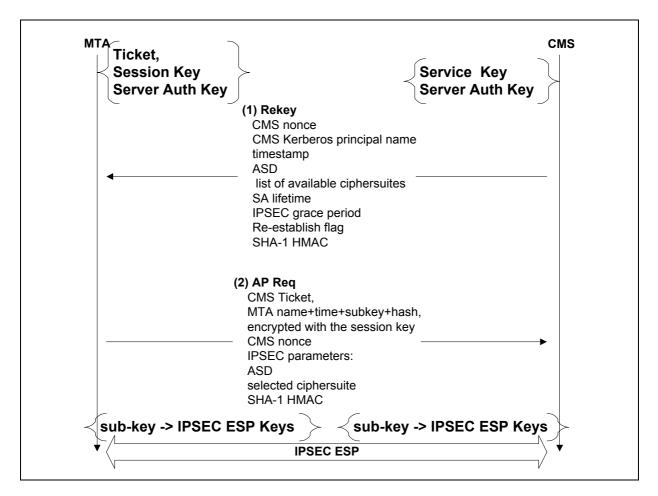
Figure 10. Rekey Message to Establish a Security Parameter
