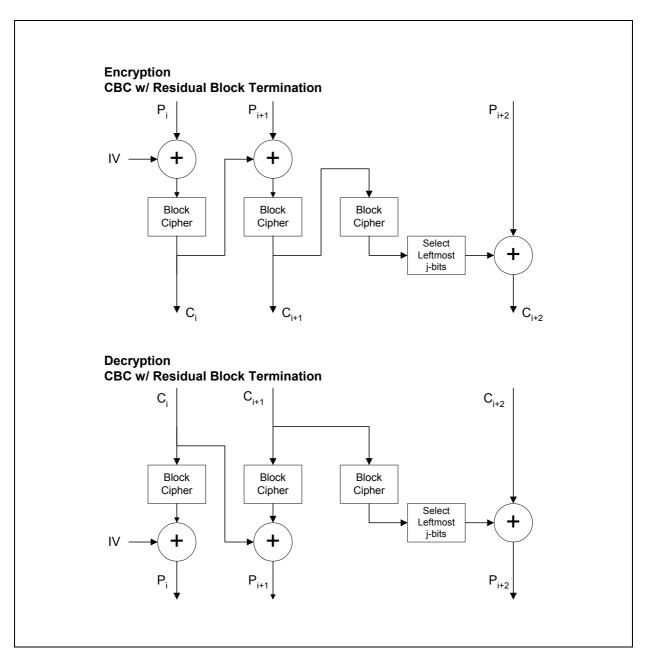
Figure 30. CBC with Residual Block Termination
