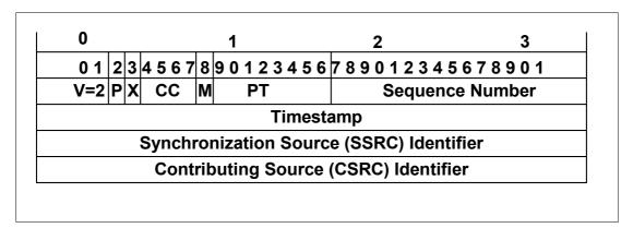
Figure 17. RTP Packet Header Format
