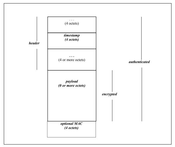
Figure 18. Format of Encoded RTP Packet
