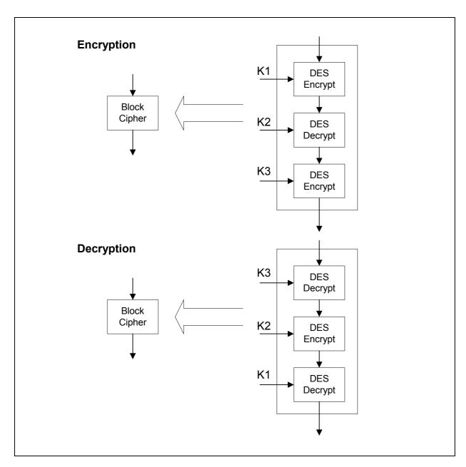
Figure 29. 3DES-EDE as Block Cipher
