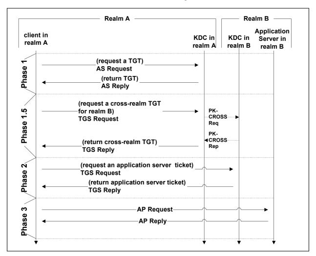
Figure 8. Kerberos Cross-Realm Operation
