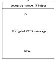
Figure 21. RTCP Encrypted Packet Format
