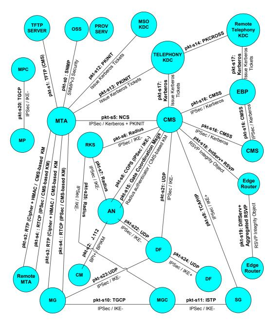
Figure 3. IPCablecom Security Interfaces with Key-Management
