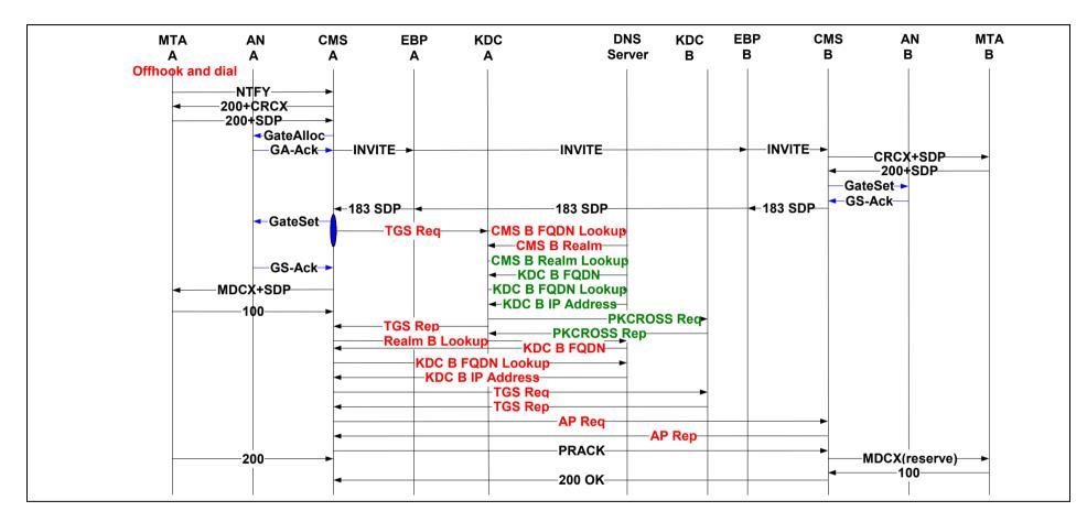
Figure 16. CMS – CMS Signaling Flow with Security
