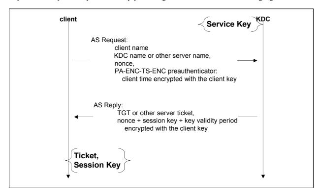
Figure 6. Symmetric-Key AS Request / AS Reply Exchange
