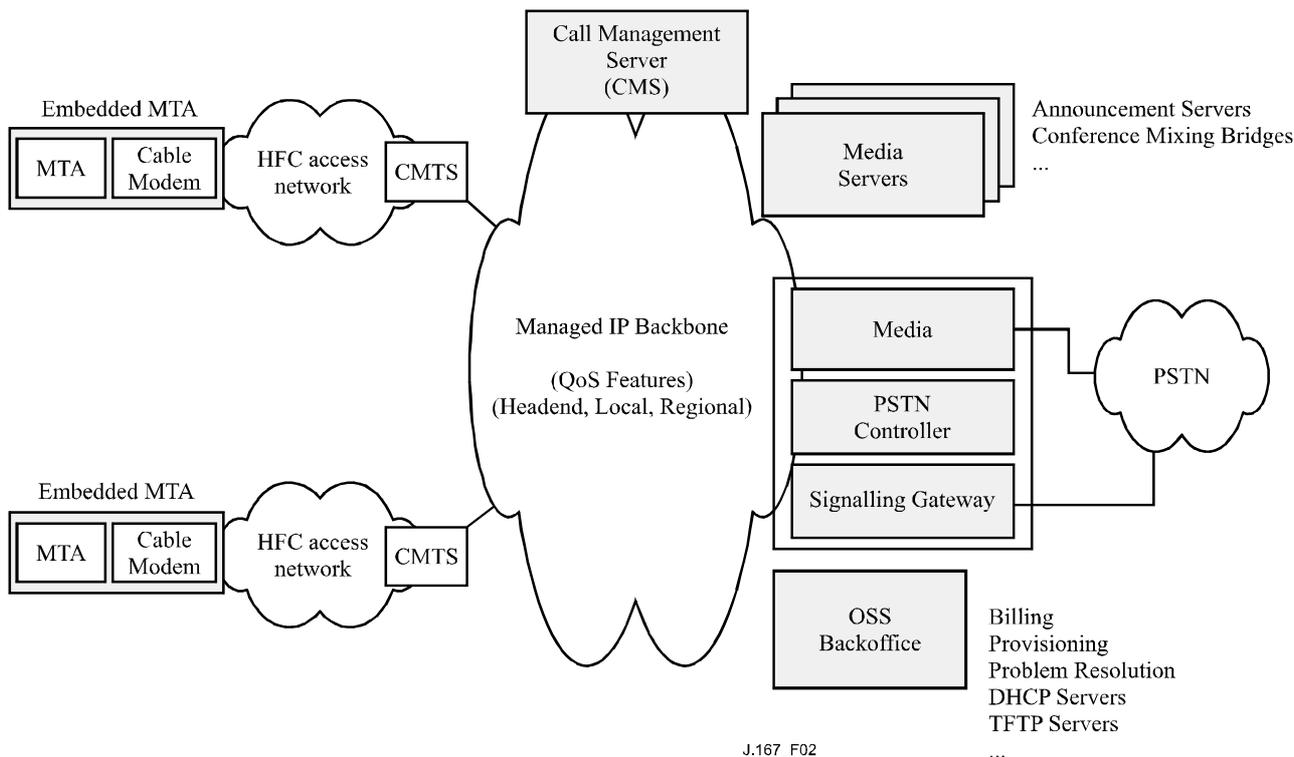
Figure 2/J.167 – IP-Cablecom network component reference model (partial)
