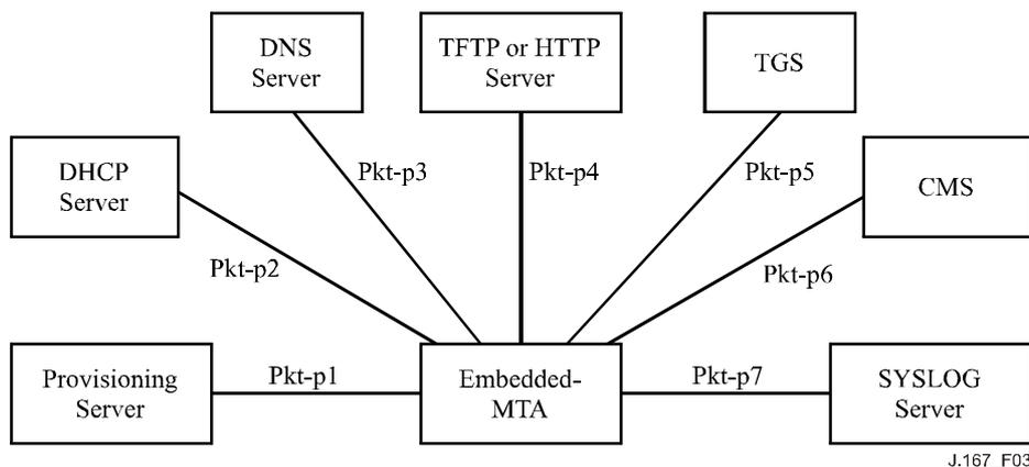
Figure 3/J.167 – IP-Cablecom provisioning interfaces
