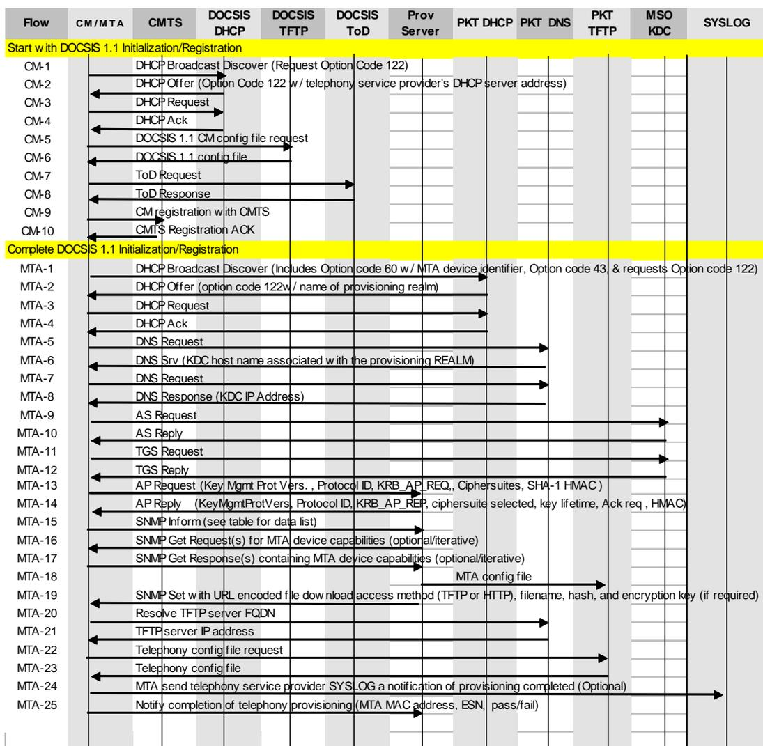
Figure 6/J.167 – Embedded-MTA secure power-on initialization flow
