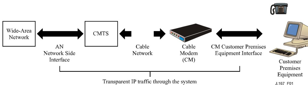
Figure 1/J.167 – Transparent IP traffic through the data-over-cable system
