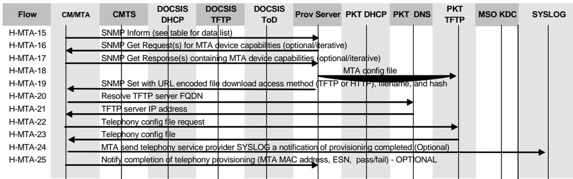
**Figure 8/J.167 – Embedded-MTA hybrid power-on initialization flow**
