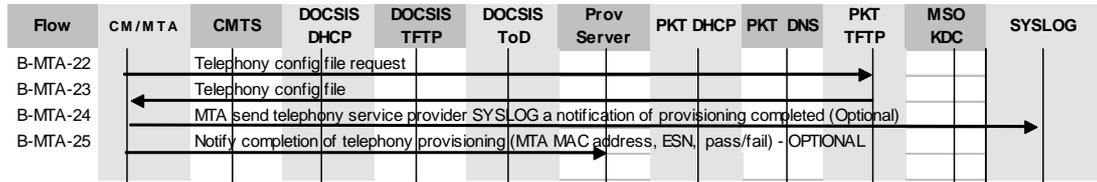
Figure 7/J.167 – Embedded-MTA basic power-on initialization flow
