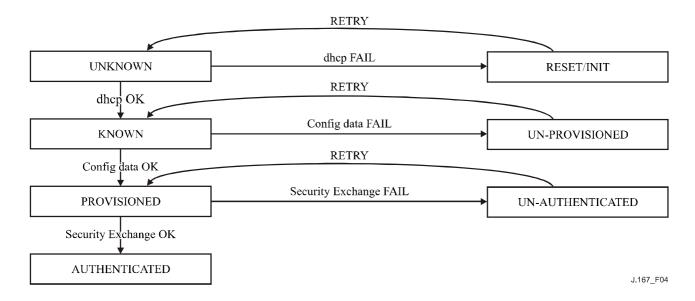
Figure 4/J.167 – Device states and state transitions for secure flow provisioning
