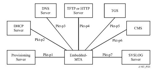
Figure 3/J.167 – IPCablecom provisioning interfaces
