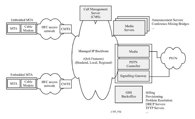
Figure 2/J.167 – IPCablecom network component reference model (partial)
