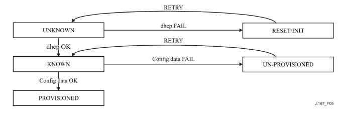
Figure 5/J.167 – Device states and state transitions for basic and hybrid flow provisioning
