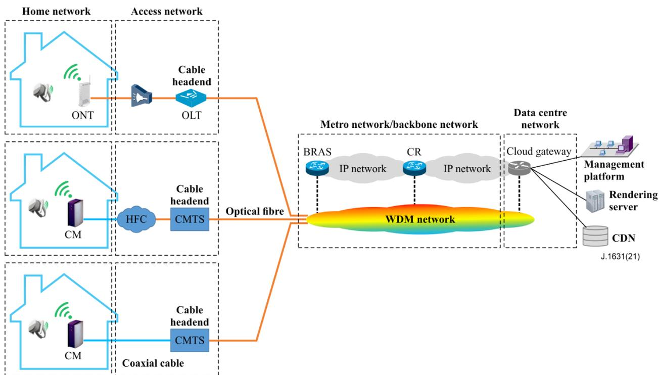
Legend: ONT – optical network terminal; OLT – optical line terminal; CM – cable modem; HFC – hybrid fibre-coaxial; CMTS – cable modem termination system; BRAS – broadband remote access server; CR – core router; CDN – content delivery network.
