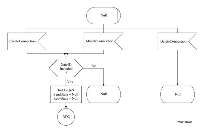
Figure B.1/J.162 – NCS/D-QoS state diagram (sheet 1 of 2)
