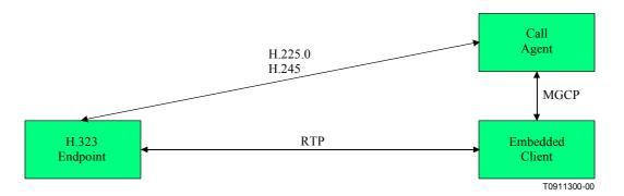
In the MGCP model, the gateways focus on the audio signal translation function, while the Call Agent handles the signalling and call processing functions. As a consequence, the Call Agent implements the "signalling" layers of the H.323 standard, and presents itself as an "H.323 Gatekeeper" or as one or more "H.323 Endpoints" to the H.323 systems. The H.225.0 call signalling and H.245 media signalling is therefore routed to the Call Agent.
