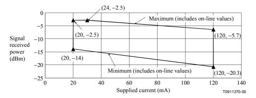
NOTE – The signal received power where the supplied current is less than 20 mA should be from -14 dBm to -2.5 dBm. When the supplied current is more than 120 mA, it should be from -20.3 dBm to -5.7 dBm.
