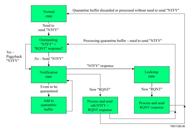
Call Agents SHOULD provide the response to a successful Notify message and the new NotificationRequest in the same datagram using the piggybacking mechanism<sup>24</sup>.
