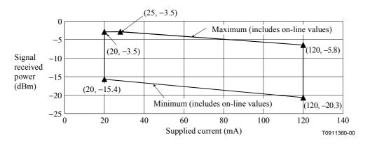
NOTE – The signal received power when the supplied current is less than 20 mA should be from -15.4 dBm to -3.5 dBm. When the supplied current is more than 120 mA, it should be from -20.3 dBm to -5.8 dBm.
