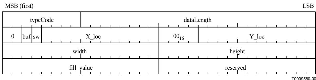
**Figure 15/J.151 – Fill region with constant subframe format**
