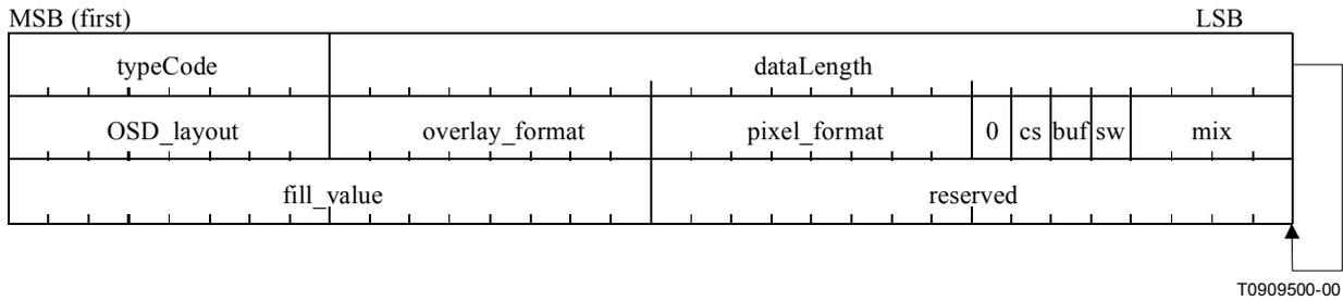
**Figure 7/J.151 – Set OSD pixel format subframe, 16-bit colour depth**
