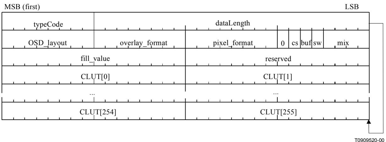
**Figure 9/J.151 – Set OSD pixel format subframe, 8-bit colour depth**
