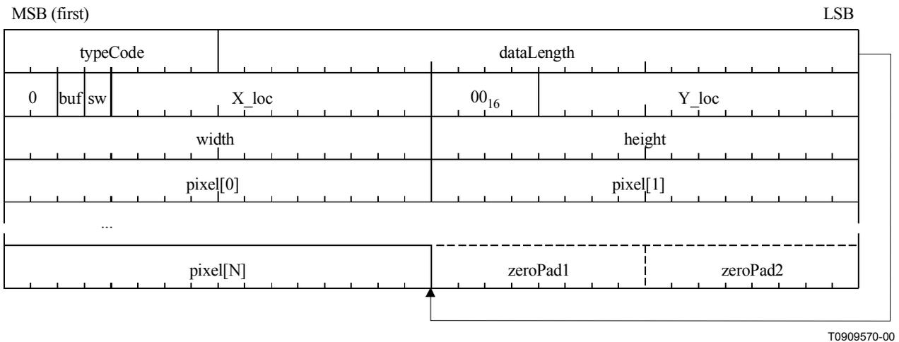
Figure 14/J.151 – Uncompressed 16-bit data subframe format
