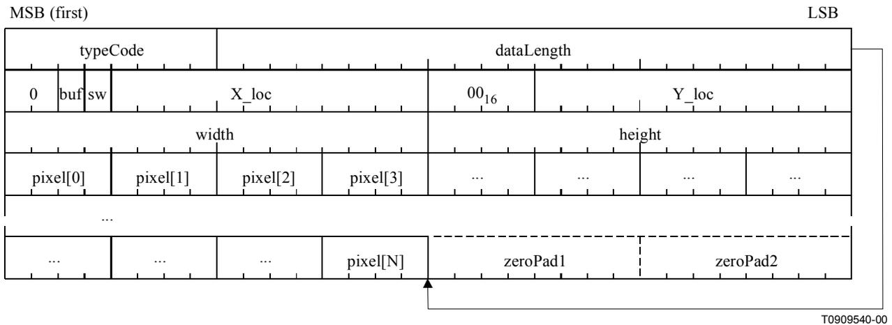
**Figure 11/J.151 – 4-bit OSD data subframe format**
