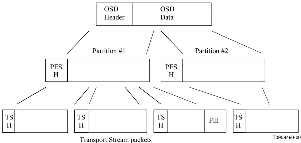
**Figure 6/J.151 – OSD data packet illustration**
