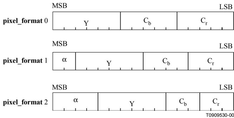
**Figure 10/J.151 – Pixel format bit fields**
