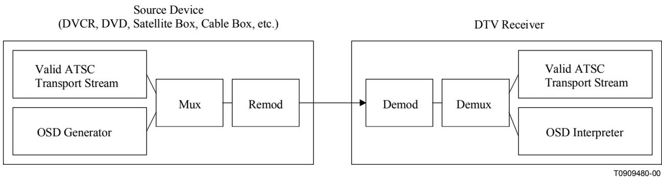
**Figure 5/J.151 – Typical OSD system illustration**
