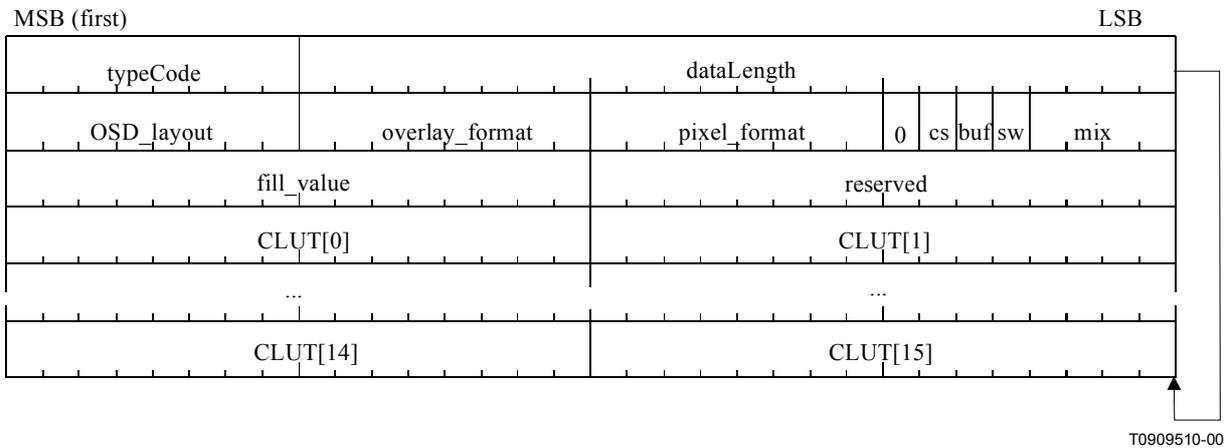
**Figure 8/J.151 – Set OSD pixel format subframe, 4-bit colour depth**
