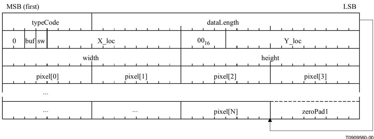
**Figure 13/J.151 – 8-bit OSD data subframe format**
