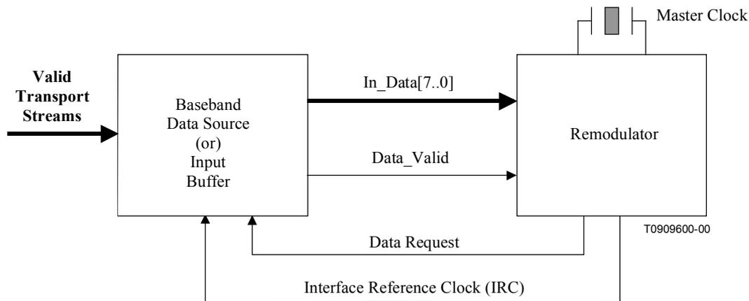
**Figure 17/J.151 – Remodulator system**
