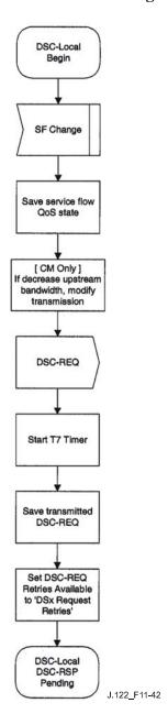
Figure 11-42 – DSC – Locally-initiated transaction begin state flow diagram
