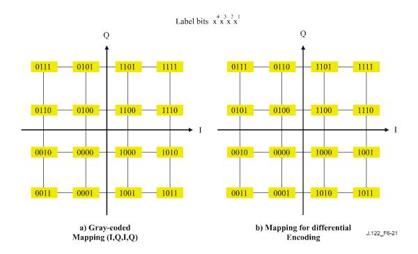
Figure 6-21 – 16QAM symbol mapping
