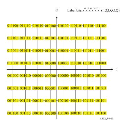
Figure 6-23 – 64QAM symbol mapping
