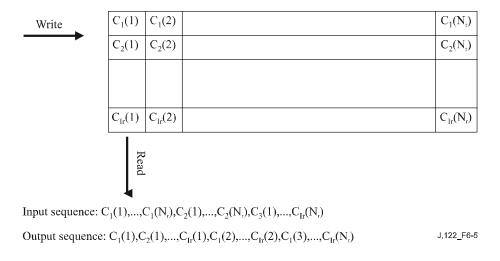
Figure 6-5 – Byte interleaver operation
