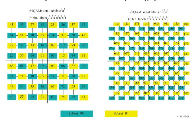
Figure 6-26 – 64QAM and 128QAM TCM symbol mapping
