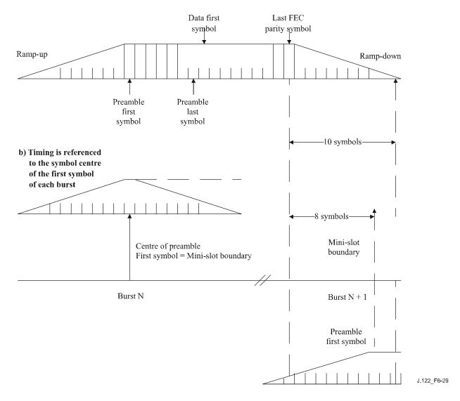
NOTE - Ramp-down of one burst can overlap ramp-up of following burst even with one transmitter assigned both bursts.
