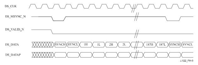
Figure H.3 – Downstream data signal protocol for J.83 Annex B operation
