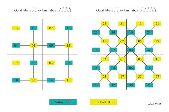
Figure 6-25 – 16QAM and 32QAM TCM symbol mapping
