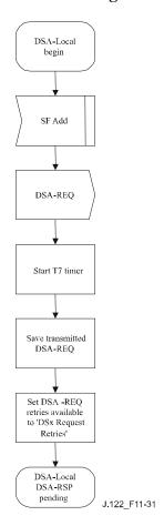
Figure 11-31 – DSA – Locally-initiated transaction begin state flow diagram
