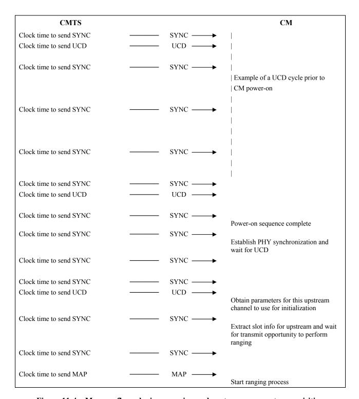
Figure 11-4 – Message flows during scanning and upstream parameter acquisition
