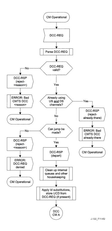
Figure 11-62 – Dynamically changing channels: CM view, part 1
