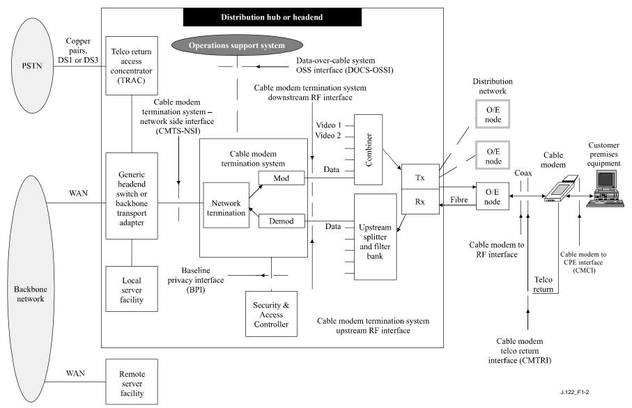
Figure 1-2 – Data-over-cable reference architecture
