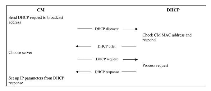
Figure 11-10 – Establishing IP connectivity
