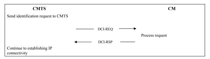
Figure 11-9 – Device class identification
