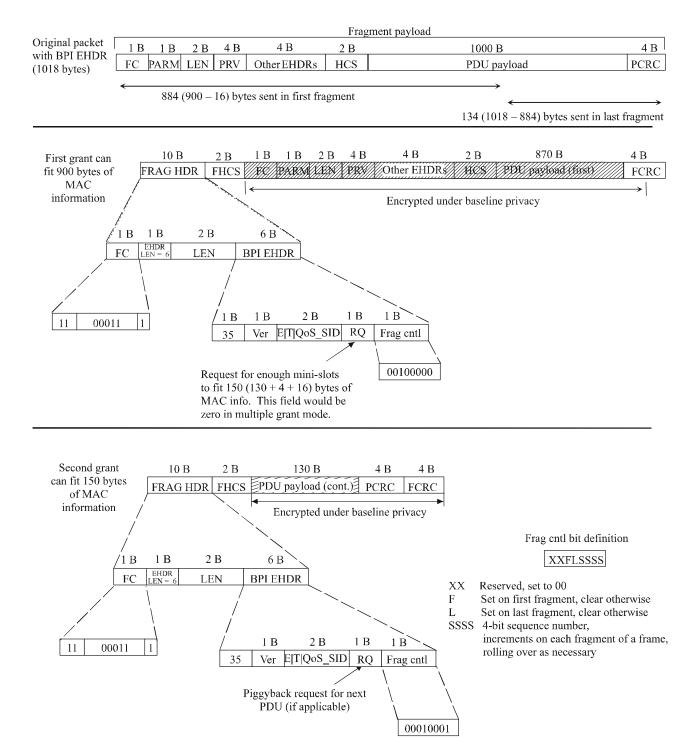
Figure 10-9 – Example of fragmenting a single packet
