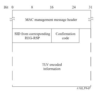
Figure 8-27 – Registration acknowledgment
