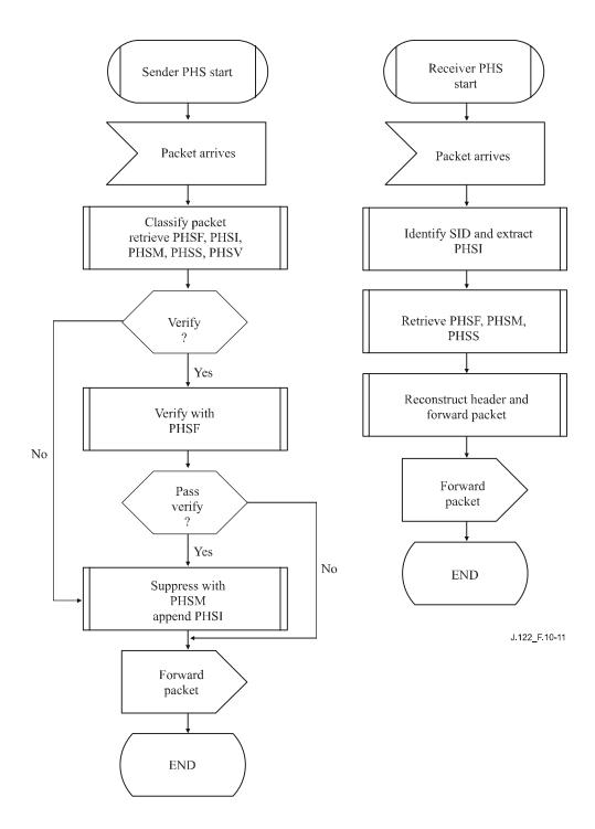
Figure 10-11 – Payload header suppression operation
