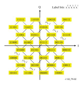
Figure 6-22 – 32QAM symbol mapping
