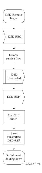
Figure 11-56 – DSD – Remotely-initiated transaction begin state flow diagram
