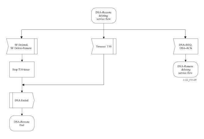
Figure 11-39 – DSA – Remotely-initiated transaction deleting service state flow diagram
