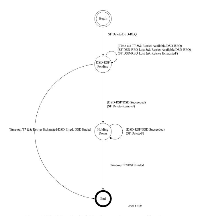
Figure 11-27 - DSD - Locally-initiated transaction state transition diagram
