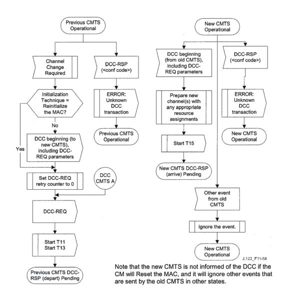
Figure 11-58 – Dynamically changing channels: CMTS view, part 1
