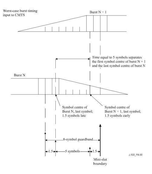
Figure 6-30 – Worst-case TDMA burst timing
