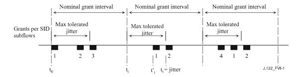
Figure VI.1 – Example jitter with multiple grants per SID
