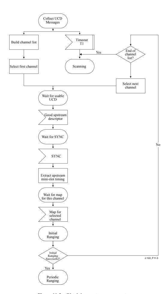
Figure 11-3 – Obtaining upstream parameters
