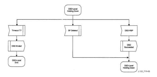
Figure 11-55 – DSD – Locally-initiated transaction holding down state flow diagram
