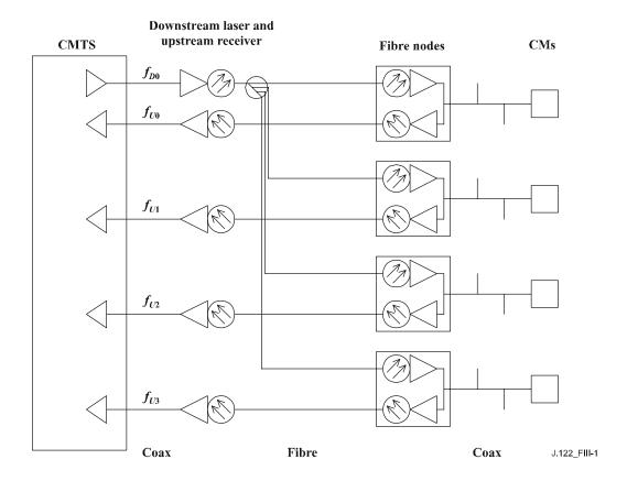
Figure III.1 - Single downstream and single upstream channels per CM
