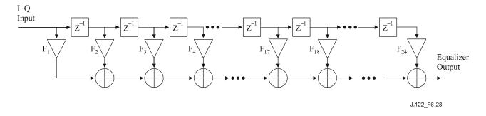
Figure 6-28 – Transmit pre-equalizer structure
