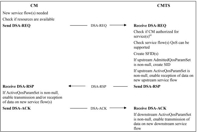
Authorization can happen prior to the DSA-REQ being received by the CMTS. The details of CMTS signalling to anticipate a DSA-REQ are beyond the scope of this Recommendation.
