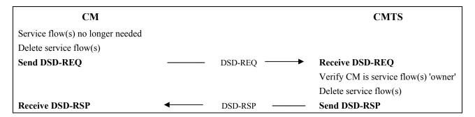
Figure 11-51 – Dynamic service deletion initiated from CM
