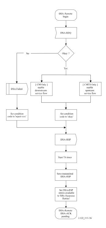
$Figure\ 11\text{--}36-DSA-Remotely-initiated\ transaction\ begin\ state\ flow\ diagram$
