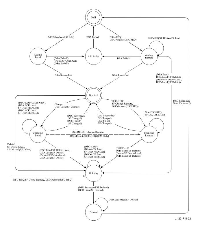
Figure 11-22 – Dynamic service flow state transition diagram
