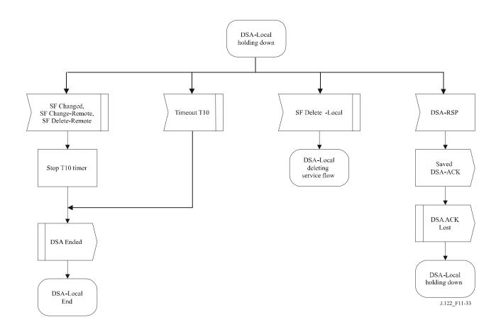
Figure 11-33 – DSA – Locally-initiated transaction holding state flow diagram
