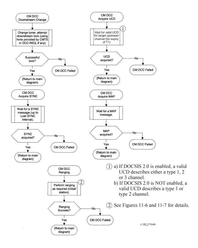
Figure 11-64 – Dynamically changing channels – CM view, part 3
