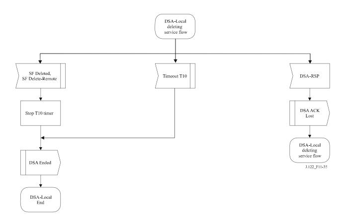
$Figure\ 11\text{-}35-DSA-Locally-initiated\ transaction\ deleting\ service\ flow\ state\ flow\ diagram$
