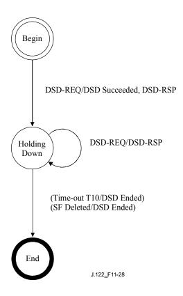
Figure 11-28 – Dynamic deletion (DSD) – Remotely-initiated transaction state transition diagram
