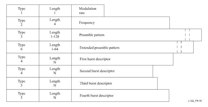
Figure 8-18 – Example of UCD encoded TLV data
