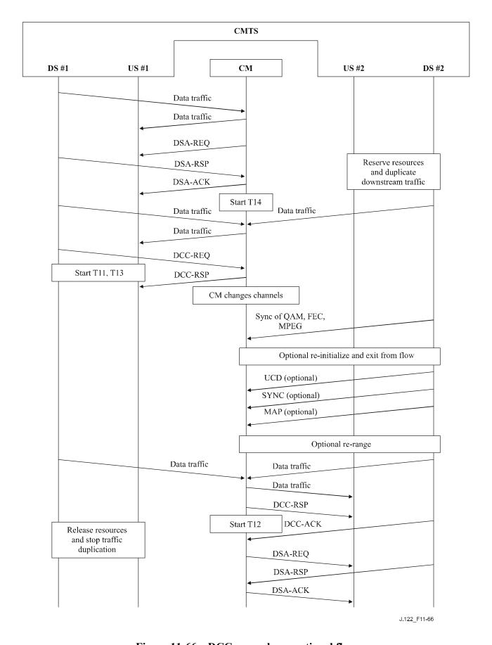
Figure 11-66 – DCC example operational flow
