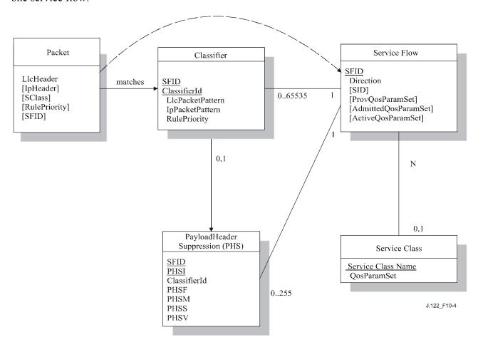
Figure 10-4 – Theory of operation object model
