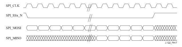
Figure H.7 – SPI bus transaction
