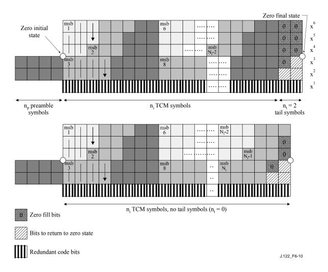
Figure 6-10 – Example byte to bit assignment for 64QAM
