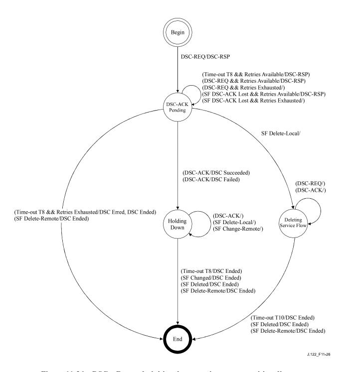
Figure 11-26 - DSC - Remotely-initiated transaction state transition diagram
