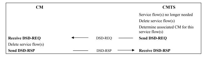
Figure 11-52 – Dynamic service deletion initiated from CMTS
