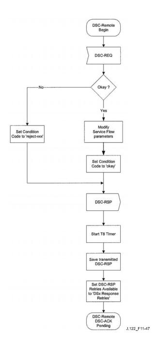
$Figure\ 11\text{-}47-DSC-Remotely-initiated\ transaction\ begin\ state\ flow\ diagram$
