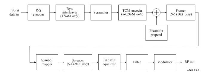
Figure 6-1 – Upstream signal-processing sequence
