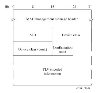
Figure 8-42 – Device class identification response
