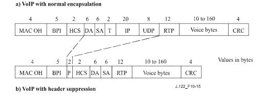
Figure 10-15 – Downstream payload header suppression example
