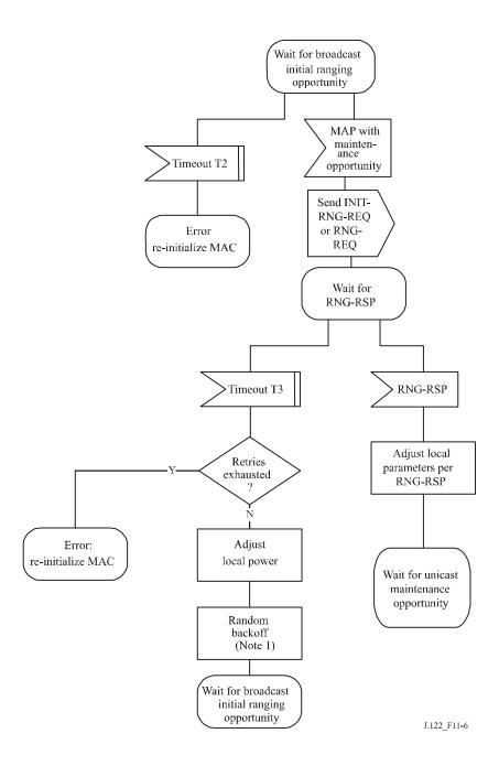
NOTE 1 – Timeout T3 may occur because the RNG-REQs from multiple modems collided. To avoid these modems repeating the loop in lockstep, a random backoff is required. This is a backoff over the ranging window specified in the MAP. T3 timeouts can also occur during multi-channel operation. On a system with multiple upstream channels, the CM MUST attempt initial ranging on every suitable upstream channel before moving to the next available downstream channel.
