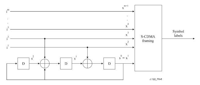
Figure 6-8 – Convolutional encoder
