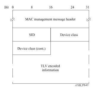
Figure 8-41 – Device class identification request
