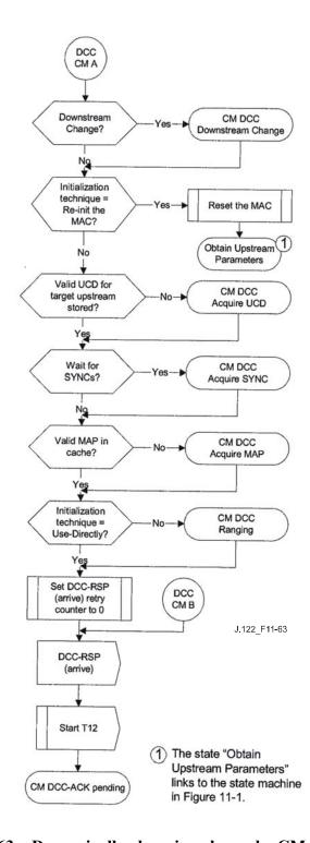
Figure 11-63 – Dynamically changing channels: CM view, part 2
