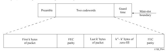
Figure 6-4 – Example frame structures with flexible burst length mode
