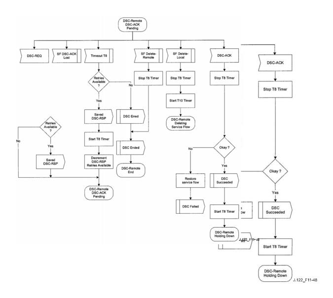
Figure 11-48 – DSC – Remotely-initiated transaction DSC-ACK pending state flow diagram
