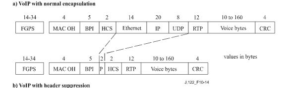
Figure 10-14 – Upstream payload header suppression example
