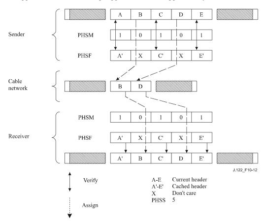
Figure 10-12 – Payload header suppression with masking
