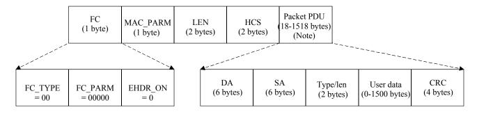
NOTE – Frame size is limited to 1518 bytes in the absence of VLAN tagging. Cooperating devices which implement IEE 802.1Q VLAN tagging MAY use a frame size up to 1522 bytes.
