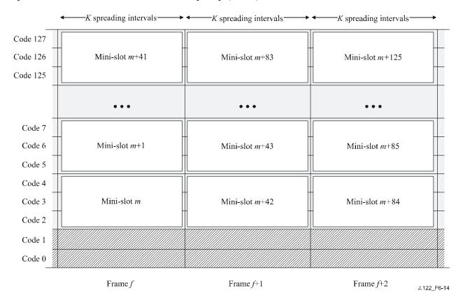
Figure 6-14 – Mini-slot mapping with three codes per mini-slot, 126 active codes
