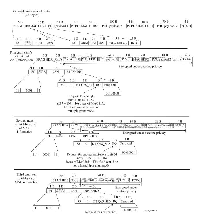
Figure 10-10 – Fragmented concatenated packet example
