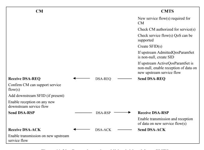
Figure 11-30 – Dynamic service addition initiated from CMTS
