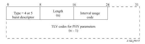
Figure 8-17 – Top-level encoding for burst descriptors
