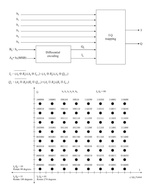
Figure J.6-6 – 256QAM signal constellation diagram and phase shift rule (I = 12)
