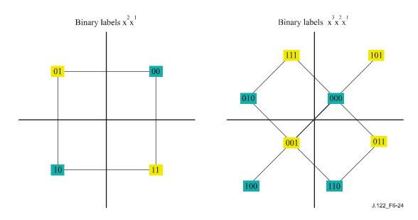
Figure 6-24 - QPSK and 8QAM TCM symbol mapping
