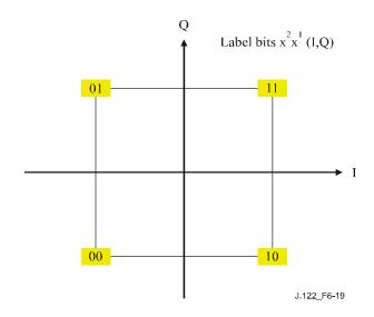
Figure 6-19 – QPSK Gray-coded and differential symbol mapping
