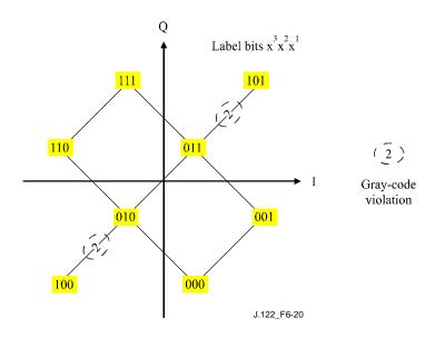
Figure 6-20 – 8QAM symbol mapping
