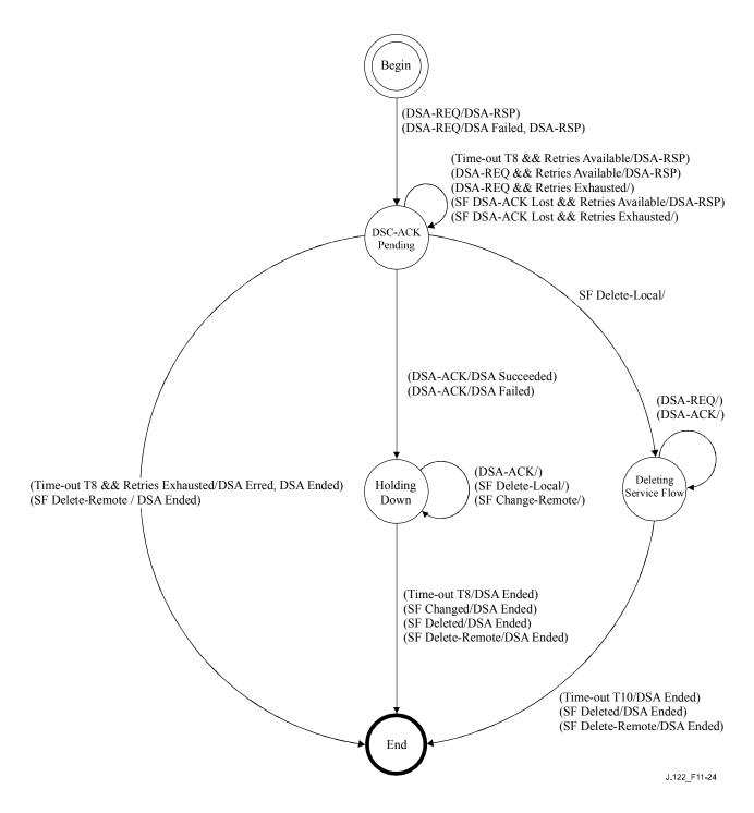
Figure 11-24 - DSA - Remotely-initiated transaction state transition diagram
