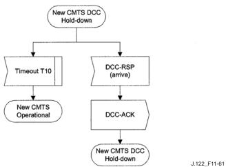
Figure 11-61 – Dynamically changing channels: CMTS view, part 4
