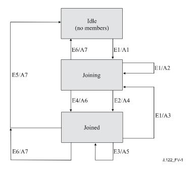
Figure V.1 – IGMP support – CM passive mode
