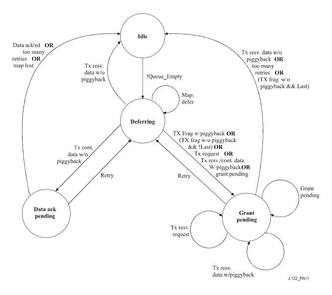
Figure IV.1 - Transmission and deference state transition diagram
