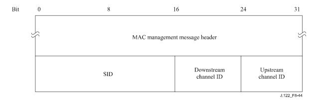
Figure 8-44 – Packet PDU following the timing header
