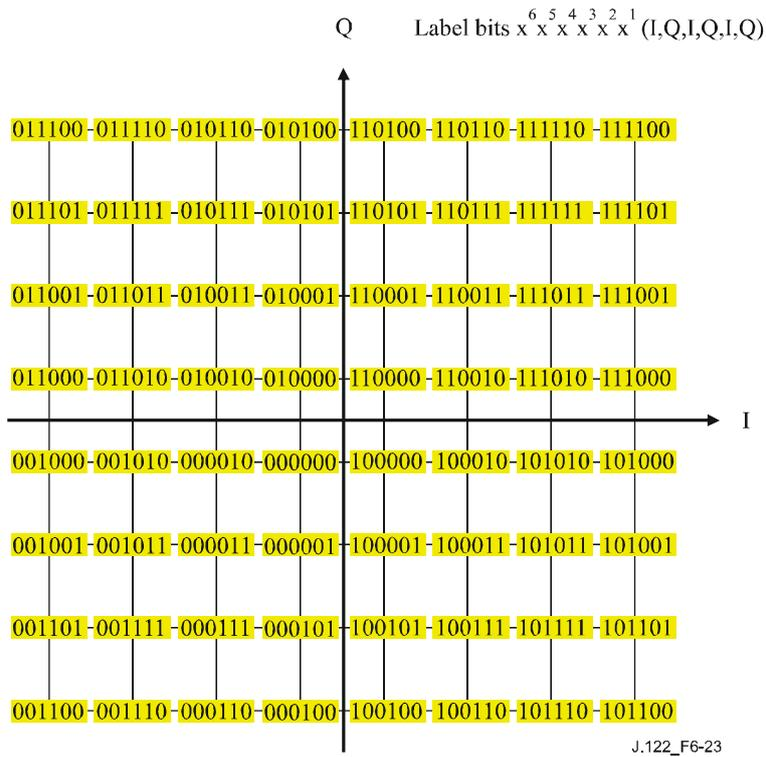
**Figure 6-23 – 64QAM symbol mapping**
