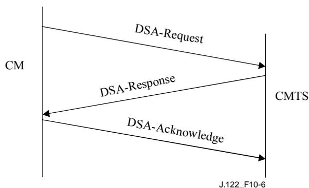
**Figure 10-6 – Dynamic service addition message flow – CM-initiated**
