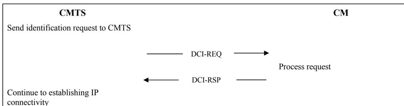
**Figure 11-9 – Device class identification**
