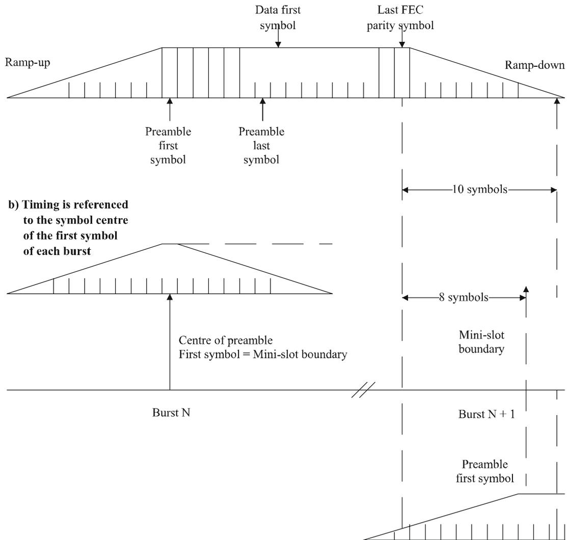
NOTE - Ramp-down of one burst can overlap ramp-up of following burst even with one transmitter assigned both bursts.
