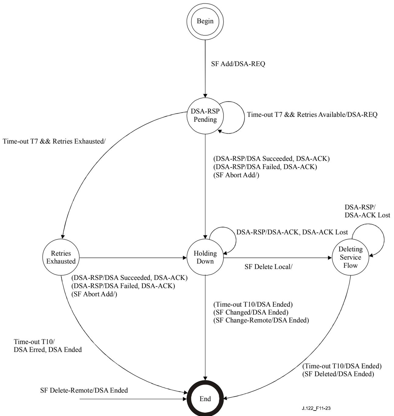
**Figure 11-23 – DSA – Locally-initiated transaction state transition diagram**
