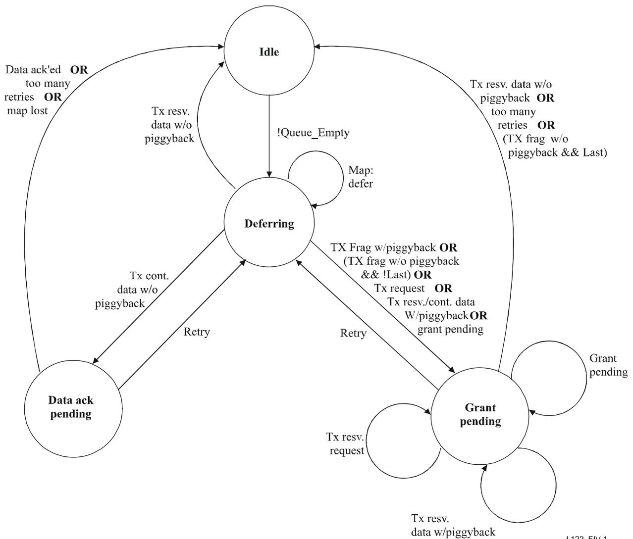
**Figure IV.1 – Transmission and deference state transition diagram**
