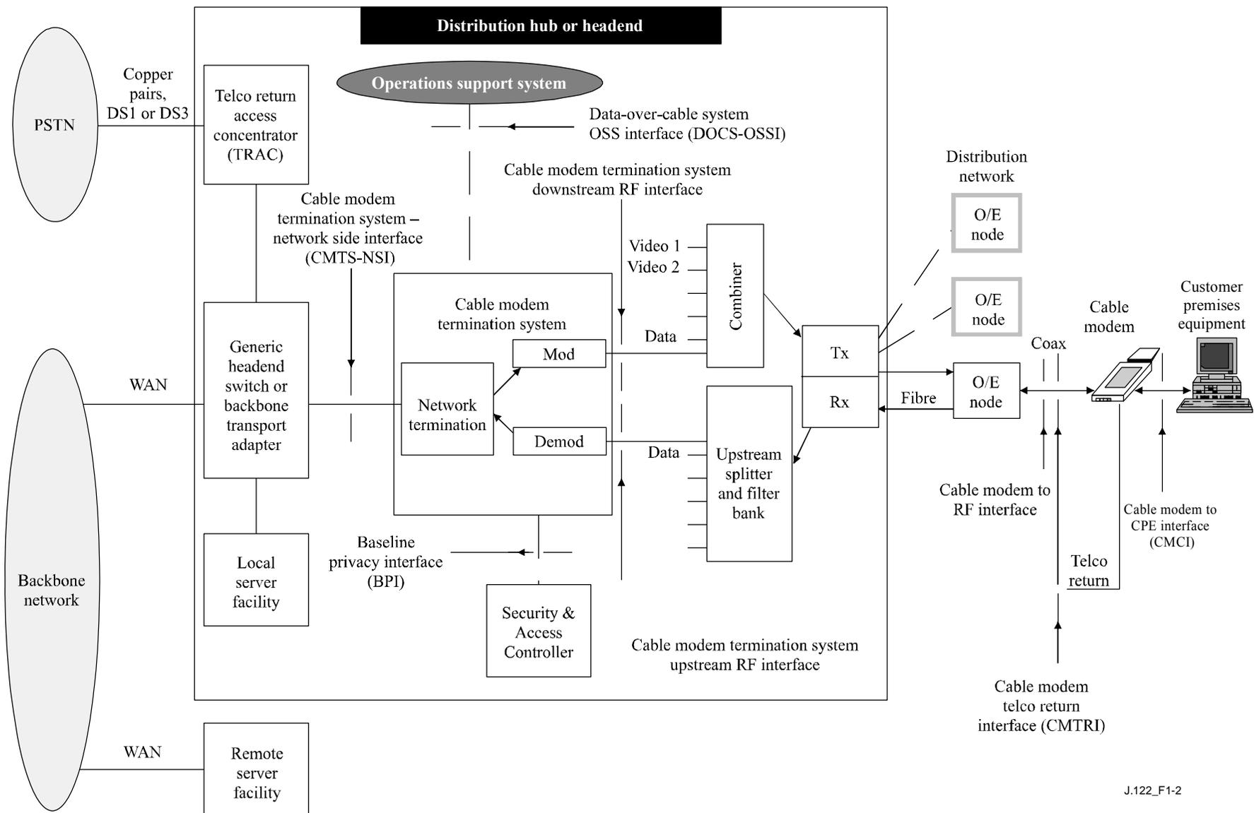
**Figure 1-2 – Data-over-cable reference architecture**
