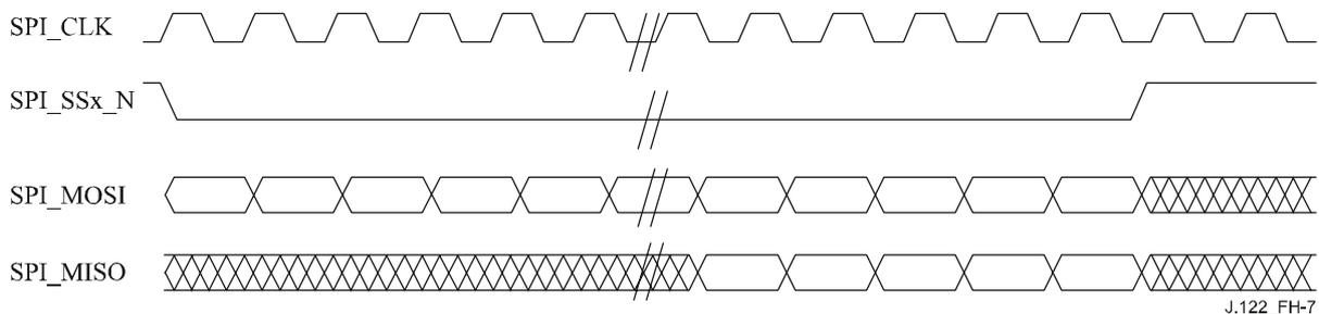
**Figure H.7 – SPI bus transaction**
