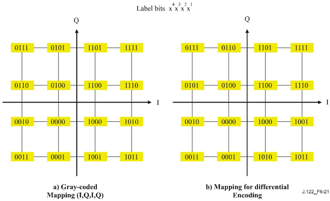
**Figure 6-21 – 16QAM symbol mapping**
