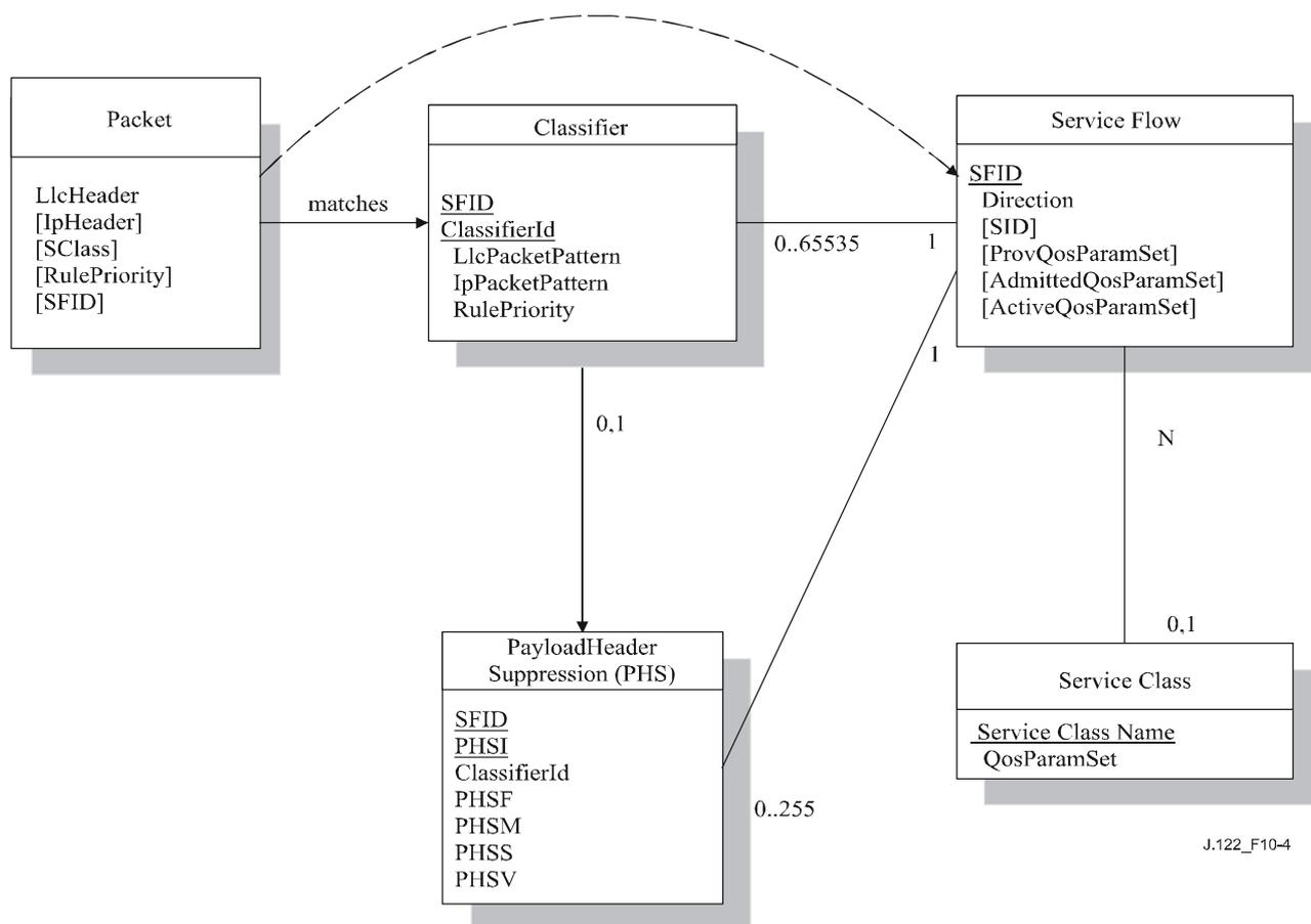
Figure 10-4 – Theory of operation object model
