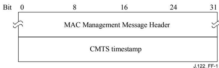
**Figure F.1 – Format of packet PDU following the timing header**
