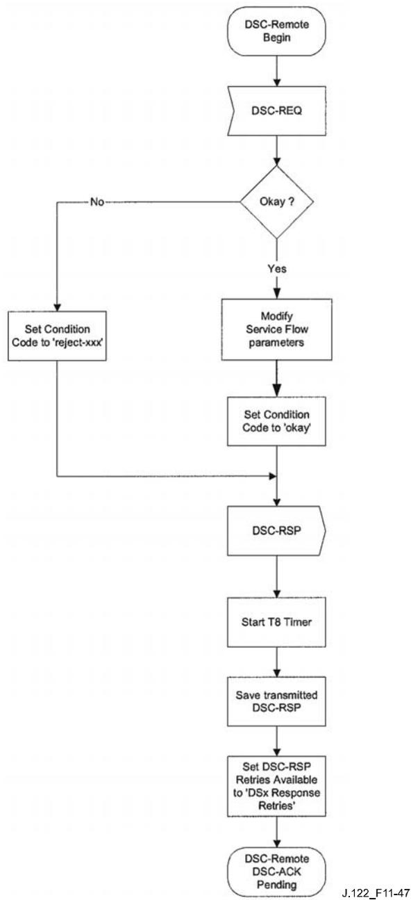
**Figure 11-47 – DSC – Remotely-initiated transaction begin state flow diagram**
