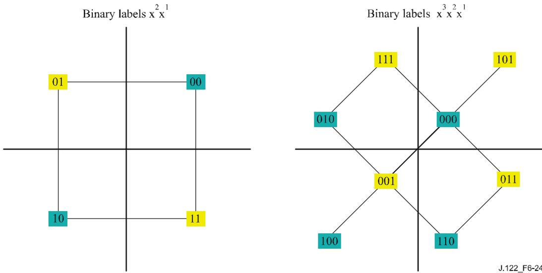
**Figure 6-24 – QPSK and 8QAM TCM symbol mapping**
