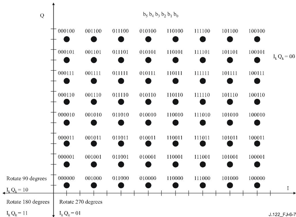
**Figure J.6-7 – 256QAM signal constellation diagram and phase shift rule (I = 34 or 204)**
