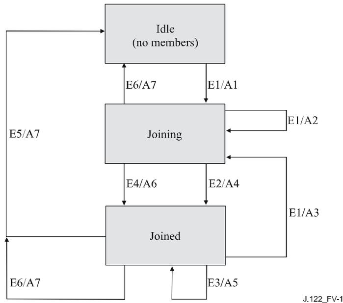
**Figure V.1 – IGMP support – CM passive mode**
