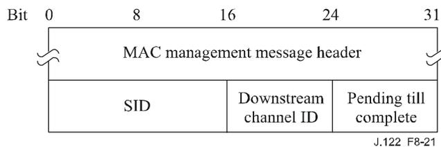
**Figure 8-21 – Packet PDU following the timing header**
