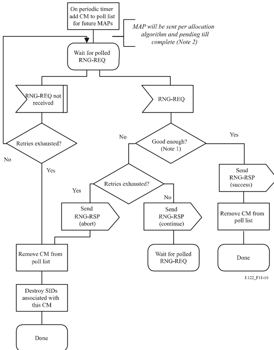
NOTE 1 – "Good enough" means ranging request is within the tolerance limits of the CMTS for power and transmit equalization (if supported).
