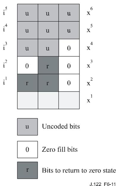
**Figure 6-11 – Example of return-to-zero bits followed by "0"**
