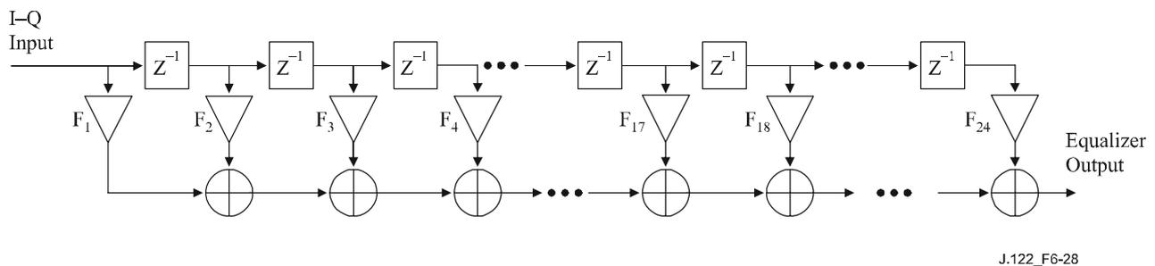
**Figure 6-28 – Transmit pre-equalizer structure**
