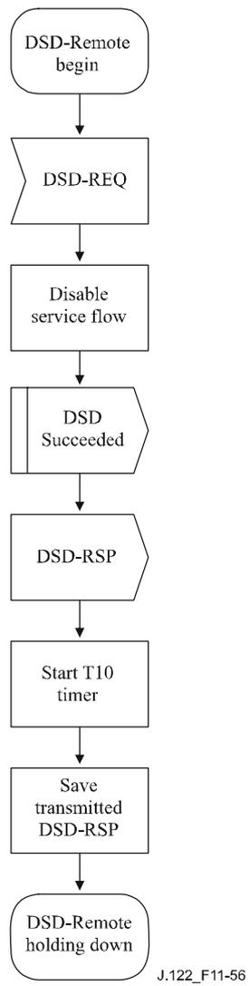
**Figure 11-56 – DSD – Remotely-initiated transaction begin state flow diagram**
