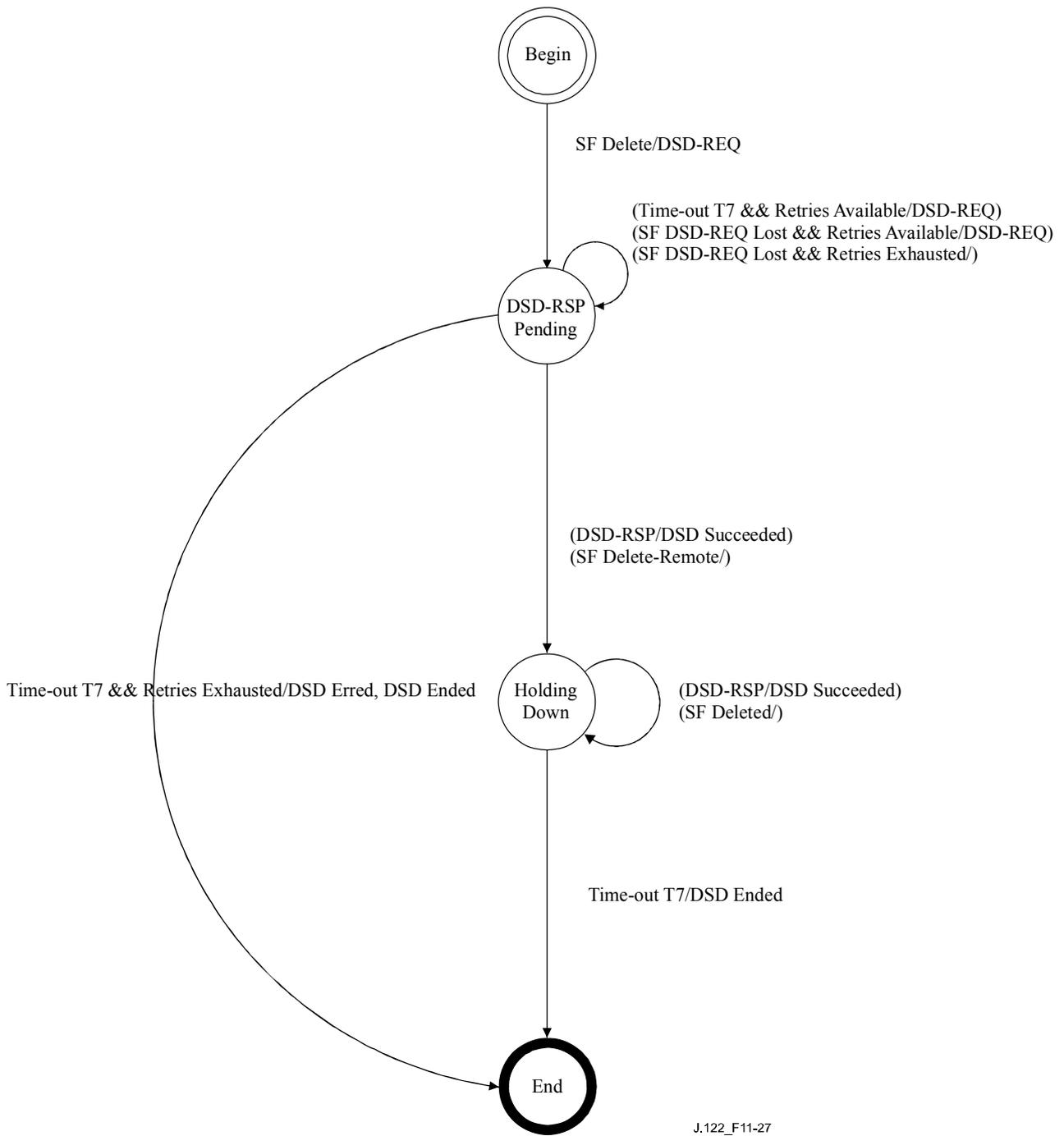
**Figure 11-27 – DSD – Locally-initiated transaction state transition diagram**
