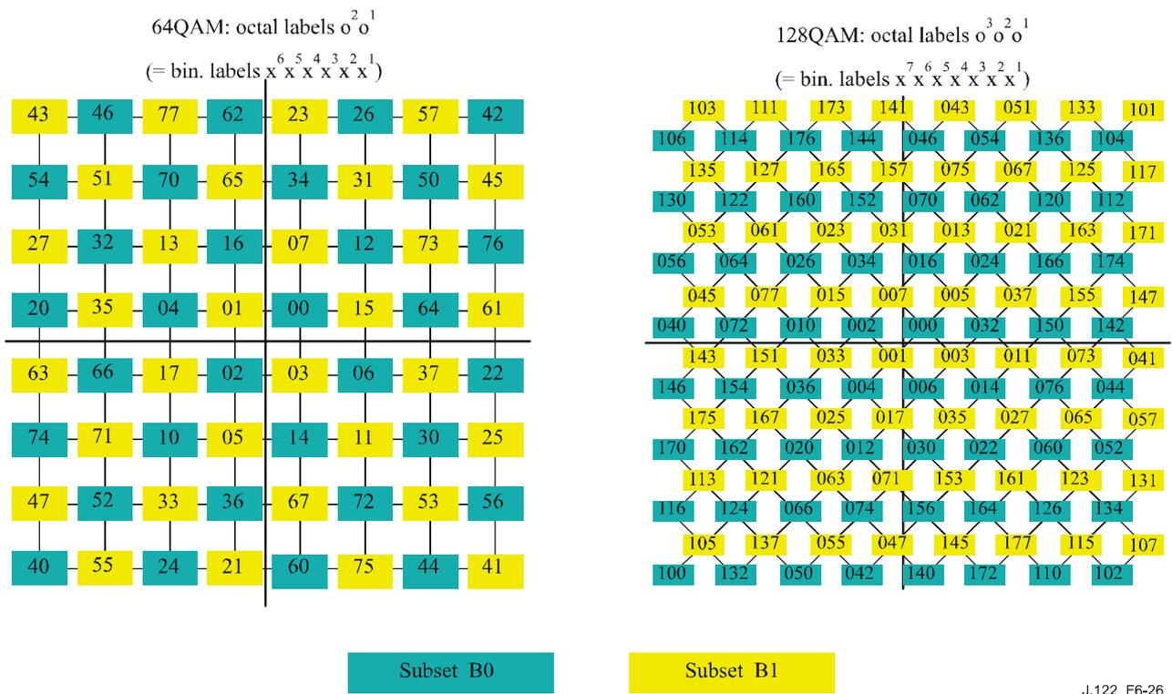
Figure 6-26 – 64QAM and 128QAM TCM symbol mapping
