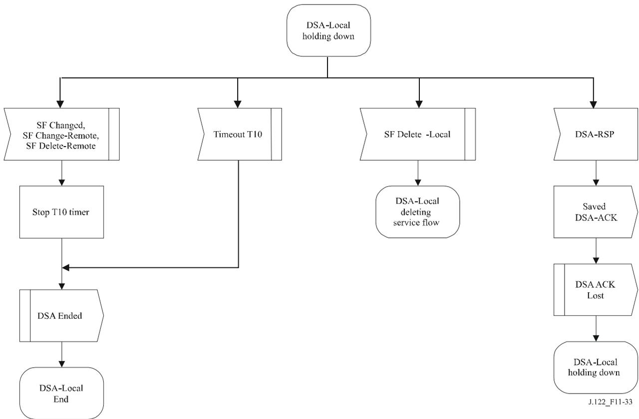
**Figure 11-33 – DSA – Locally-initiated transaction holding state flow diagram**
