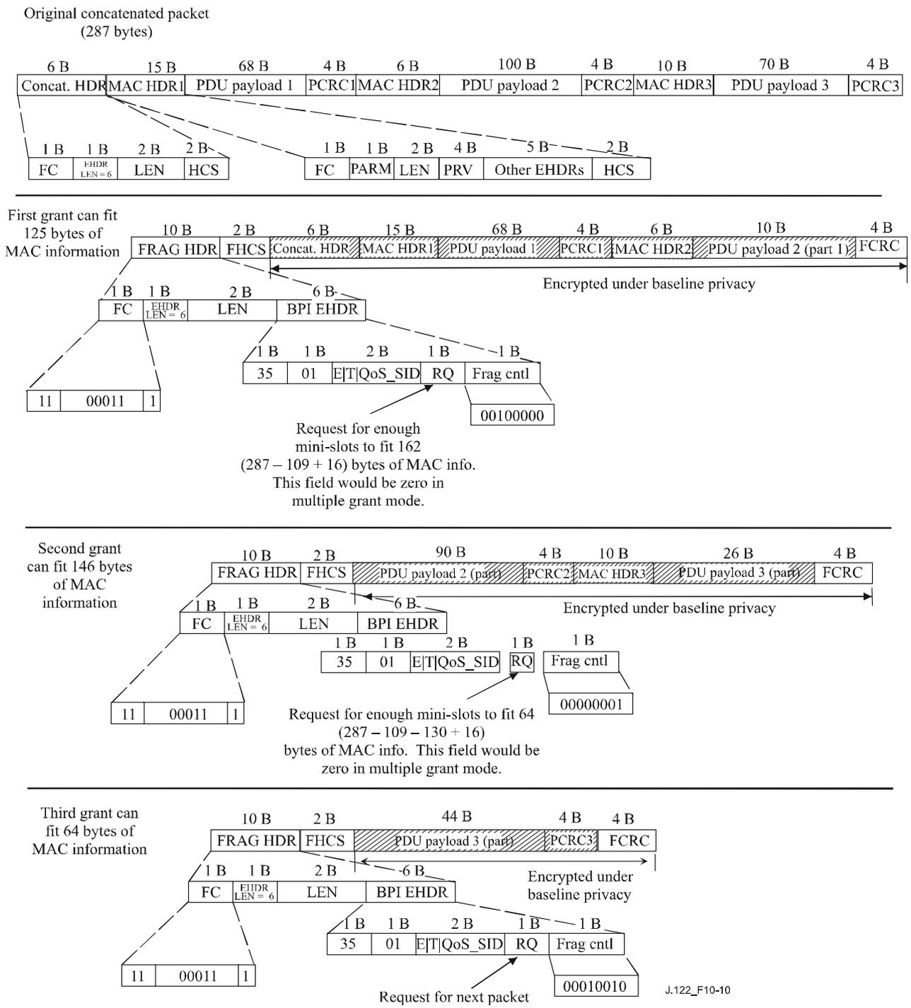
Figure 10-10 – Fragmented concatenated packet example
