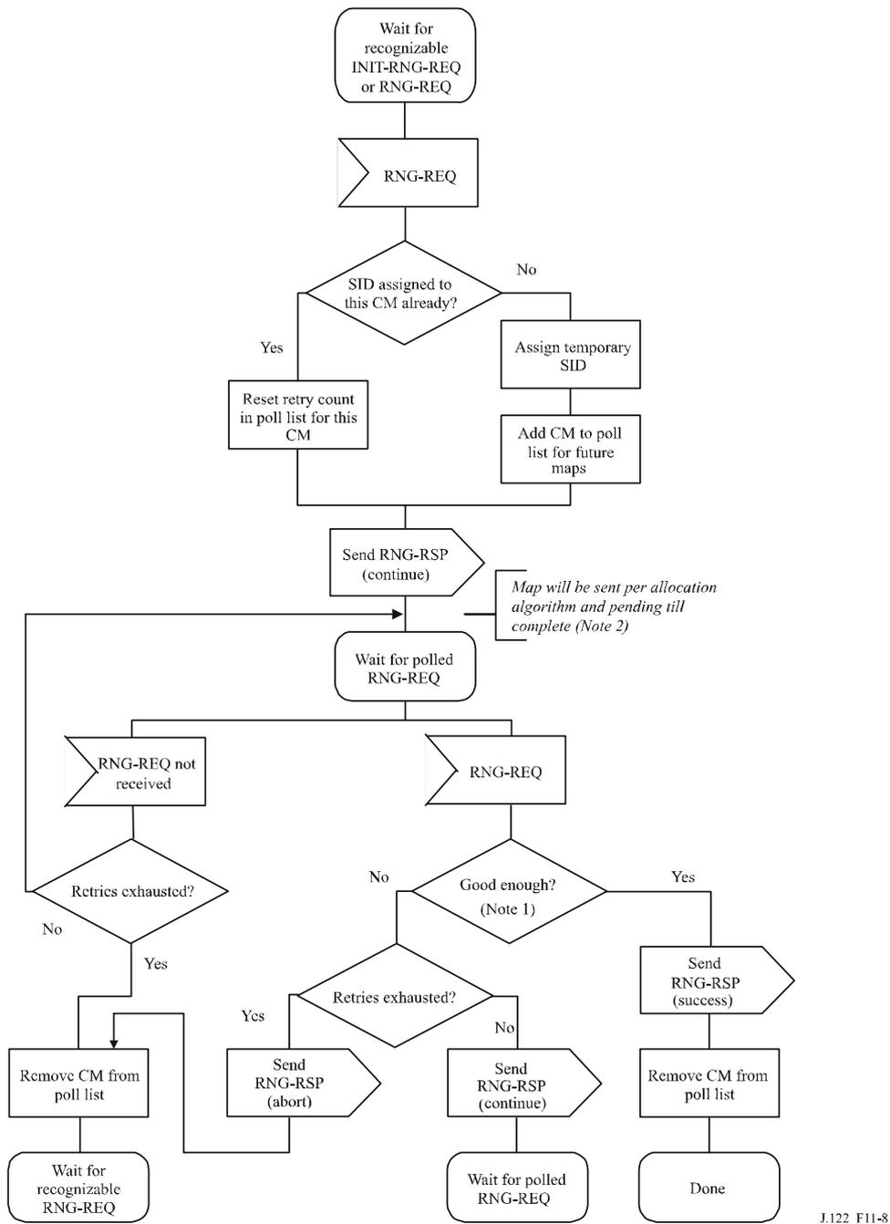
NOTE 1 – "Good enough" means ranging is within the tolerable limits of the CMTS.
