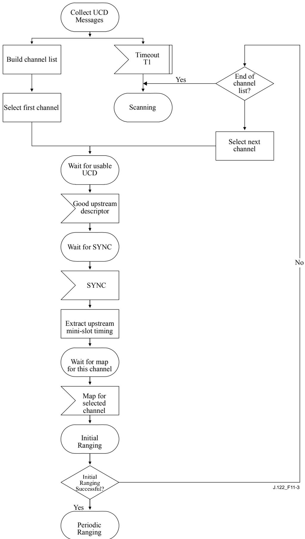
**Figure 11-3 – Obtaining upstream parameters**
