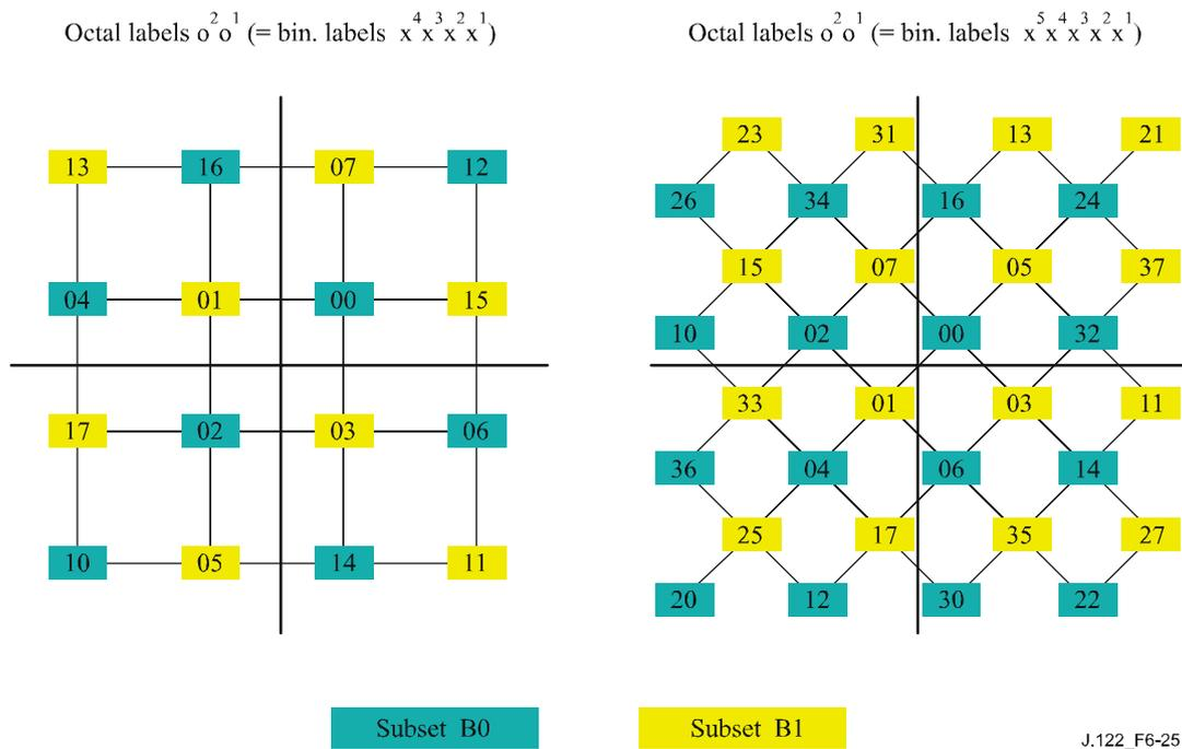
Figure 6-25 – 16QAM and 32QAM TCM symbol mapping
