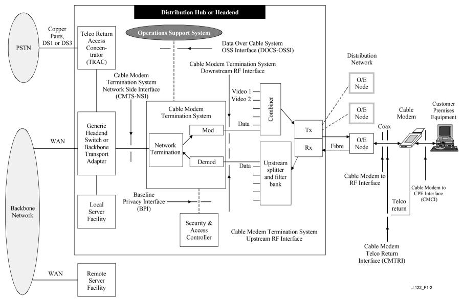
Figure 1-2 – Data-over-cable reference architecture
