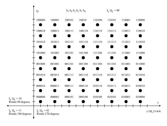
Figure J.6-6/J.122 - 256QAM signal constellation diagram and phase shift rule (I = 12)
