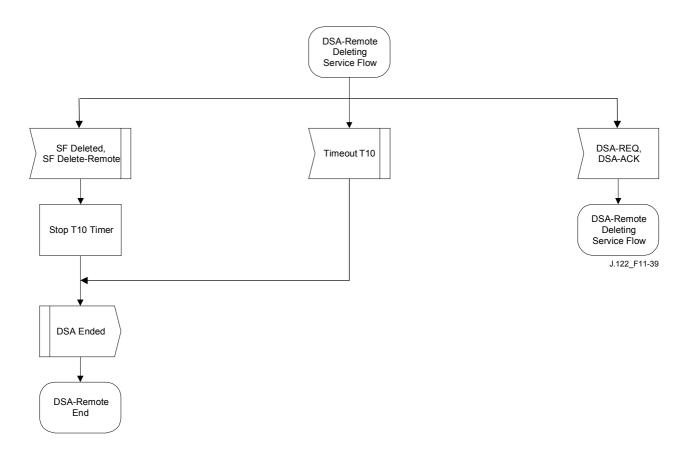
Figure 11-39/J.122 – DSA – Remotely initiated Transaction Deleting Service State Flow Diagram
