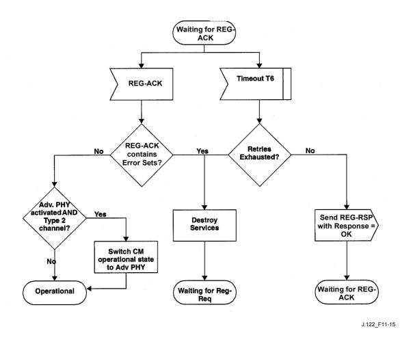
Figure 11-15/J.122 – Registration Acknowledgment – CMTS
