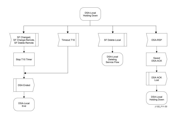
Figure 11-33/J.122 – DSA – Locally initiated Transaction Holding State Flow Diagram
