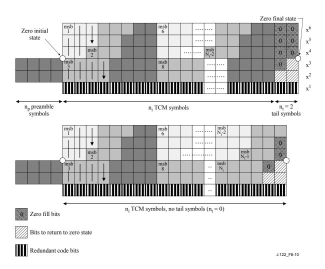
Figure 6-10/J.122 – Example byte to bit assignment for 64QAM
