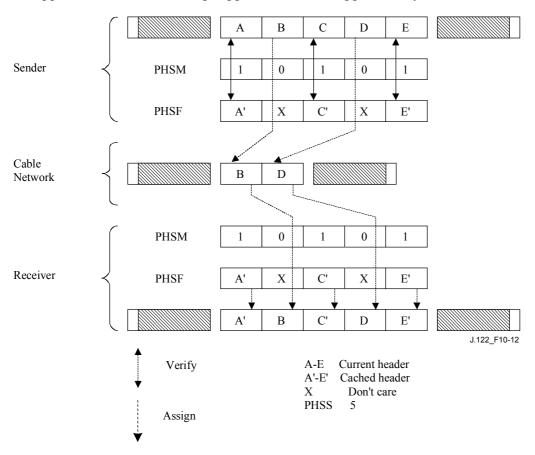
Figure 10-12/J.122 – Payload Header Suppression with Masking
