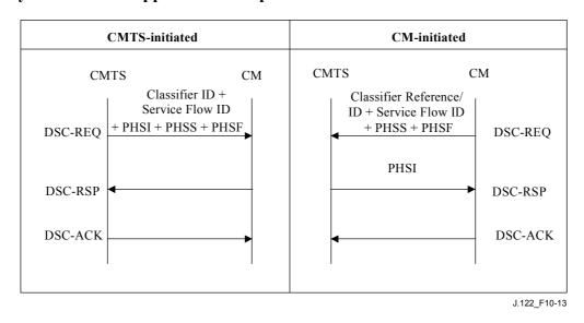
Figure 10-13/J.122 – Payload Header Suppression signalling example
