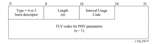
Figure 8-17/J.122 – Top-level encoding for burst descriptors
