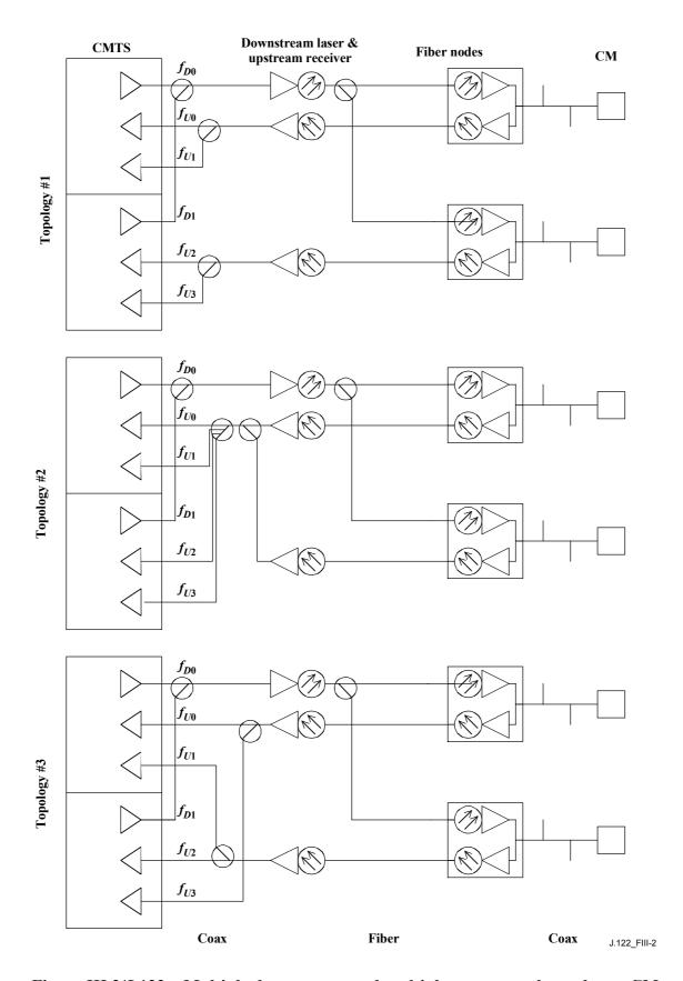
Figure III.2/J.122 – Multiple downstream and multiple upstream channels per CM
