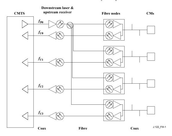
Figure III.1/J.122 – Single downstream and single upstream channels per CM
