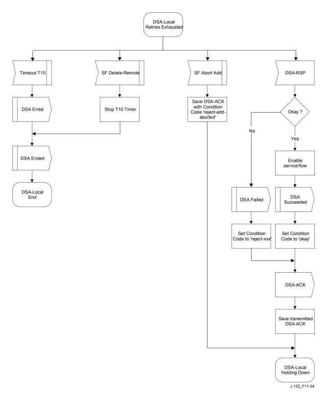
Figure 11-34/J.122 – DSA – Locally initiated Transaction Retries Exhausted State Flow Diagram
