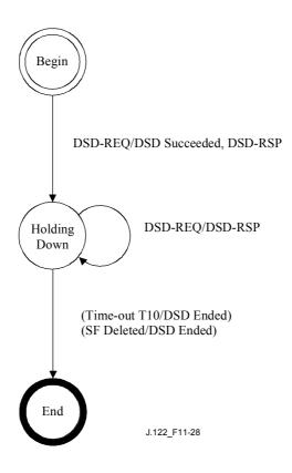
Figure 11-28/J.122 – Dynamic Deletion (DSD) – Remotely Initiated Transaction State Transition Diagram
