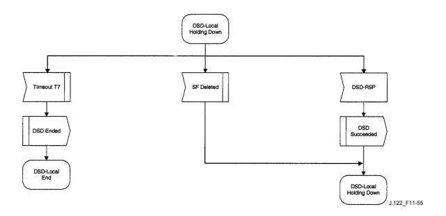
Figure 11-55/J.122 – DSD – Locally initiated Transaction Holding Down State Flow Diagram
