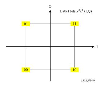
Figure 6-19/J.122 – QPSK Gray-coded and differential symbol mapping
