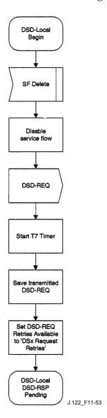
Figure 11-53/J.122 – DSD – Locally initiated Transaction Begin State Flow Diagram
