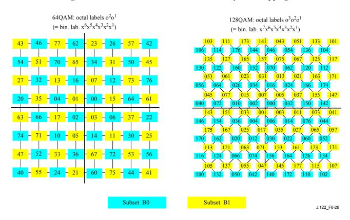
Figure 6-26/J.122 – 64QAM and 128QAM TCM symbol mapping
