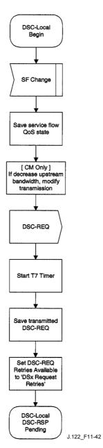
Figure 11-42/J.122 – DSC – Locally initiated Transaction DSC-RSP Pending State Flow Diagram
