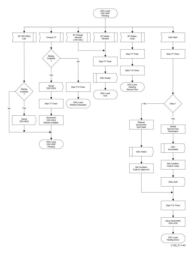
Figure 11-43/J.122 – DSC – Locally initiated Transaction DSC-RSP Pending State Flow Diagram
