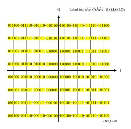
Figure 6-23/J.122 – 64QAM symbol mapping
