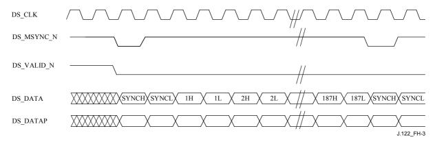
Figure H.3/J.122 – Downstream Data Signal Protocol For J.83 Annex B Operation
