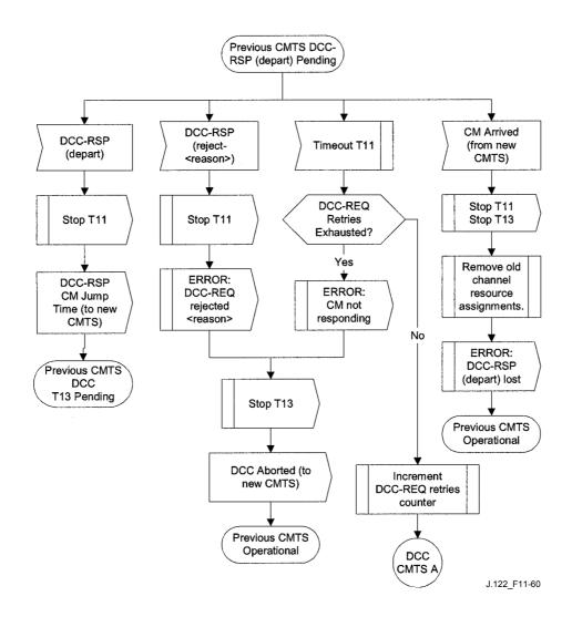
Figure 11-60/J.122 – Dynamically changing channels: CMTS view, Part 2
