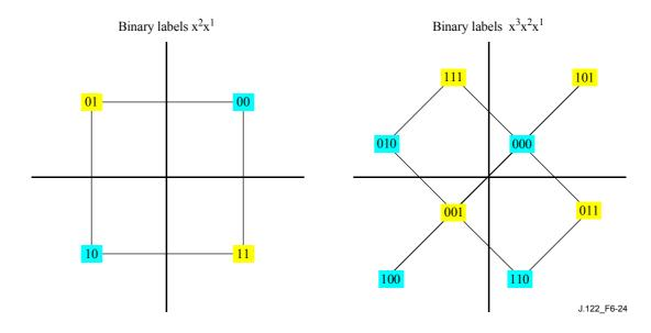
Figure 6-24/J.122 - QPSK and 8QAM TCM symbol mapping
