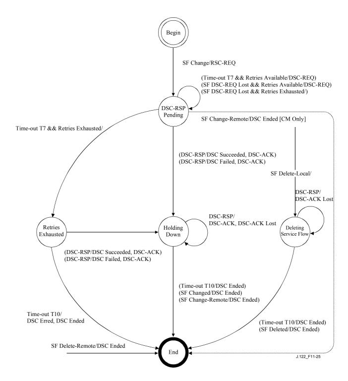
Figure 11-25/J.122 - DSC - Locally initiated Transaction State Transition Diagram
