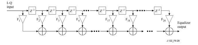
Figure 6-28/J.122 – Transmit pre-equalizer structure
