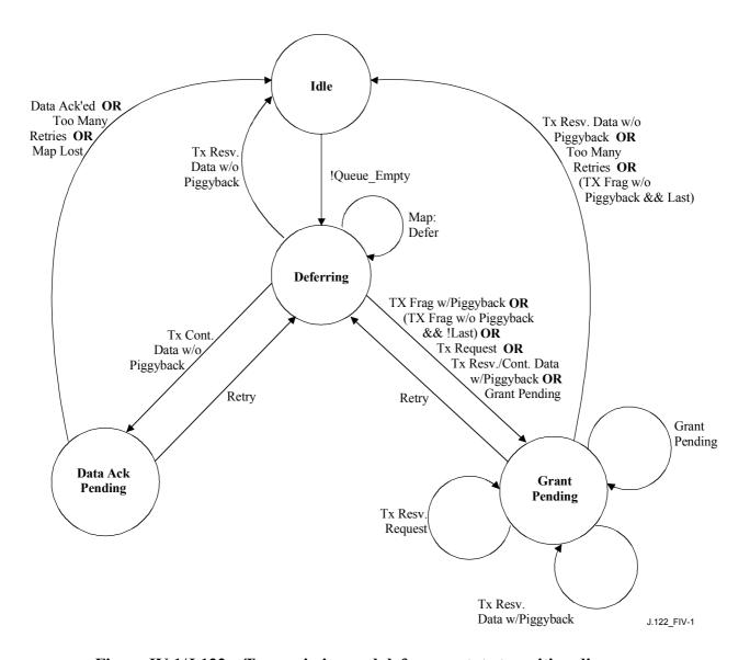
Figure IV.1/J.122 - Transmission and deference state transition diagram
