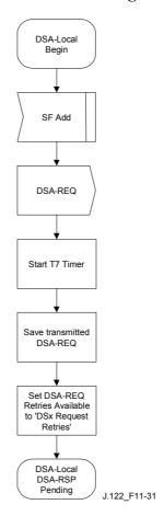
Figure 11-31/J.122 – DSA – Locally initiated Transaction Begin State Flow Diagram
