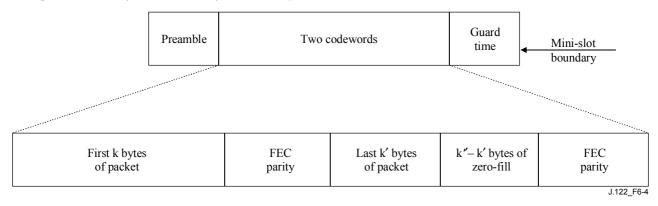
Figure 6-4/J.122 – Example frame structures with flexible burst length mode
