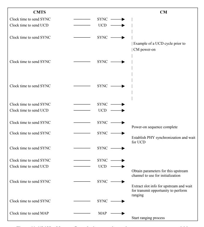
Figure 11-4/J.122 – Message flows during scanning and upstream parameter acquisition
