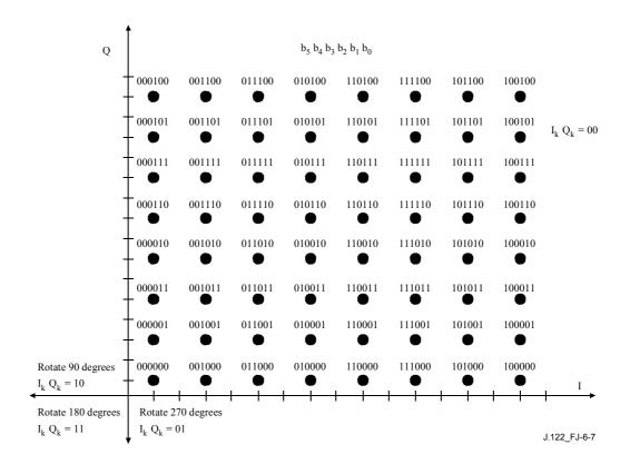
Figure J.6-7/J.122 – 256QAM Signal Constellation Diagram and Phase Shift Rule (I=34 or 204)
