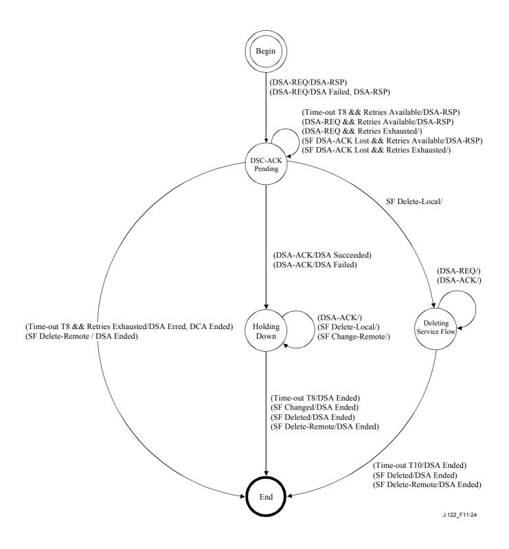
Figure 11-24/J.122 - DSA - Remotely initiated Transaction State Transition Diagram
