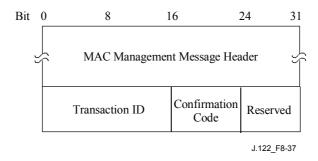
Figure 8-37/J.122 – Dynamic Service Deletion Response
