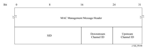
Figure 8-44/J.122 – Packet PDU following the Timing Header
