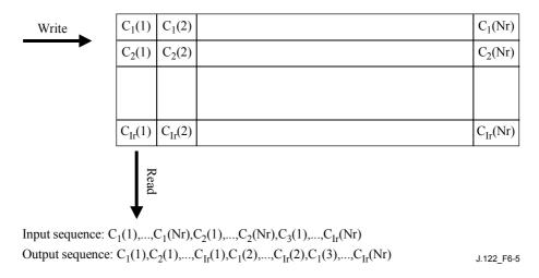
Figure 6-5/J.122 – Byte interleaver operation
