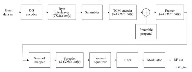
Figure 6-1/J.122 – Upstream signal-processing sequence
