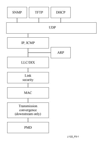
Figure 5-1/J.122 – Protocol stack on the RF interface
