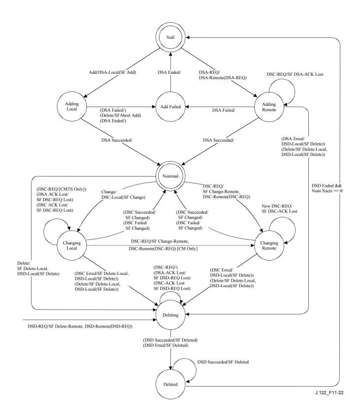
Figure 11-22/J.122 – Dynamic Service Flow State Transition Diagram
