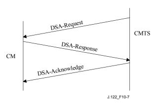
Figure 10-7/J.122 – Dynamic Service Addition message flow – CMTS-initiated
