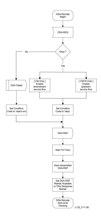
Figure 11-36/J.122 – DSA – Remotely initiated Transaction Begin State Flow Diagram
