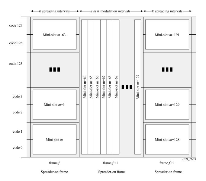
Figure 6-15/J.122 – S-CDMA and spreader-off intervals
