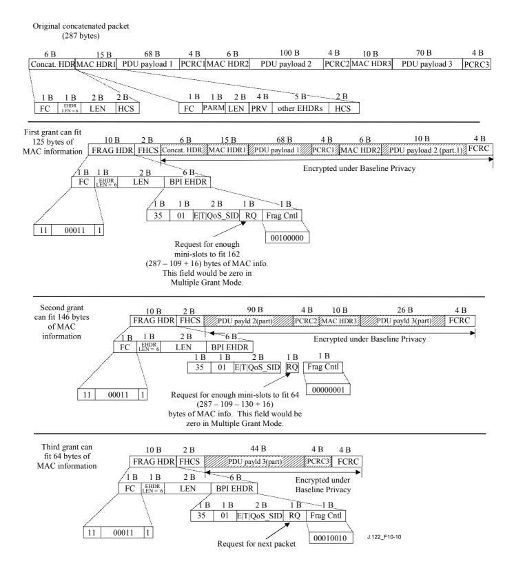
Figure 10-10/J.122 – Fragmented concatenated packet example
