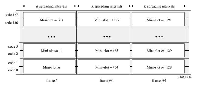
Figure 6-13/J.122 – Mini-slot mapping with two codes per mini-slot, 128 active codes
