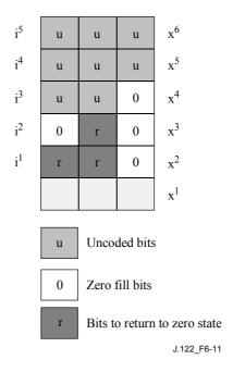
Figure 6-11/J.122 – Example of return to zero bits followed by "0"
