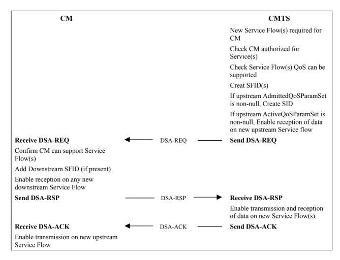
Figure 11-30/J.122 – Dynamic Service Addition initiated from CMTS
