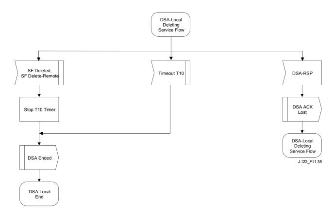
Figure 11-35/J.122 – DSA – Locally initiated Transaction Deleting Service Flow State Flow Diagram
