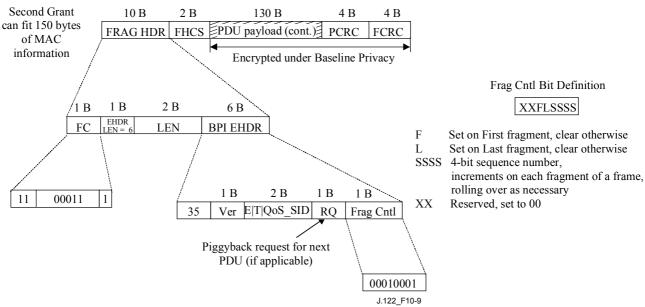
Figure 10-9/J.122 – Example of fragmenting a single packet
