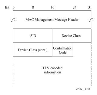
Figure 8-42/J.122 – Device Class Identification Response
