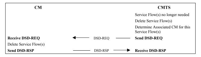
Figure 11-52/J.122 – Dynamic Service Deletion initiated from CMTS
