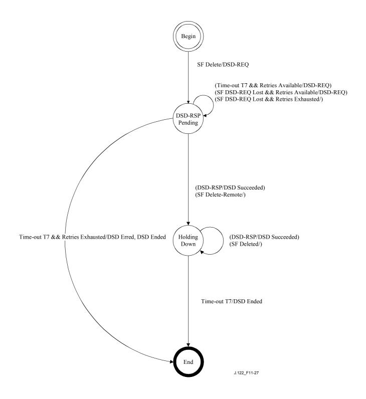
Figure 11-27/J.122 – DSD – Locally initiated Transaction State Transition Diagram
