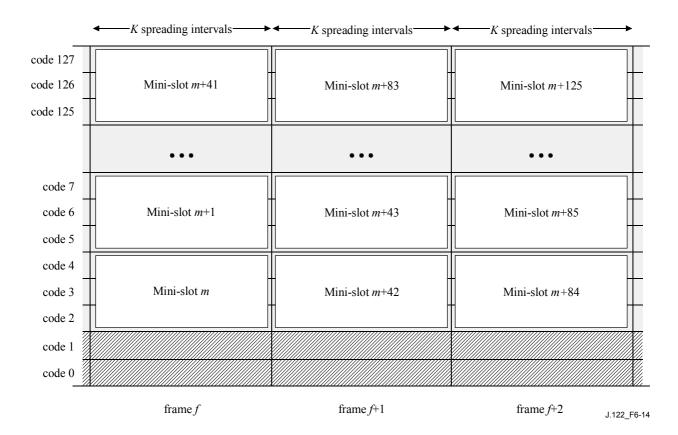
Figure 6-14/J.122 – Mini-slot mapping with three codes per mini-slot, 126 active codes
