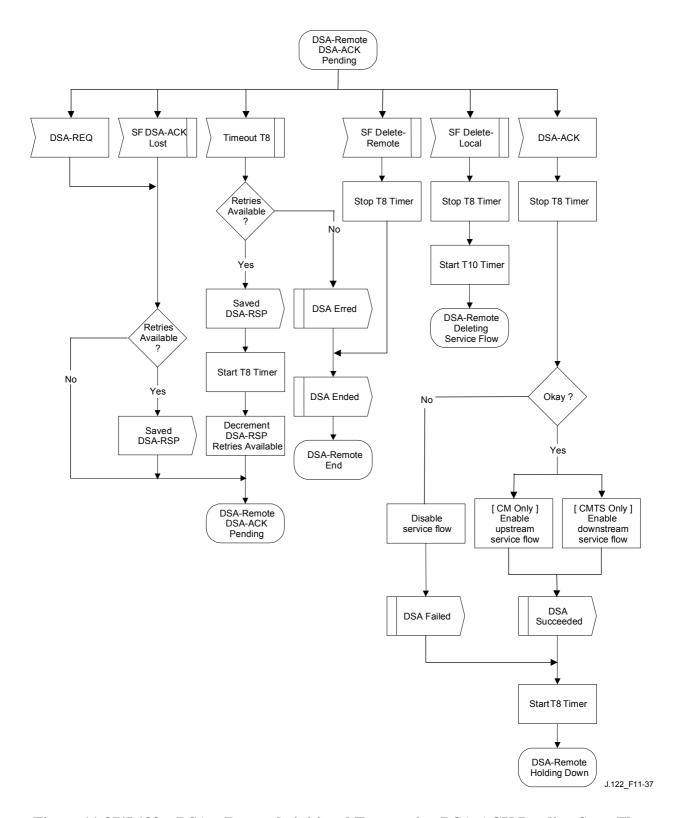
Figure 11-37/J.122 – DSA – Remotely initiated Transaction DSA-ACK Pending State Flow Diagram
