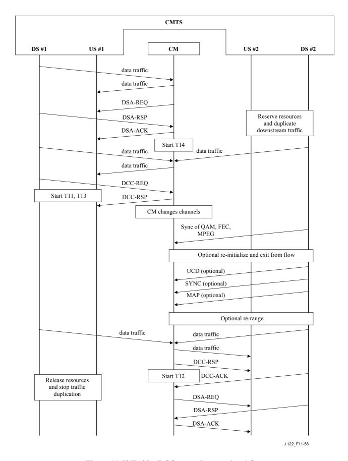
Figure 11-58/J.122 – DCC example operational flow
