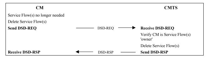
Figure 11-51/J.122 – Dynamic Service Deletion initiated from CM
