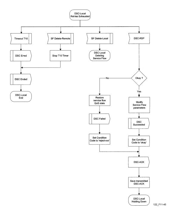
Figure 11-45/J.122 – DSC – Locally initiated Transaction Retries Exhausted State Flow Diagram
