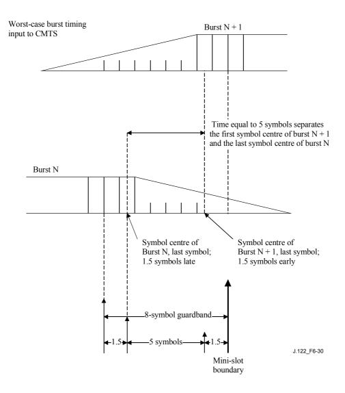
Figure 6-30/J.122 – Worst-case TDMA burst timing
