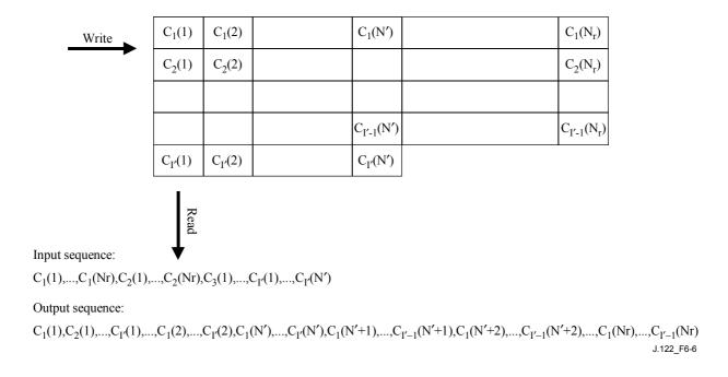
Figure 6-6/J.122 – Interleaver operation for last Interleaver block (with shortened last codeword)
