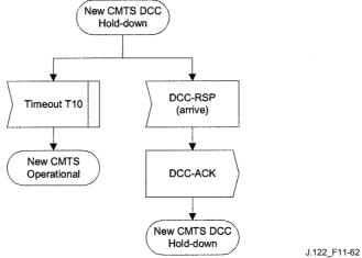
Figure 11-62/J.122 – Dynamically changing channels: CMTS view, Part 4
