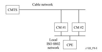
Figure 5-3/J.122 – Example condition for network loops
