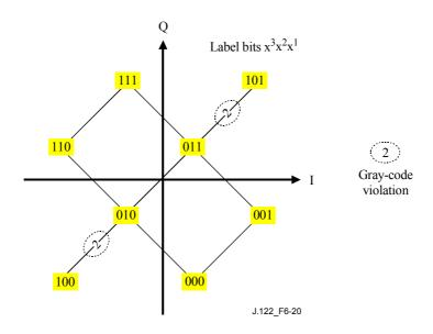
Figure 6-20/J.122 – 8QAM symbol mapping
