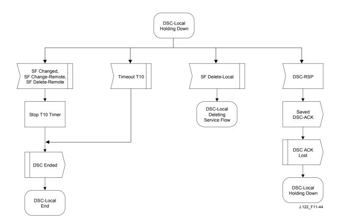
$Figure\ 11\text{-}44\text{/}J.122-DSC-Locally\ initiated\ Transaction\ Holding\ Down\ State\ Flow\ Diagram$
