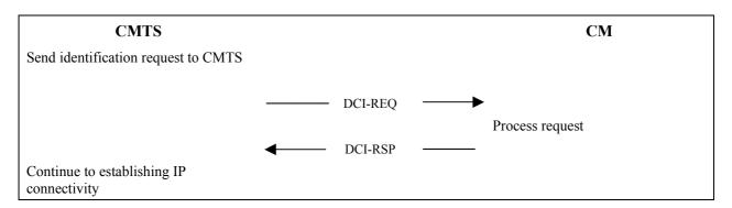
Figure 11-9/J.122 – Device Class identification
