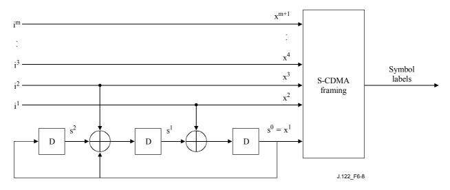
Figure 6-8/J.122 – Convolutional encoder
