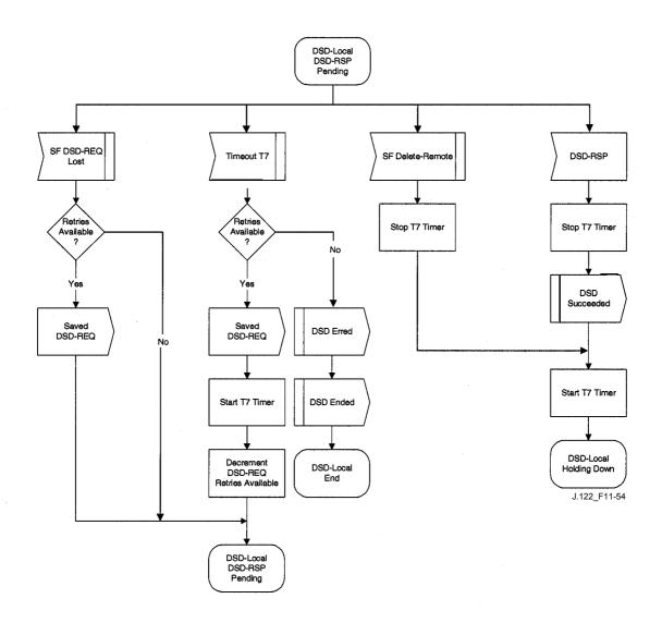
Figure 11-54/J.122 – DSD – Locally initiated Transaction DSD-RSP Pending State Flow Diagram
