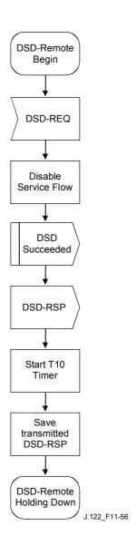
Figure 11-56/J.122 – DSD – Remotely initiated Transaction Begin State Flow Diagram
