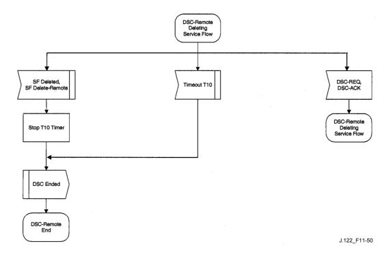
Figure 11-50/J.122 – DSC – Remotely initiated Transaction Deleting Service Flow State Flow Diagram
