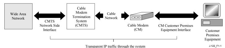
Figure 1-1/J.122 – Transparent IP traffic through the Data-Over-Cable system
