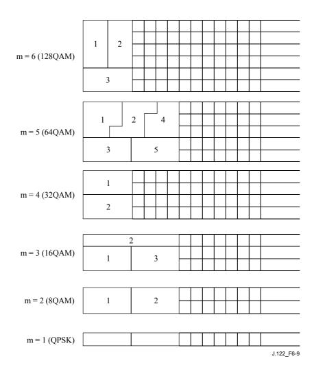
Figure 6-9/J.122 – Repetitive patterns of byte mapping to symbol map bits for TCM
