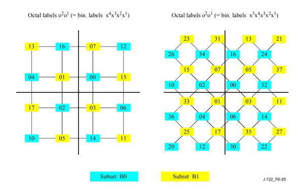
Figure 6-25/J.122 – 16QAM and 32QAM TCM symbol mapping
