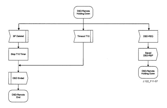
Figure 11-57/J.122 – DSD – Remotely initiated Transaction Holding Down State Flow Diagram
