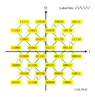
Figure 6-22/J.122 - 32QAM symbol mapping
