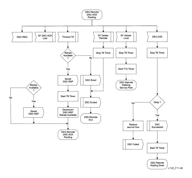
Figure 11-48/J.122 – DSC – Remotely initiated Transaction DSC-ACK Pending State Flow Diagram
