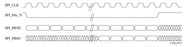
Figure H.7/J.122 – SPI Bus transaction
