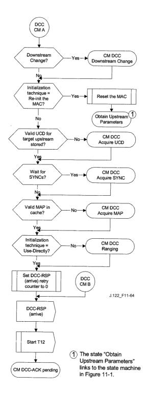
Figure 11-64/J.122 – Dynamically changing channels: CM view, Part 2
