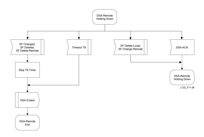
Figure 11-38/J.122 – DSA – Remotely initiated Transaction Holding Down State Flow Diagram
