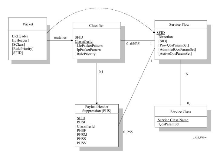
Figure 10-4/J.122 – Theory of Operation Object Model
