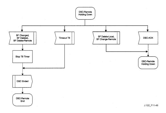
Figure 11-49/J.122 – DSC – Remotely initiated Transaction Holding Down State Flow Diagram
