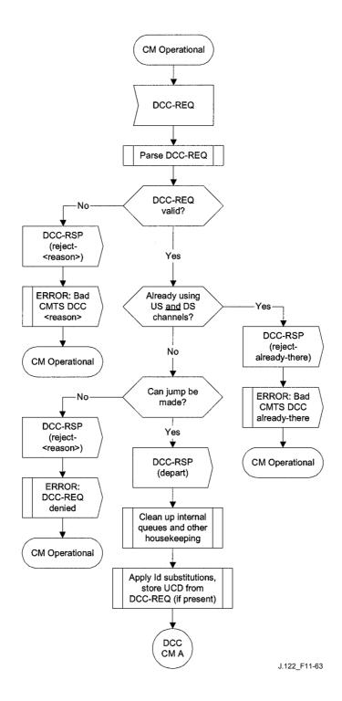
Figure 11-63/J.122 – Dynamically changing channels: CM view, Part 1
