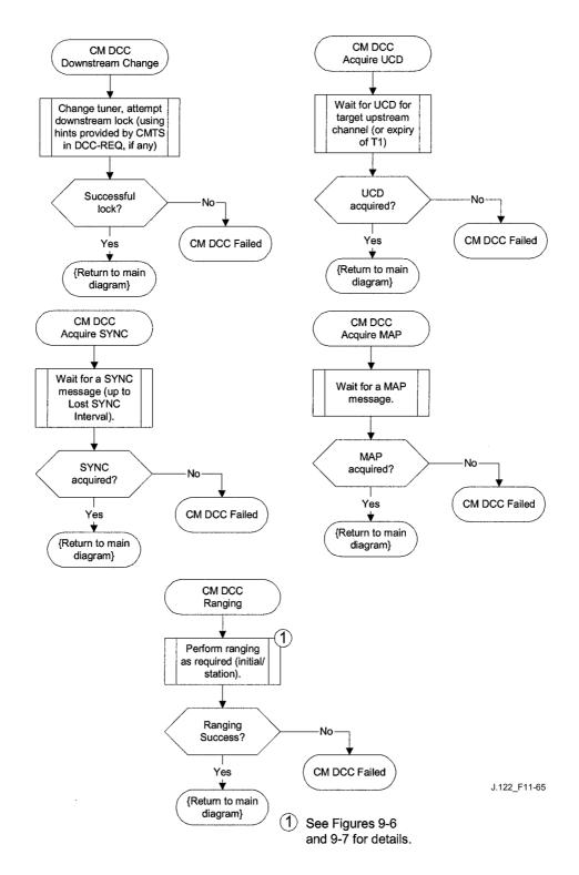
Figure 11-65/J.122 – Dynamically changing channels: CM view, Part 3
