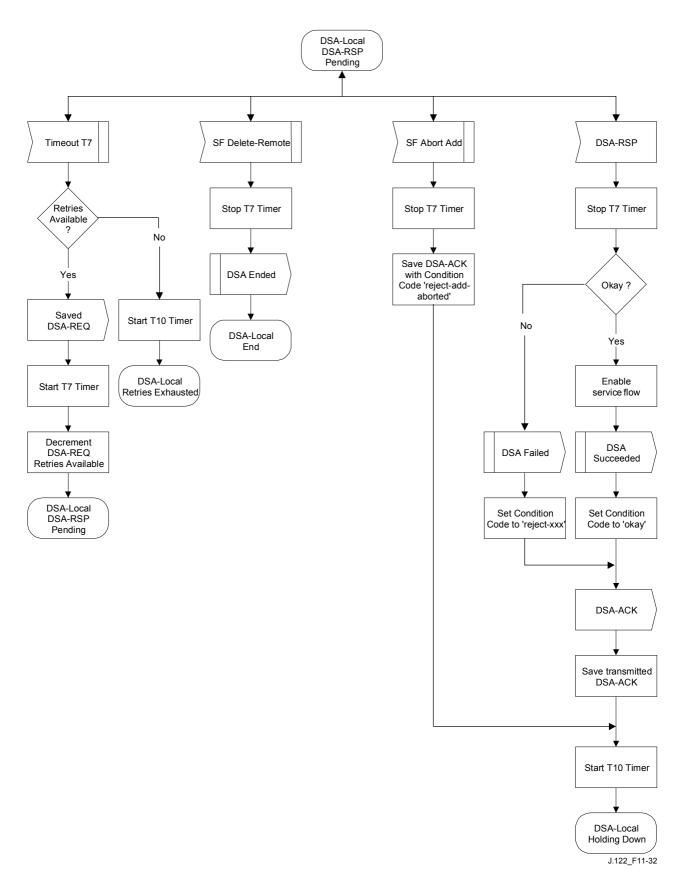
Figure 11-32/J.122 – DSA – Locally initiated Transaction DSA-RSP Pending State Flow Diagram
