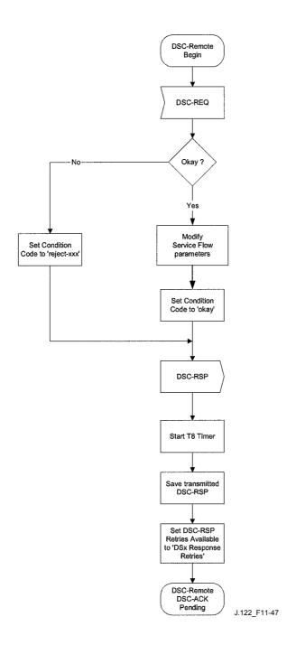
Figure 11-47/J.122 – DSC – Remotely initiated Transaction Begin State Flow Diagram
