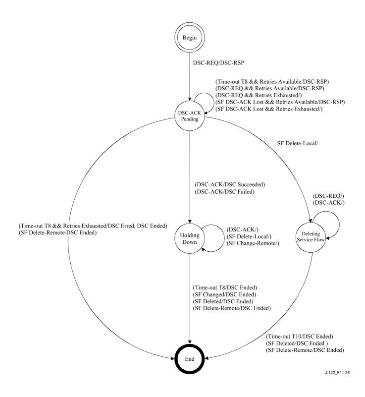
Figure 11-26/J.122 - DSC - Remotely initiated Transaction State Transition Diagram
