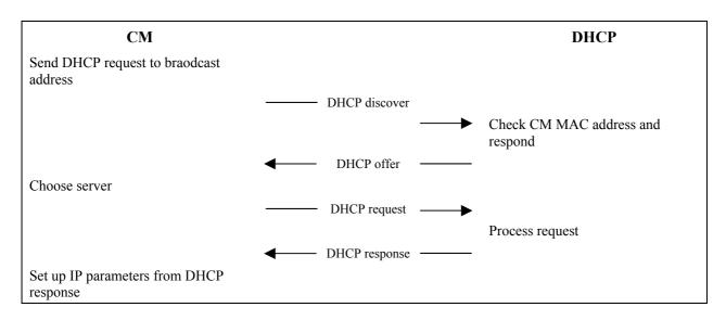
Figure 11-10/J.122 – Establishing IP connectivity
