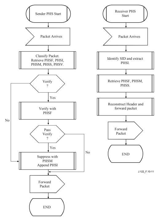
Figure 10-11/J.122 – Payload Header Suppression operation
