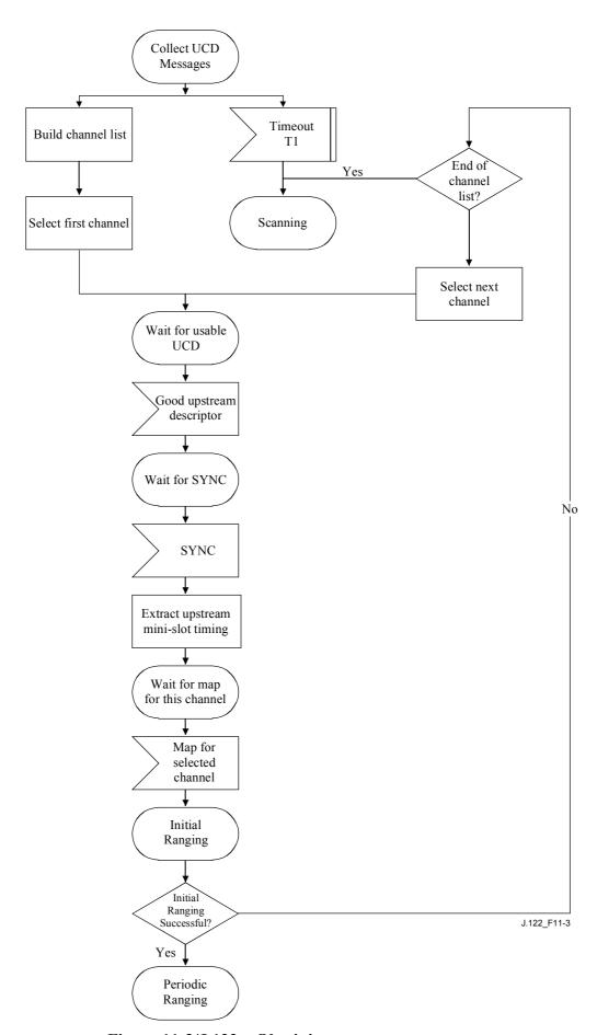
Figure 11-3/J.122 – Obtaining upstream parameters
