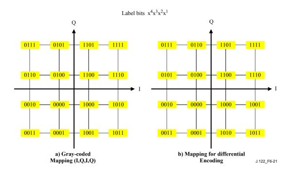
Figure 6-21/J.122 – 16QAM symbol mapping
