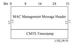
Figure 8-15/J.122 – Format of Packet PDU following the Timing Header
