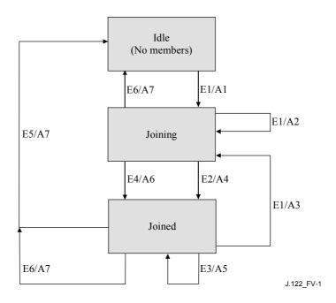
Figure V.1/J.122 – IGMP support – CM passive mode
