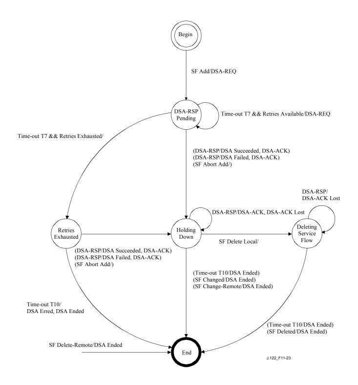
Figure 11-23/J.122 - DSA - Locally initiated Transaction State Transition Diagram
