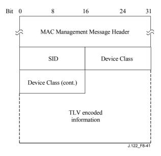
Figure 8-41/J.122 – Device Class Identification Request
