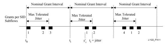
Figure VI.1/J.122 – Example jitter with multiple grants per SID
