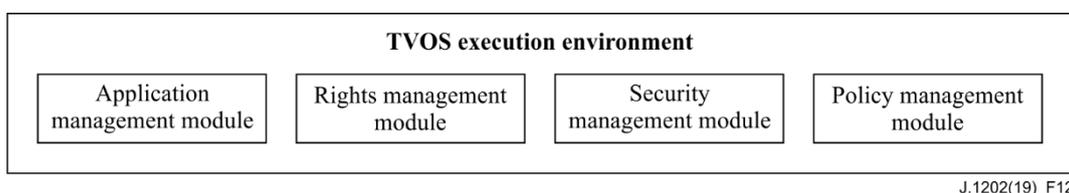
**Figure 12 – Architecture and implementation of a TVOS execution environment**
