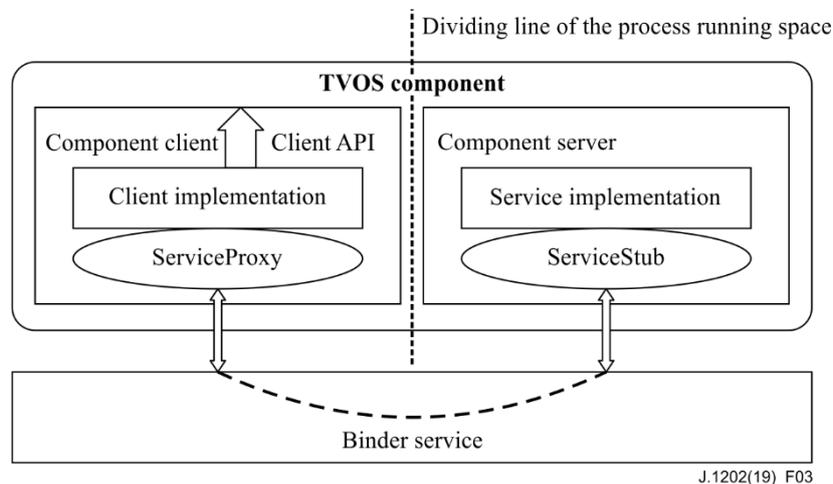
**Figure 3 – Component model diagram**
