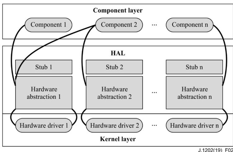
**Figure 2 – Principle of the stub hardware abstraction model of the TVOS HAL**
