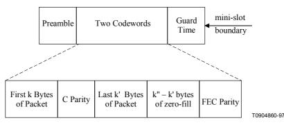
Figure B.4-7/J.116 – Example frame structures with flexible burst length mode
