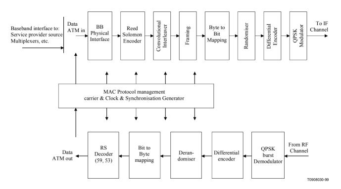
Figure A.5/J.116 - Conceptual block diagram for the OOB head-end transceiver
