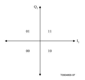
Figure B.4-1/J.116 – QPSK symbol mapping
