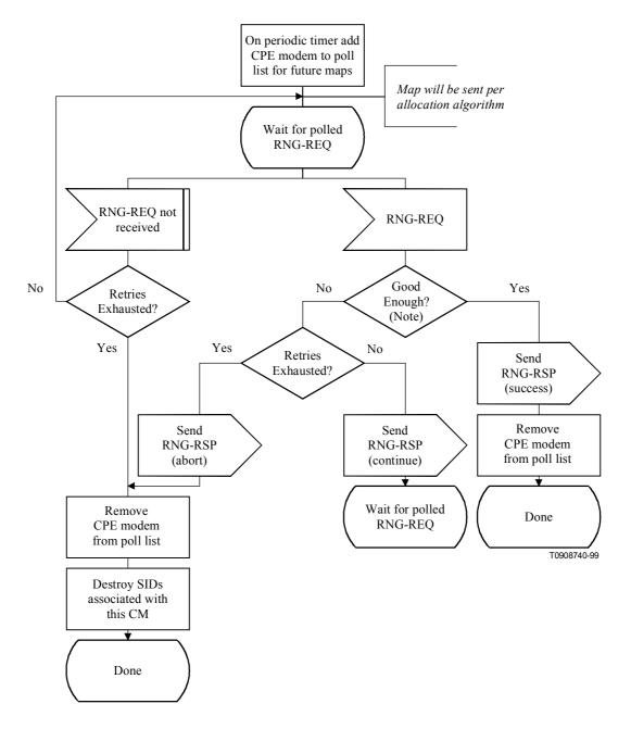
NOTE - Means Ranging Request is within the tolerance limits of the BTS modem for power and transmit equalization (if supported).
