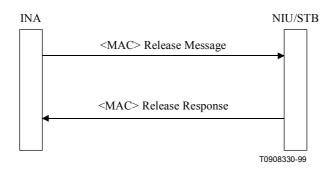
Figure A.31/J.116 – Connection release signalling
