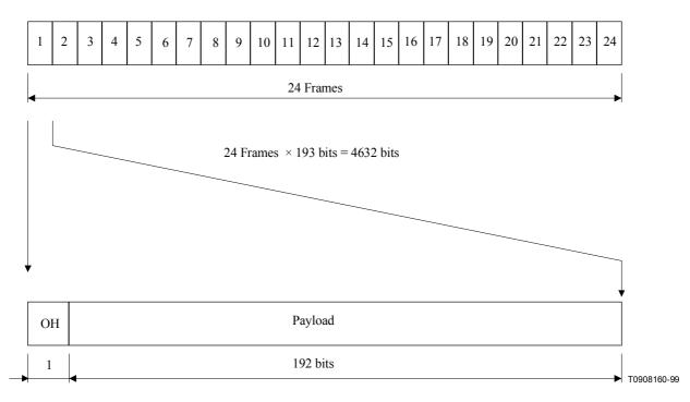
Figure A.15/J.116 – SL-ESF frame structure
