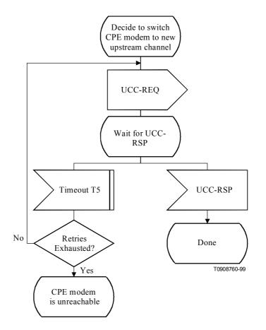
Figure B.7-14/J.116 – Changing upstream channels: BWA BTS Modem View
