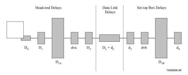
Figure A.22/J.116 – System model for timing analysis
