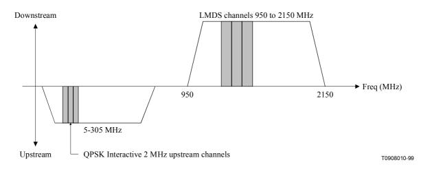
Figure A.3b/J.116 – Preferred IF frequency ranges for LMDS interactive systems (IB)
