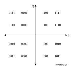
Figure B.4-2/J.116 – 16-QAM Gray-Coded Symbol Mapping
