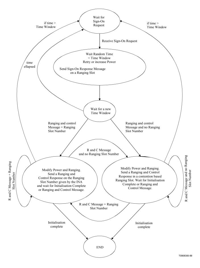
Figure A.28/J.116 – State diagram for ranging and calibration
