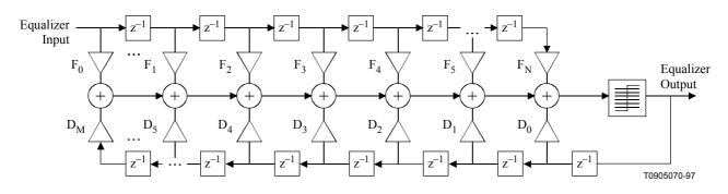
Figure B.6-23/J.116 – BWA BTS Modem Demodulator Equaliser Tap Location Definition
