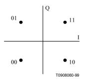
Figure A.8/J.116 – Mapping for the QPSK constellation (downstream OOB)
