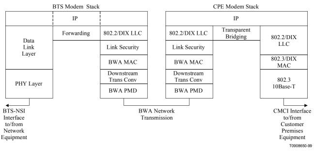
Figure B.3-2/J.116 – Data forwarding through the BWA CPE Modem and the BWA BTS Modem
