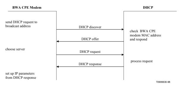
Figure B.7-9/J.116 – Establishing IP connectivity
