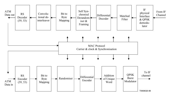
Figure A.4/J.116 – Conceptual block diagram for the NIU OOB transceiver
