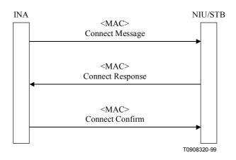
Figure A.30/J.116 – Connection signalling
