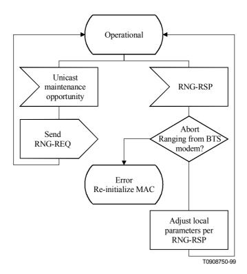
Figure B.7-13/J.116 – Periodic Ranging – BWA CPE Modem View
