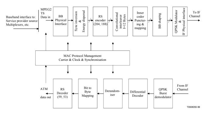
Figure A.7/J.116 - Conceptual block diagram for the IB head-end transceiver
