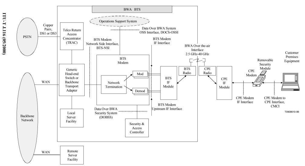
Figure B.1-2/J.116 – Data-over-BWA reference architecture
