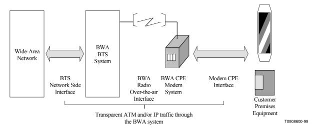
Figure B.1-1/J.116 – Transparent ATM and/or IP traffic through the BWA system
