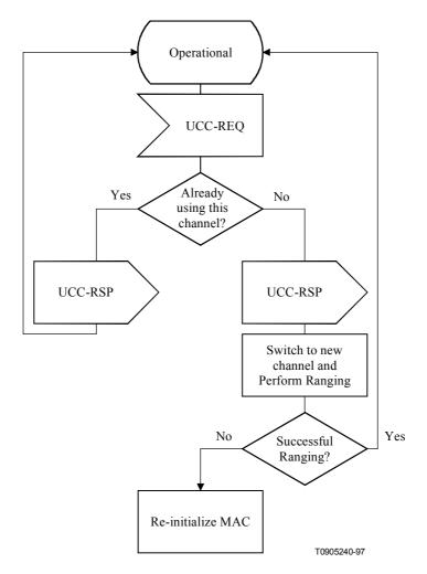
Figure B.7-15/J.116 – Changing upstream channels: BWA CPE Modem View
