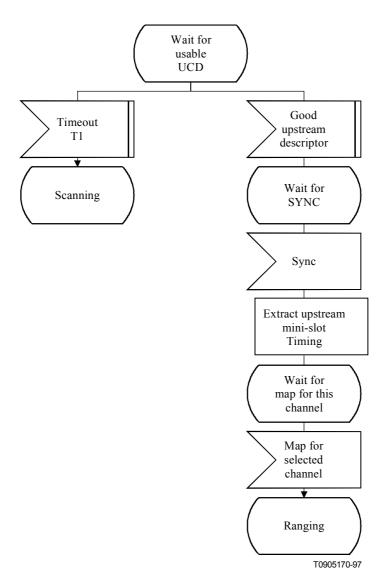
Figure B.7-3/J.116 – Obtaining Upstream Parameters
