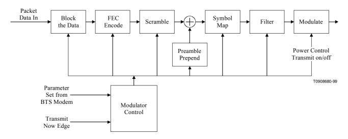
Figure B.4-8/J.116 – Signal processing sequence
