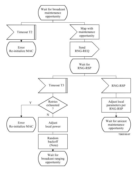
NOTE – Timeout T3 may occur because the RNG-REQs from multiple modems collided. To avoid these modems repeating the loop in lockstep, a random backoff is required. This is a backoff over the ranging window specified in the UCD.
