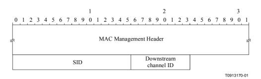
Figure B.6-20/J.116 – Packet PDU following the Timing Header
