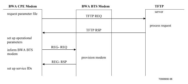
Figure B.7-11/J.116 – Transferring operational parameters and registration
