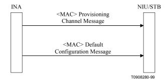
Figure A.26/J.116 – Initialisation and provisioning signalling
