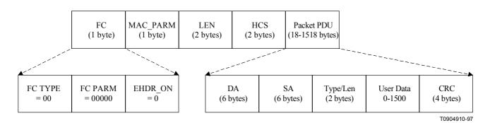
Figure B.6-4/J.116 – Ethernet/802.3 packet PDU format
