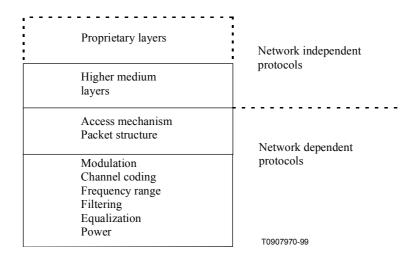
Figure A.1/J.116 – Layer structure for generic system reference model
