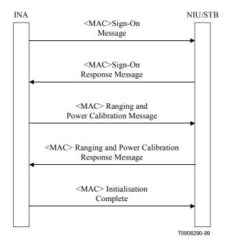
Figure A.27/J.116 – Ranging and calibration signalling
