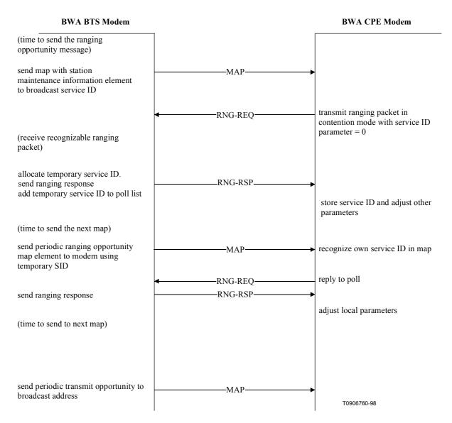
Figure B.7-5/J.116 – Ranging and Automatic Adjustments Procedure
