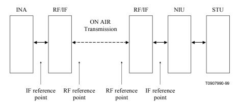
Figure A.2b/J.116 – Position of IF and RF reference points in the particular case of LMDS networks
