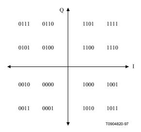
Figure B.4-3/J.116 – 16-QAM Differential-Coded Symbol Mapping
