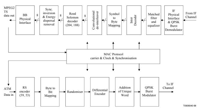
Figure A.6/J.116 - Conceptual block diagram for the IB NIU transceiver
