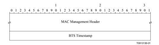
Figure B.6-14/J.116 – Format of packet PDU following the timing header
