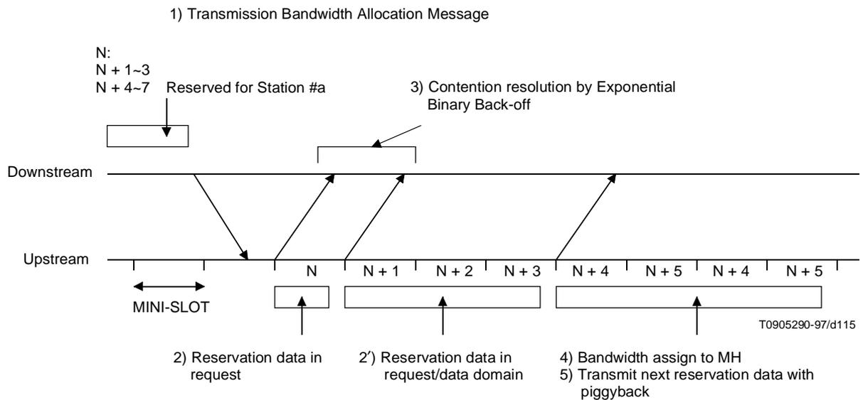
Figure C.6-2/J.112 – Bandwidth assignment by mini-slot and message
