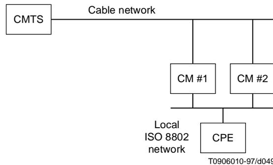
**Figure B.3-3/J.112 – Example condition for network loops**
