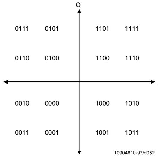
Figure B.4-2/J.112 – 16 QAM Gray-coded symbol mapping
