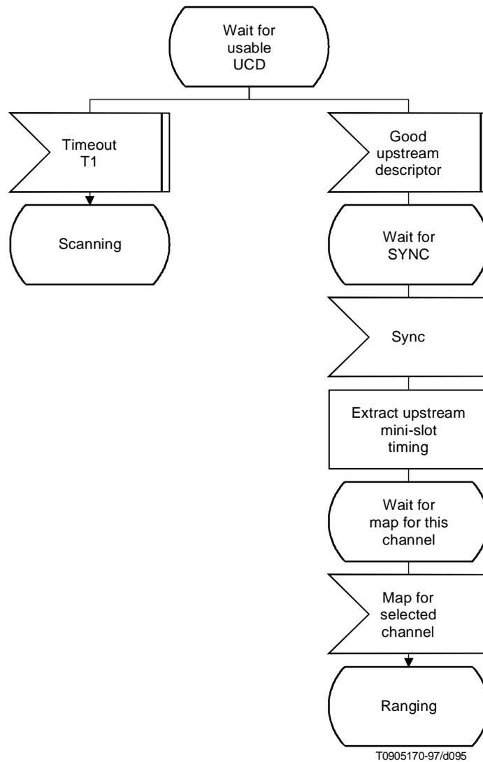
**Figure B.7-3/J.112 – Obtaining upstream parameters**
