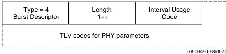
**Figure B.6-16/J.112 – Top-level encoding for a Burst Descriptor**
