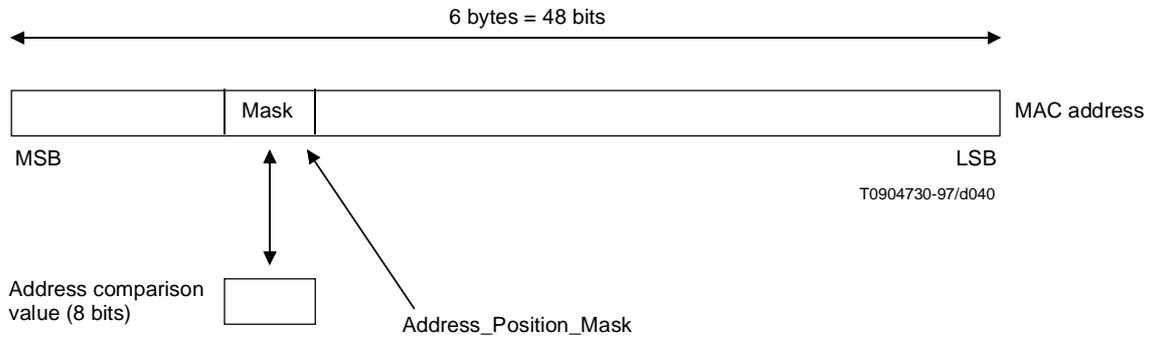
Figure A.31/J.112 – Position of Mask in MAC address
