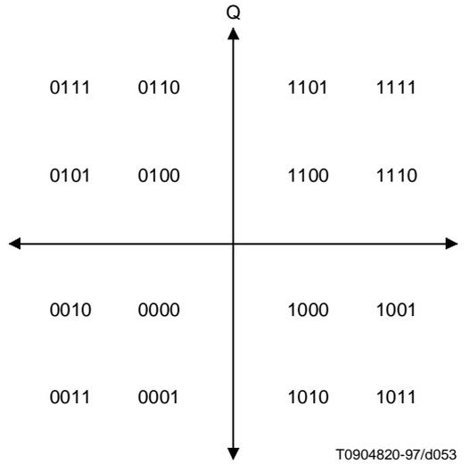
**Figure B.4-3/J.112 – 16 QAM differential-coded symbol mapping**
