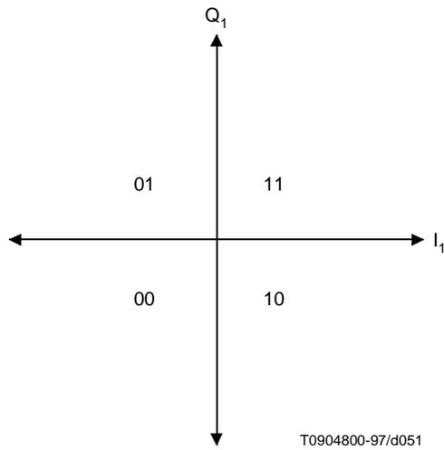
Figure B.4-1/J.112 – QPSK symbol mapping
