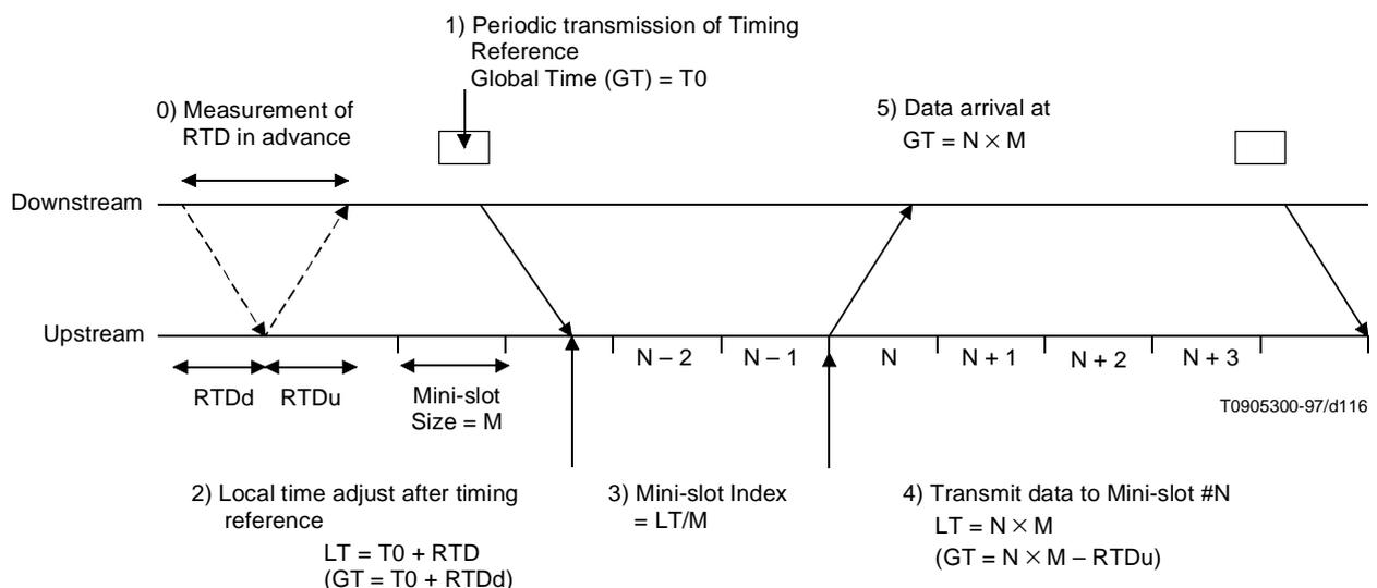
Figure C.6-3/J.112 – Global timing synchronization
