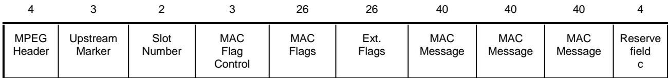
Figure A.20/J.112 – Frame structure (MPEG-2 TS format)
