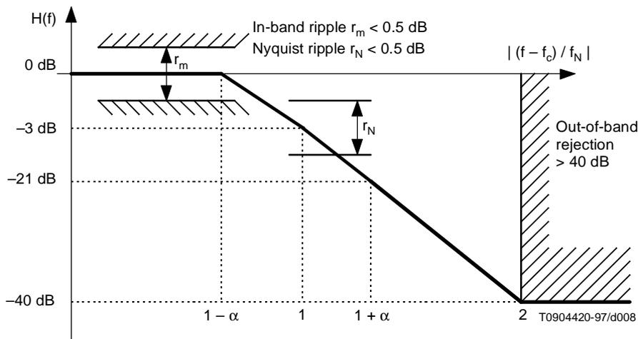
**Figure A.9/J.112 – QPSK downstream transmitter Power Spectrum**
