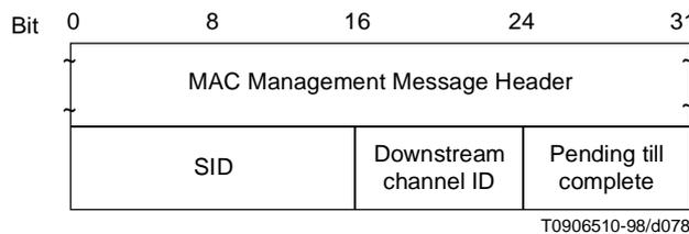
**Figure B.6-20/J.112 – Packet PDU following the Timing Header**
