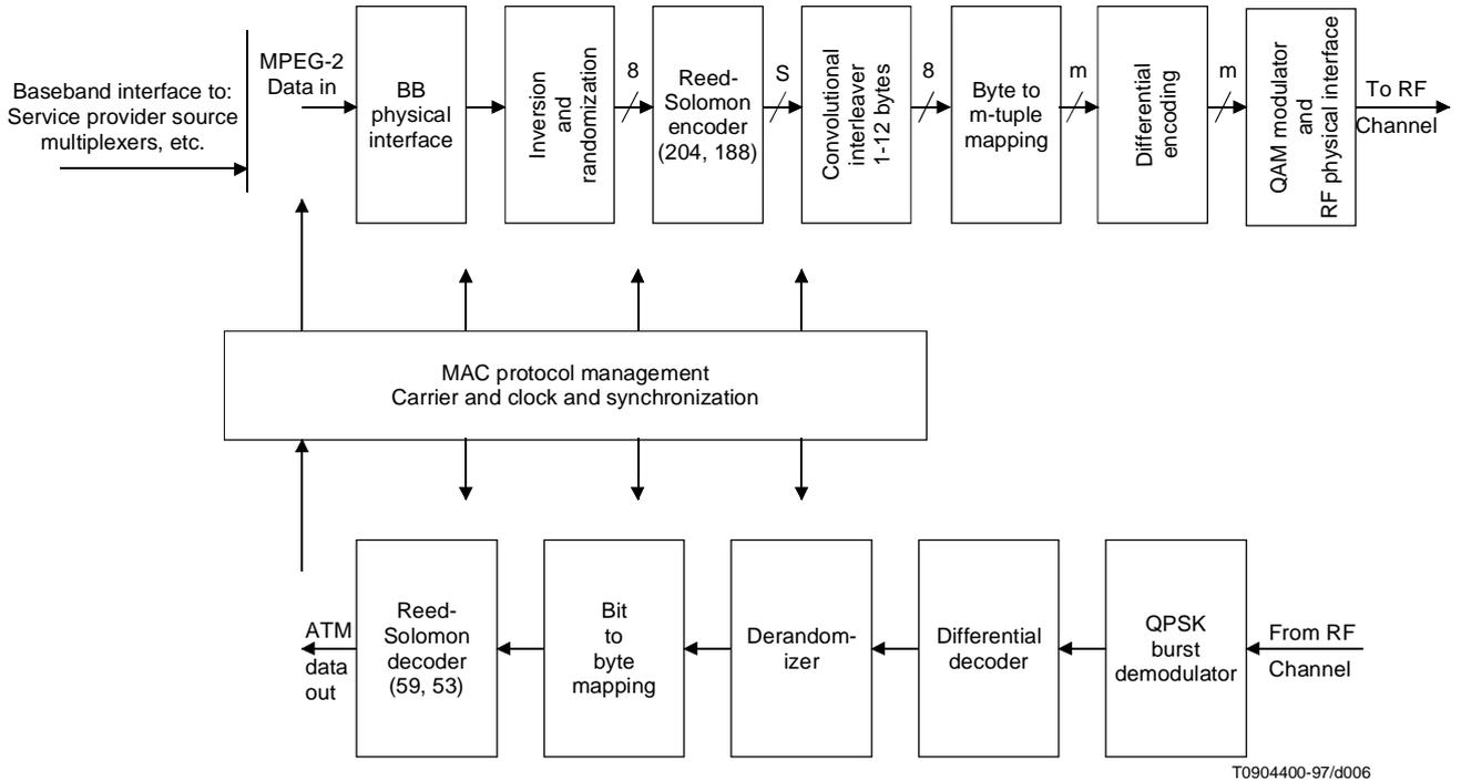
Figure A.7/J.112 – Conceptual block diagram for the IB head-end transceiver
