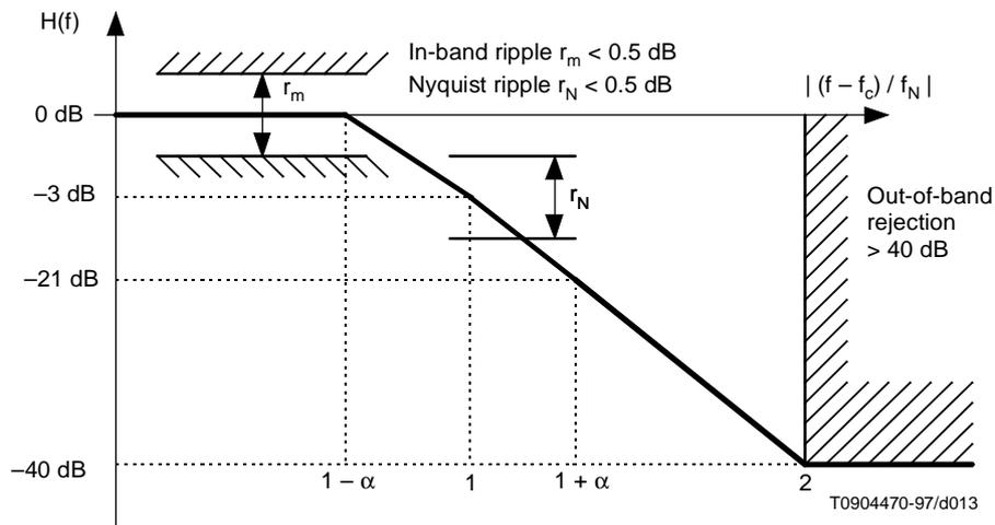
Figure A.14/J.112 – QPSK upstream transmitter Power Spectrum
