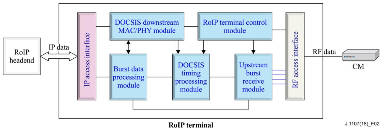
**Figure 2 – Architecture for radio over Internet protocol terminal**
