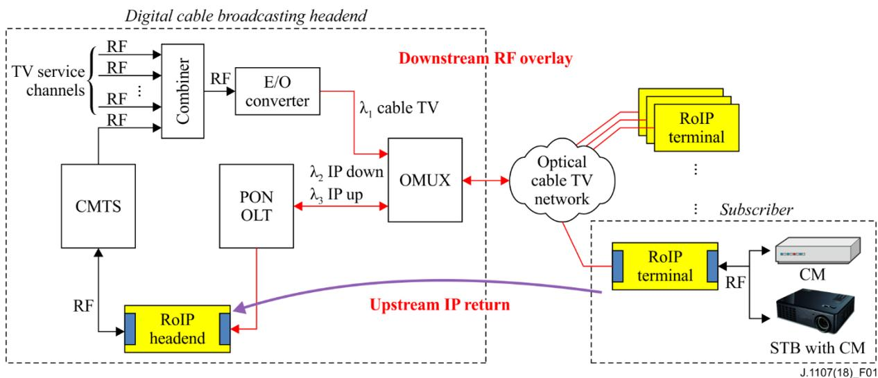
**Figure 1 – System architecture for radio over Internet protocol**
