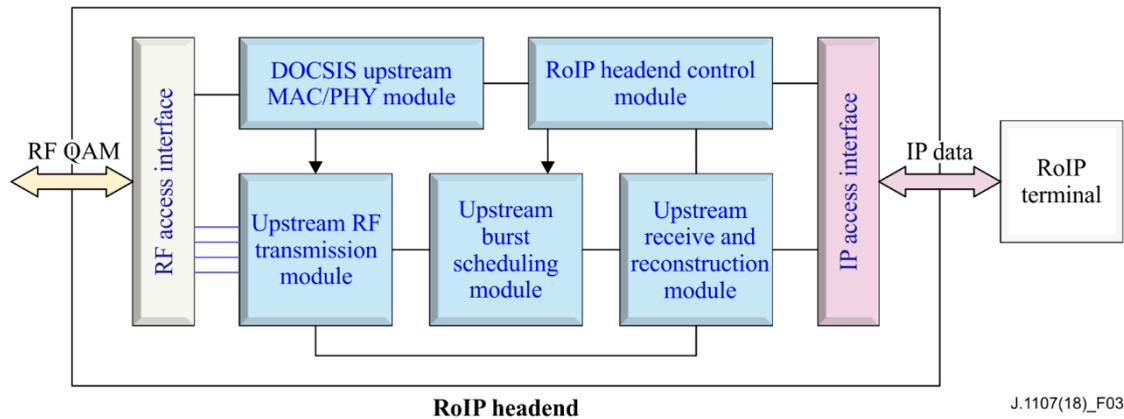
**Figure 3 – Architecture for radio over Internet protocol headend**
