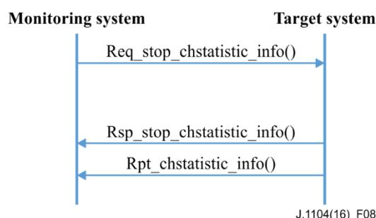
**Figure 8 – Message communication procedure to stop collecting channel statistics information of performance monitoring**
