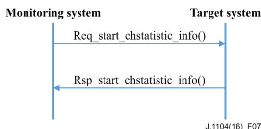
**Figure 7 – Message communication procedure to start collecting channel statistics information of performance monitoring**
