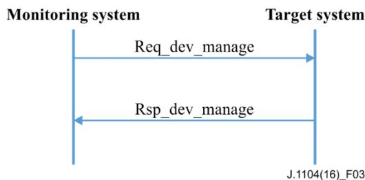
**Figure 3 – Message communication procedure for device management**
