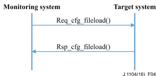
**Figure 4 – Message communication procedure for configuration file load**
