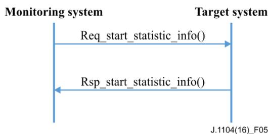
**Figure 5 – Message communication procedure to start collecting statistics information of performance monitoring**
