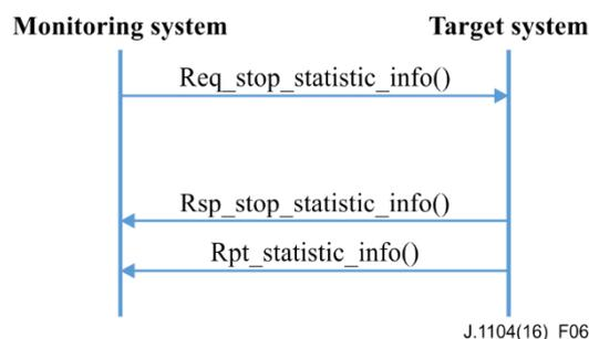
**Figure 6 – Message communication procedure to stop collecting statistics information of performance monitoring**
