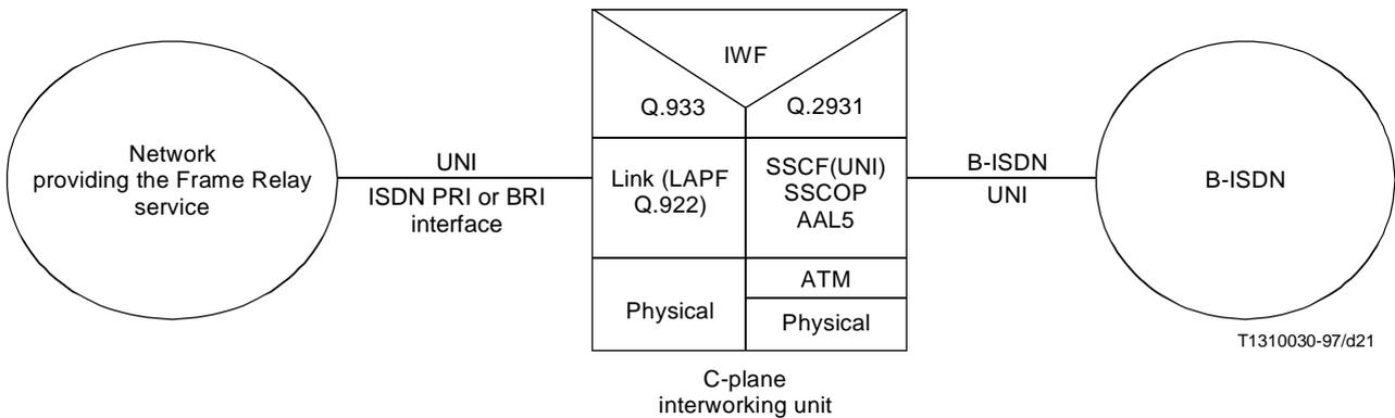
**Figure 19/I.555 – Service interworking in the C-plane between a network providing the Frame Relay service and B-ISDN**
