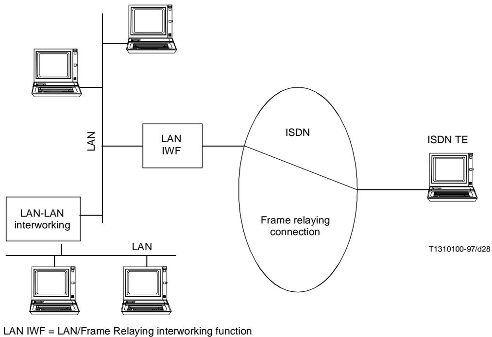
**Figure I.2/I.555 – Interconnecting LANs to an ISDN TE**
