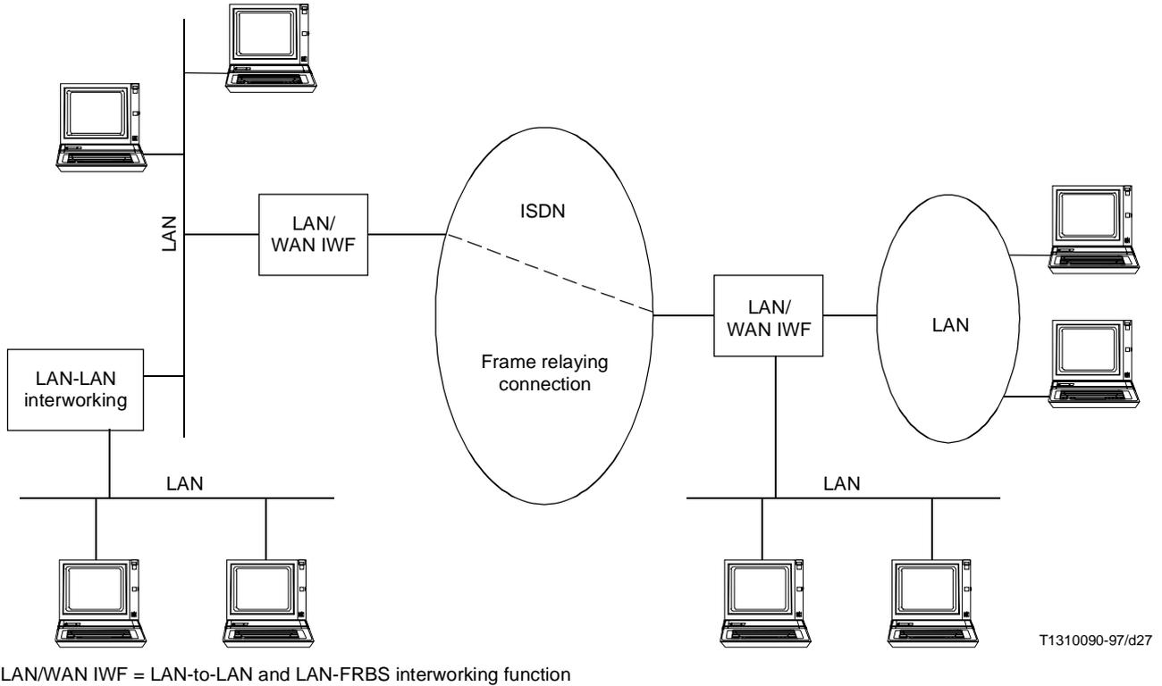
**Figure I.1/I.555 – LAN-LAN interconnection via ISDN Frame Relaying**
