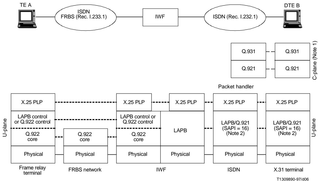
NOTE 1 – C-plane procedures are used for outgoing calls on the B-channel (i.e. from DTE B) to establish an access connection to the Packet Handler (PH) in the ISDN and for incoming calls (i.e. to DTE B) when notification of an X.25 incoming call is required.
