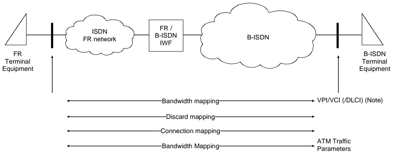
NOTE – The DLCI parameter identifies FR connections at the FR interface. The VPI/VCI parameter identifies the ATM connection at the B-ISDN interface. The connection identifiers only have local significance, and accordingly there is no requirement to map between the FR DLCI and the ATM VPI/VCI parameters. The DLCI is only significant on the B-ISDN side in the case of N to 1 mapping.
