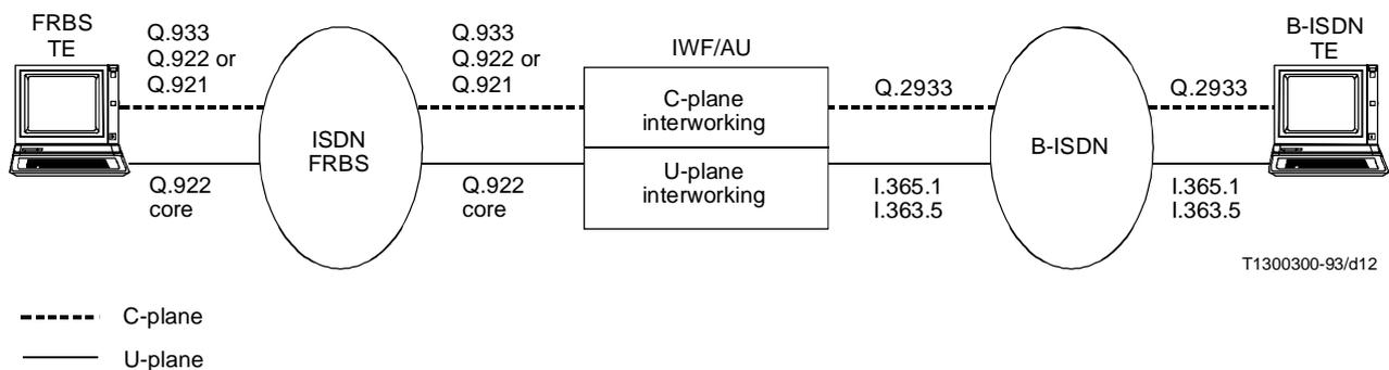
NOTE 1 – Q.2933 is only used for network interworking and in the case of service interworking I.365.1 is not used but Q.2931 is used.
