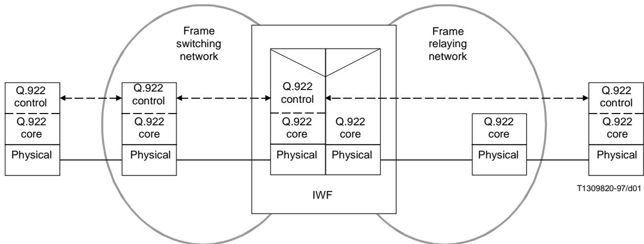
**Figure 1/I.555 – Interworking between Frame Relaying and Frame Switching:
