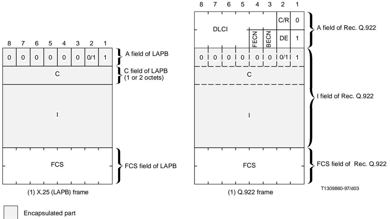
**Figure 3a/I.555 – Encapsulation of LAPB address, control and I-fields in Q.922 core**
