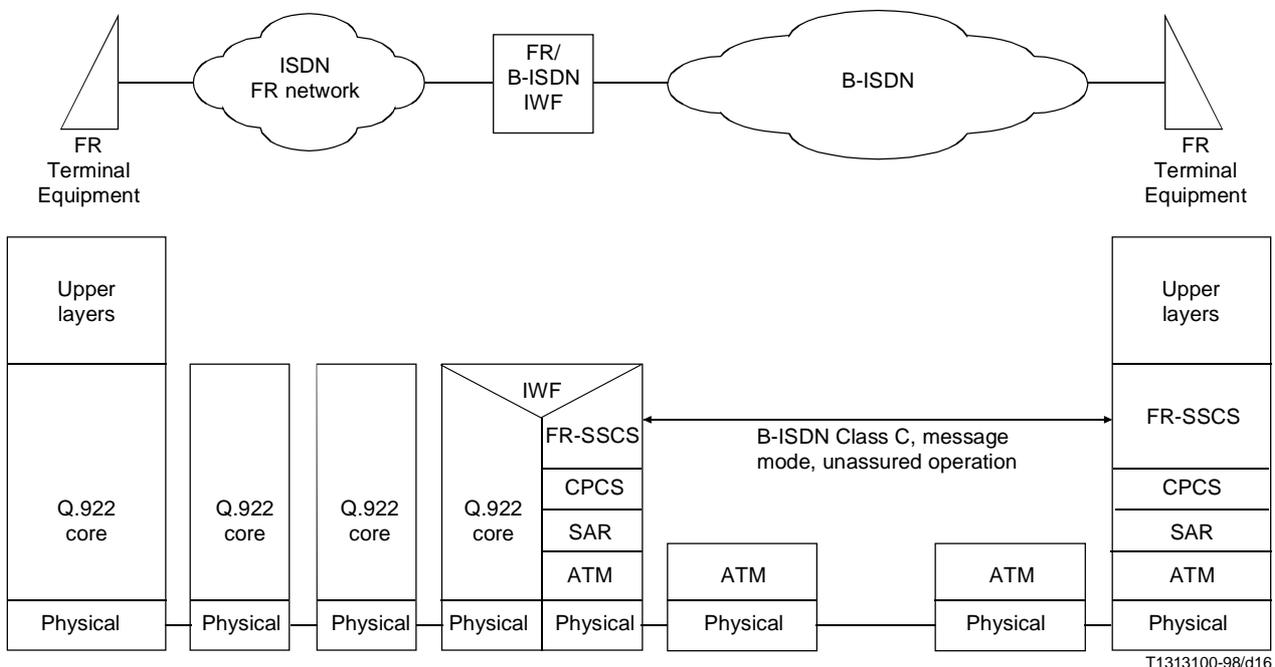
Figure 14/I.555 – Frame Relay/B-ISDN network interworking (Scenario 2)
