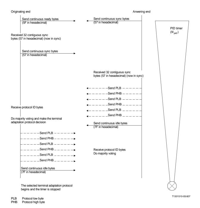
NOTE – If the PID phase fails for whatever reason (e.g. no PID, error in PID) and the timer expires, the TA device can default to a preferred TA protocol as shown in the flow diagram of Figure I.1.
