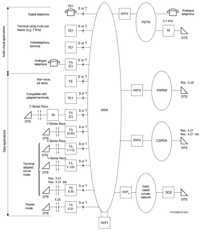
IWF Interworking function (may include: physical requirements, signalling requirements, terminal adaptation modulation,etc.) M Modem
