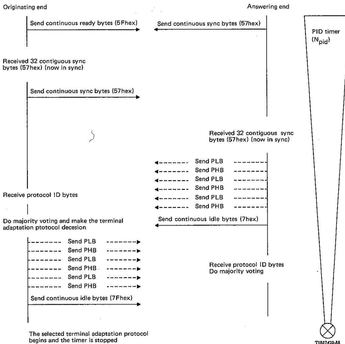
Note – If the PID phase fails for whatever reason (e.g. no PID, error in PID) and the timer expires, the TA device can default to a preferred TA protocol as shown in the flow diagram of Figure I-1/I.515.
