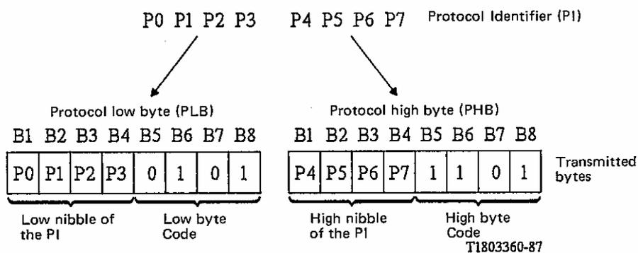
*Note 1* — P0 and P4 are the first bits transmitted and received in their respective bytes.
