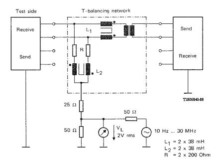
Note — The inherent longitudinal conversion loss of the T-balancing network should be 20 dB better than required at the interface under test (see Recommendation 0.121).
