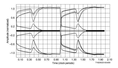
$\label{eq:FIGURE 8/I.430} Waveform for test configuration iii) a) - Short passive bus \\ with one TE near to NT, and seven TEs at the far end (C = 120 nF/km)$
