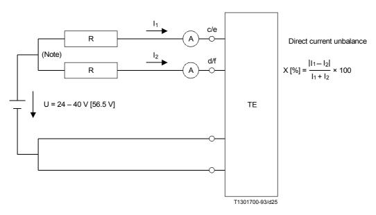
NOTE-The resistors R (2 ohm) represent the TE cord equivalent. They should not be used if the TE has an attached cord.
