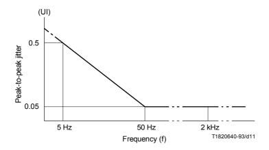
FIGURE 10/I.430 Lower limit of maximum tolerable jitter
