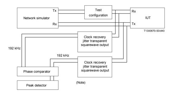
NOTE-For measurement purposes, an additional low-pass filter with a cut-off frequency higher than 96 kHz can be added.
