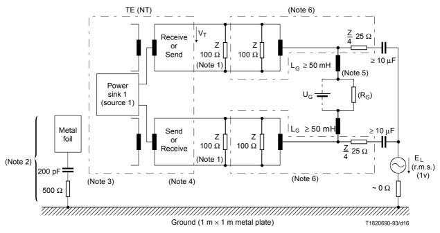
The longitudinal conversion loss: LCL = 20  $\log_{10} \frac{E_L}{V_L}$  dB.
