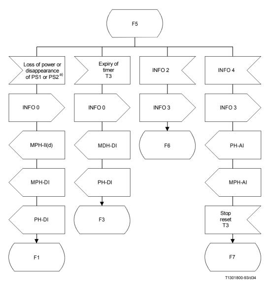
a) Whichever power source is used for determining the connection status.
