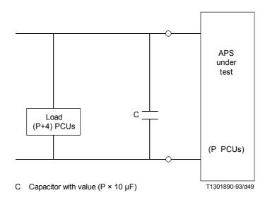
FIGURE I.11/I.430 **APS switch-on time measurement**
