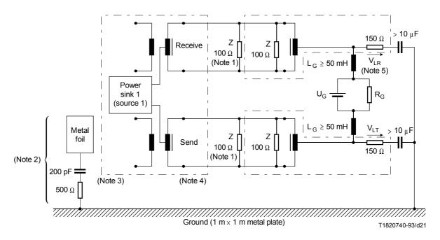
$V_{LT}$  and  $V_{LR} \le -24$  dBV peak.
