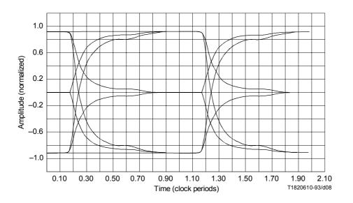
$FIGURE\ 7/I.430$  Waveform for test configuration ii) – Short passive bus with eight clustered TEs at the far end (C = 120 nF/km)
