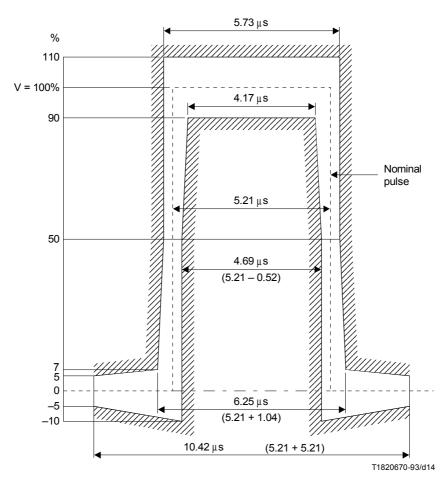
NOTE – For clarity of presentation, the above values are based on a pulse width of 5.21  $\mu\,s$ . See 8.1 for a precise specification of the bit rate.
