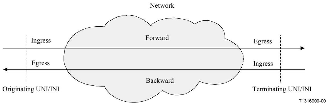
**Figure 1/I.377 – Illustration of the terminology originating/terminating UNI, forward/backward direction and ingress/egress sides of one network**
